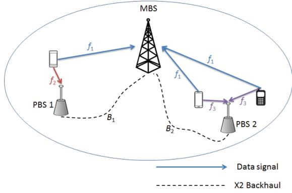
Fig. 1. A schematic diagram of the system model. The MBS operates on frequency band  $f_1$ . The two PBSs operate on frequency bands  $f_2$  and  $f_3$ , respectively. At the same time, each user can only be connected to one PBS.
