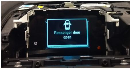
Fig. 7. The ECU obtained for bench testing operating in the lab vehicle. Despite ordering the correct used unit, it is a lower specification component (there is a small difference in the part numbers), it does functions correctly.
