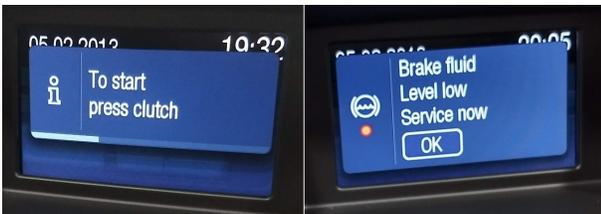
Fig. 12. CAN packets are injected into the lab vehicle's internal network to display false messages. The messages are incorrect because the vehicle requires the brake to be pressed to start, and the brake fluid level is correct.
