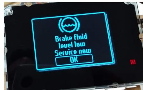
Fig. 10. The CAN data sent to the display ECU is manipulated to reverse engineer the ECU's functionality.
