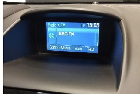
Fig. 5. The Display Interface (DI) ECU in the laboratory vehicle, a variety of messages are displayed in response to occupants operating the vehicle.
