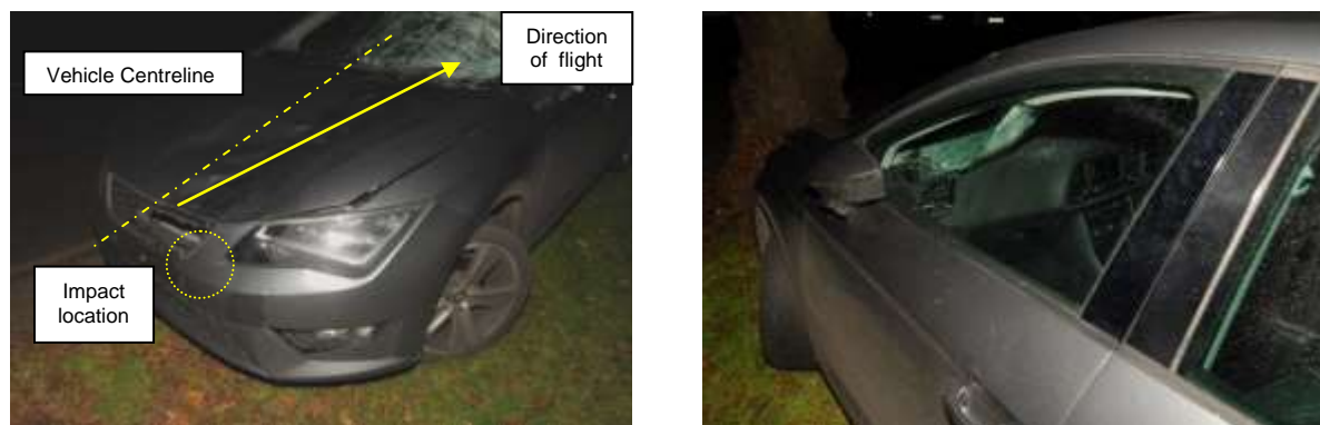
Fig.9: Vehicle damage at the accident scene
