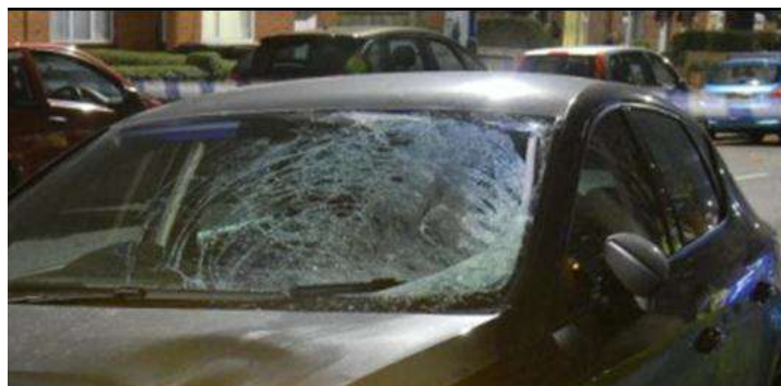
Fig.14: Focus on the windscreen area (impact area more outboard than CAE model)
