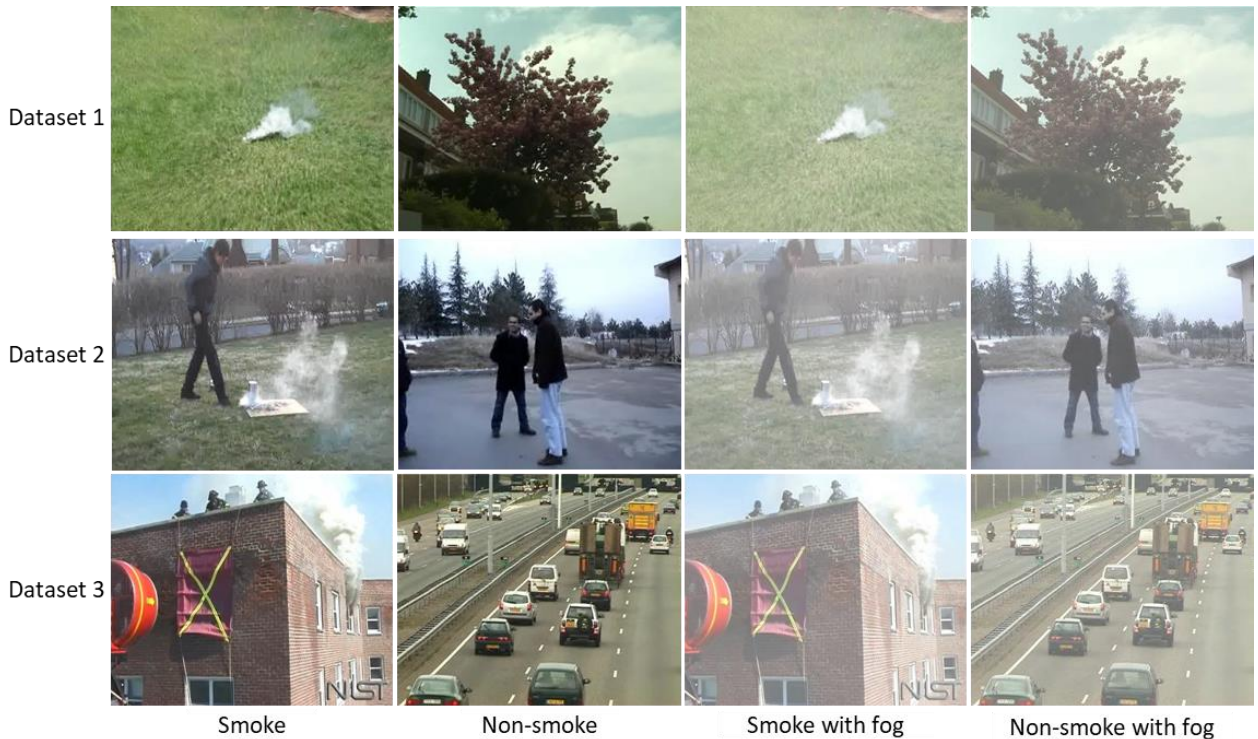
Fig. 5. Sample frames from the dataset belonging to our target four classes: “smoke”, “non-smoke”, “smoke with fog”, and “non-smoke with fog”.
