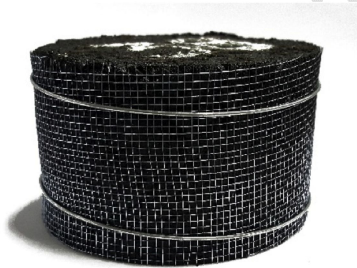
Fig. 5. Marshall lateral confinement before aging process.
