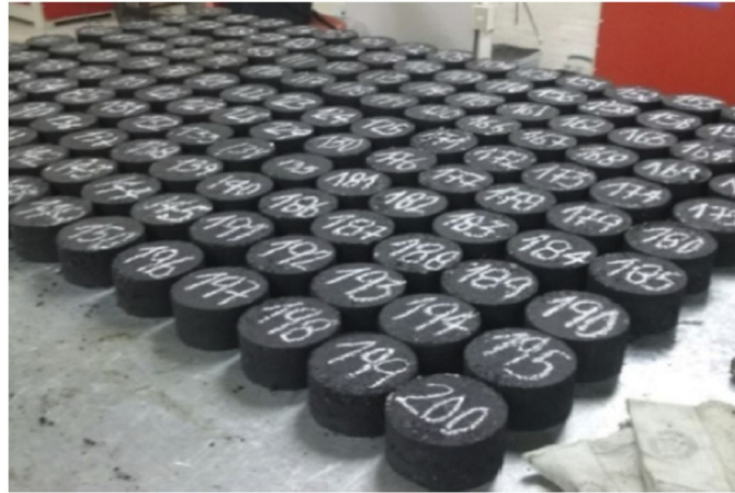
Fig. 4. Marshall samples fabricated in the laboratory.
