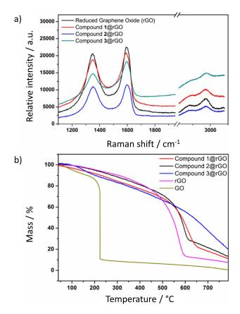
Figure 6. (a) Raman spectroscopy of solvothermally reduced rGO, 1@rGO, 2@rGO and 3@rGO at selected ranges of the spectra; (b) TGA-curves of GO, rGO and graphene@porphyrin composites.
