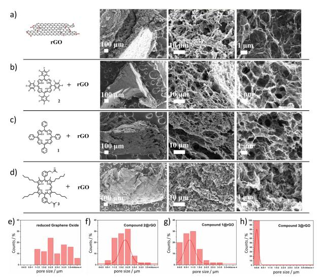
Figure 3. SEM images. Scale bar is 100  $\mu$ m, 10  $\mu$ m and 1  $\mu$ m respectively (a) rGO; (b) 2@rGO composite; (c) 1@rGO composite; (d) 3@rGO composite. Histogram of pore sizes (N = 100) as measured on SEM (e) rGO; (f) 2@rGO composite; (g) 1@rGO composite; (h) 3@rGO composite.
