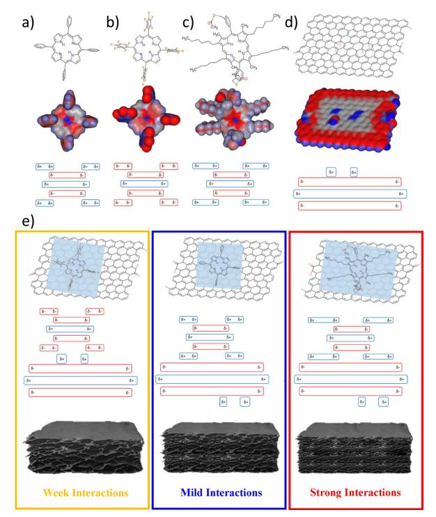
Figure 5. Semi-empirical level optimised geometries of: (a) compound 1; (b) compound 2; (c) compound 3 and (d) GO (red denotes areas of relatively high electron density, blue denotes electron deficient areas); (e) proposed stacking arrangements between compounds and GO and schemes show the formed 3D structures.
