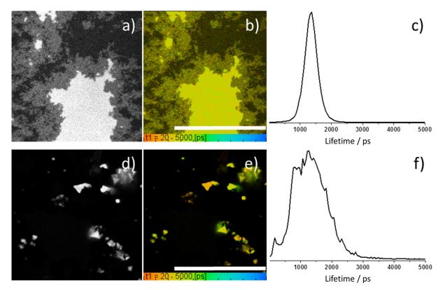
**Figure 8.** Single-photon FLIM of a thin film obtained by drop casting of a 1 mg/mL dispersion of nanohybrids in CHCl<sub>3</sub>: EtOH 1:1 onto borosilicate glass, (a) 1@rGO, intensity image,  $\lambda_{ex}$ =405 nm; (b) lifetime mapping of  $\tau_1$ ; (c) corresponding fluorescence lifetime  $\tau_1$  distribution curve; (d) 2@rGO, intensity image,  $\lambda_{ex}$ =405 nm; (e) lifetime mapping of  $\tau_1$ ; (f) corresponding fluorescence lifetime  $\tau_1$  distribution. Scale bars: 20 µm.
