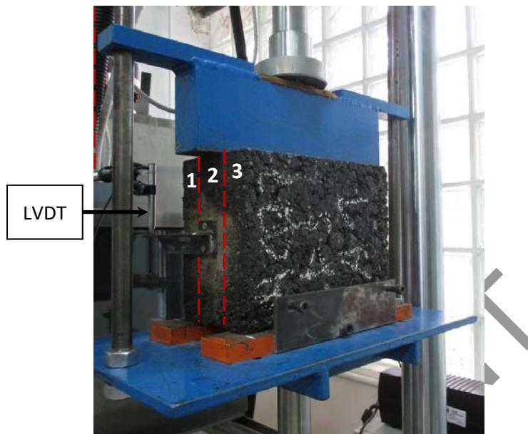
Figure 4. Shear fatigue adherence test
