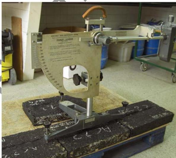
Figure 2. Evaluation of skid resistance
