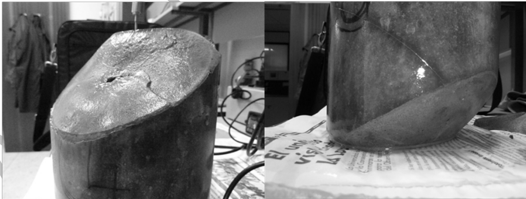
Fig. 11. Failure observed in the thermal conductivity probes of the Neat cement mortar.
