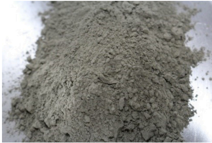
Fig. 1. Ash used was sifted through a sieve N°200 (0.08 mm).
