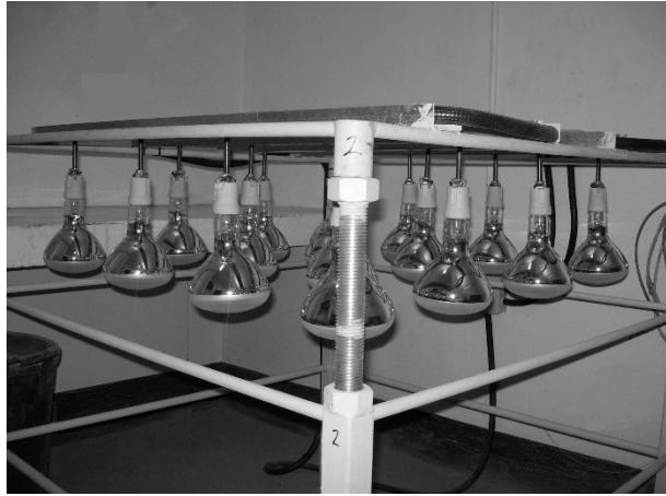
Fig. 3 - Solar simulator lamp used for the thermal (irradiation) tests of the asphalt samples.
