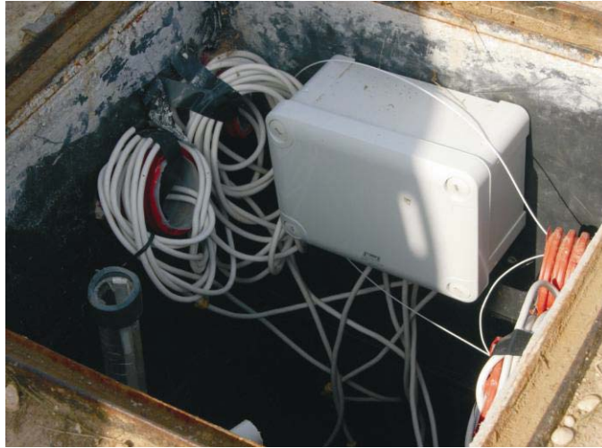
Figure 4. Register box with datalogger and temperature probes
