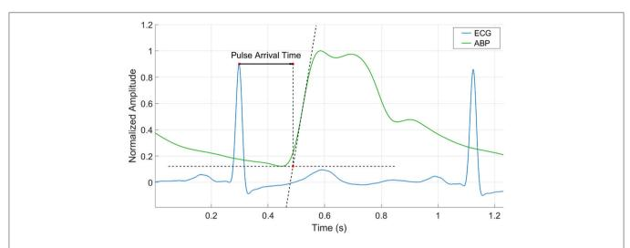
FIGURE 2 | Pulse Arrival Time calculation by the intersecting tangent method. The time is estimated from the r-peak of the ECG waveform to the intersection point of the tangent to the maximum gradient and tangent of the onset value in the ABP waveform.
