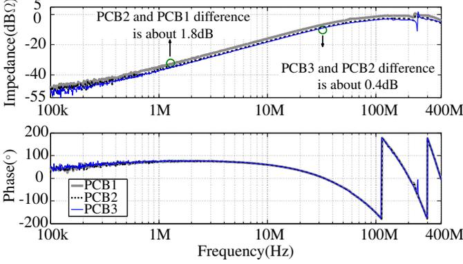
(b) CSP complex transfer impedance measurement results
