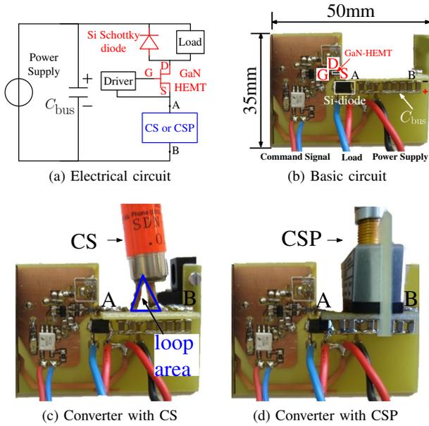
Fig. 6: GaN-HEMT buck converter with two current probes
