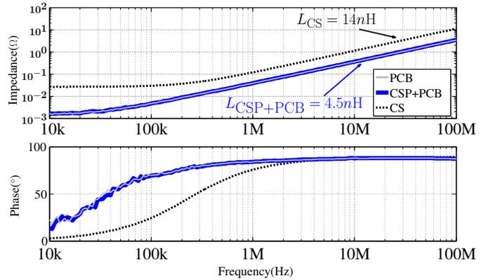
Fig. 8: CS and CSP insertion impedance measurement results
