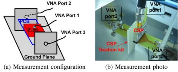
Fig. 2: CSP transfer impedance measurement configuration
