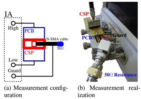
Fig. 7: CSP insertion impedance measurement configuration and its realization
