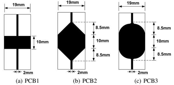
Fig. 3: Three PCB configurations to characterize CSP transfer impedance
