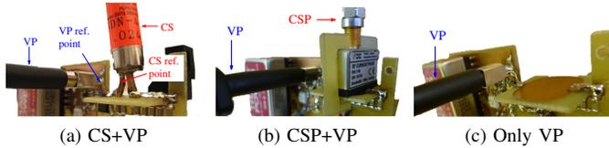
Fig. 13: GaN-HEMT  $V_{DS}$  switching voltage measurement
