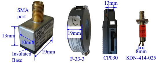
Fig. 1: Dimension of different current probes
