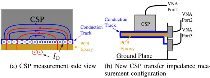
Fig. 9: CSP measurement side view and new transfer impedance measurement configuration
