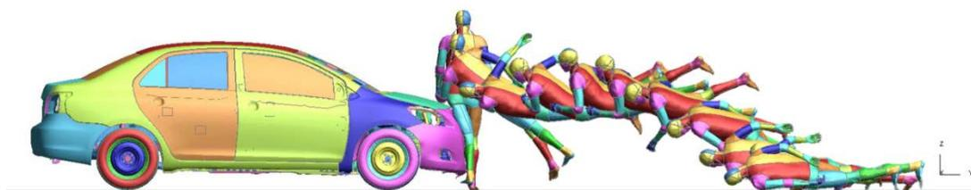
Figure 2: Typical pedestrian kinematics during collision
