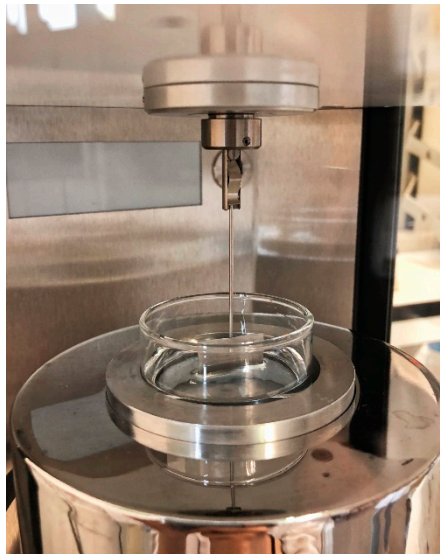
Figure 10. Surface tension measurement by KRUSS tensiometer with plate method.
