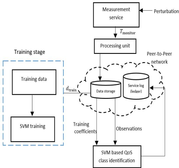
FIGURE 4. Flow diagram of QoS monitoring.
