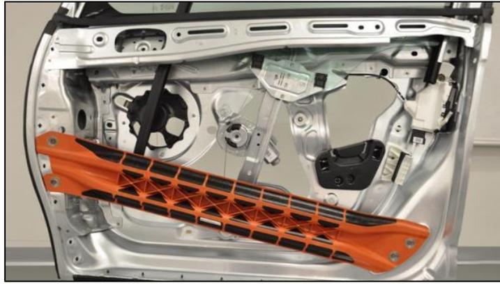
Figure 26: The location of the side-door impact beam (Winter 2013)
