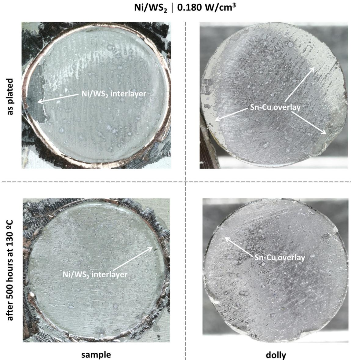
**Figure 7.3.** Images of the surface of samples and dollies after bonding tests performed on samples simulating real bearing systems consisting of a steel backing, a Pb-bronze lining deposited over the steel backing, a Ni/WS<sub>2</sub> diffusion barrier layer electrodeposited over the lining under ultrasound at 0.180 W/cm<sup>3</sup>, and an electrodeposited Sn-Cu overlay on top.
