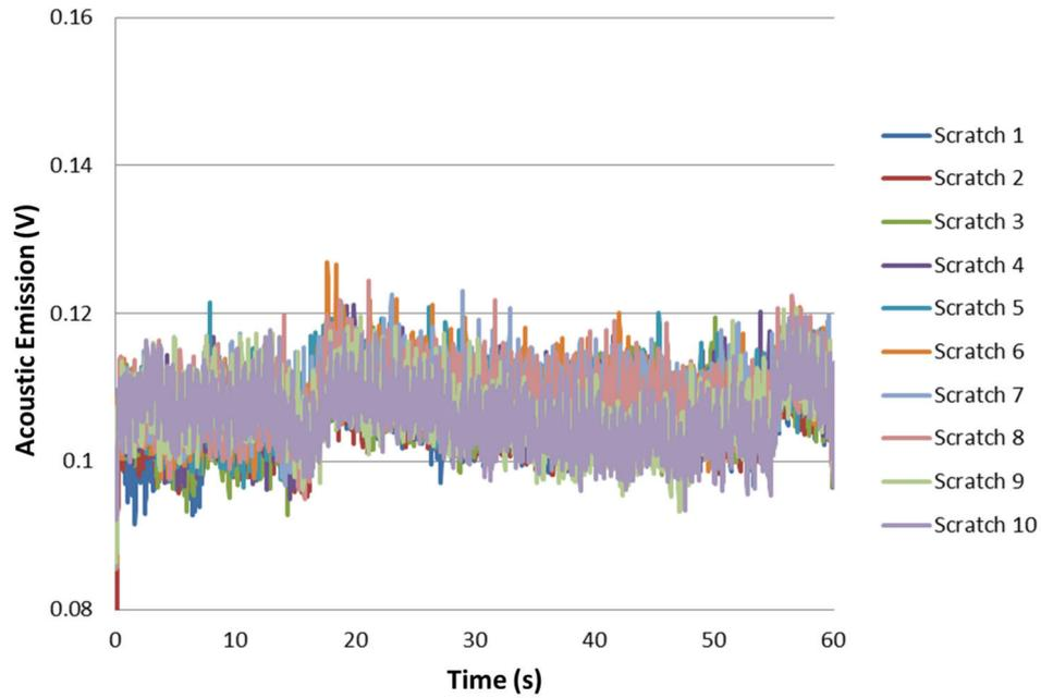
**Figure 6.5.** Acoustic emission recorded during a lubricated scratch test (10 continuous scratches) performed on a Ni coating electrodeposited under ultrasound at  $0.180 \text{ W/cm}^3$ .
