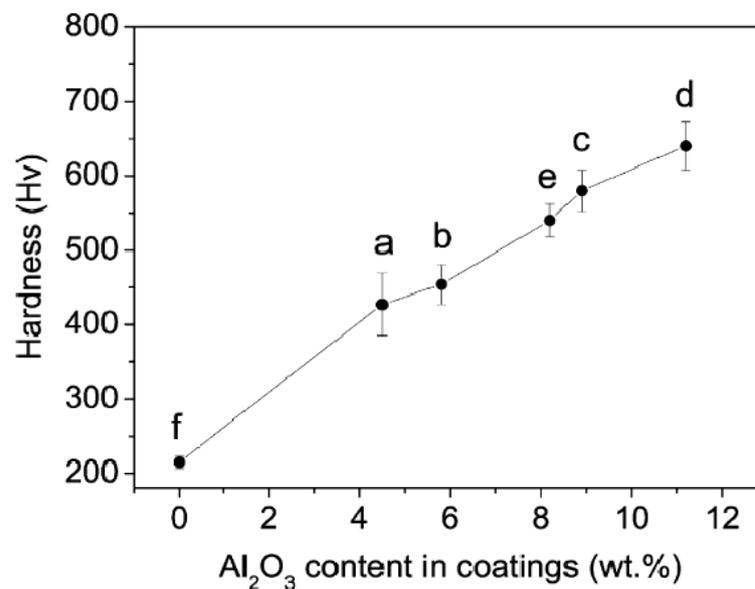
**Figure 2.12.** Hardness of Zn-Ni alloy (f) and Zn-Ni/Al<sub>2</sub>O<sub>3</sub> composite coatings fabricated under different powers: (a) 0 W cm<sup>-2</sup>; (b) 0.5 W cm<sup>-2</sup>; (c) 0.7 W cm<sup>-2</sup>; (d) 0.9 W cm<sup>-2</sup>; (e) 1.2 W cm<sup>-2</sup>. Adapted from Ref. [122].
