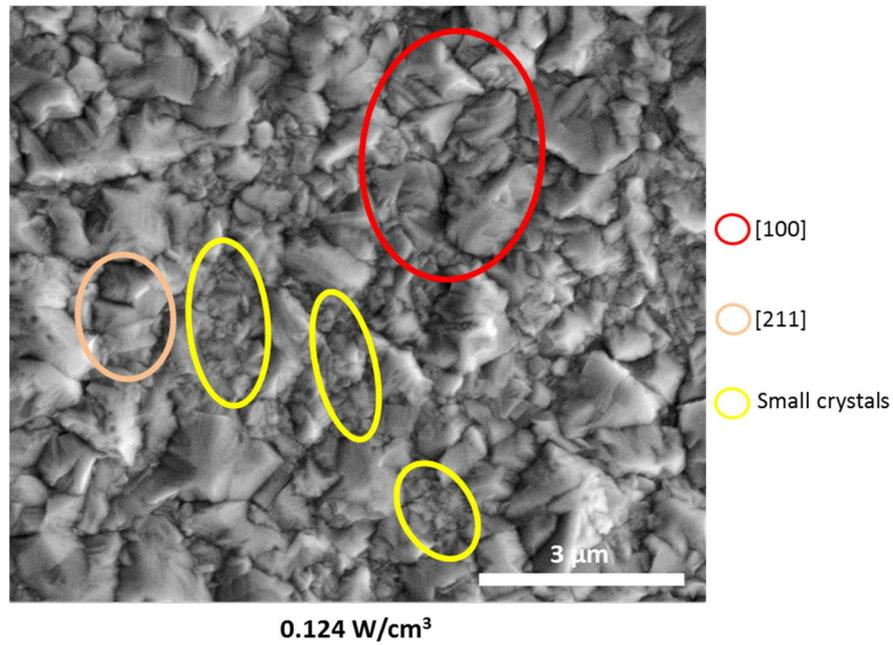
**Figure 4.15.** High magnification FIB-SEM images of the surface of Ni electrodeposited under ultrasound at 0.124 W/cm<sup>3</sup>. Electrodeposition time: 14 minutes. Current density: 4 A/dm<sup>2</sup>. Some of the crystals with a surface morphology similar to that of Ni crystals with different orientations reported by other authors [7,8,14,31] are highlighted with different colours.
