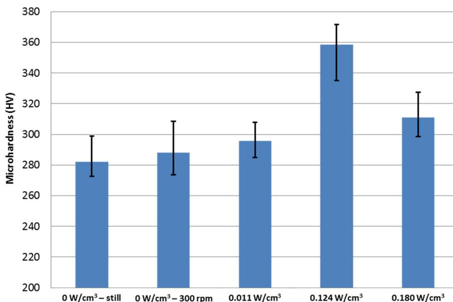
**Figure 4.19.** Microhardness values measured in the central area of the cross-section of Ni coatings ( $\approx 6 \mu\text{m}$ ) electroplated onto Cu substrates under different agitation conditions. Electrodeposition parameters:
