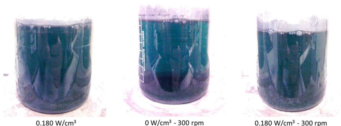
**Figure 5.3.** Appearance of Ni Watts bath + WS<sub>2</sub> dispersions (15 g/L of WS<sub>2</sub> particles) 180 minutes after dispersing the particles for 30 minutes in the electrolyte under different conditions: ultrasound at 0.180 W/cm<sup>3</sup>, mechanical agitation at 300 rpm and combined ultrasound/mechanical agitation at 0.180 W/cm<sup>3</sup> – 300 rpm. Images were edited (50% increase in brightness) to show the quality of the dispersion.
