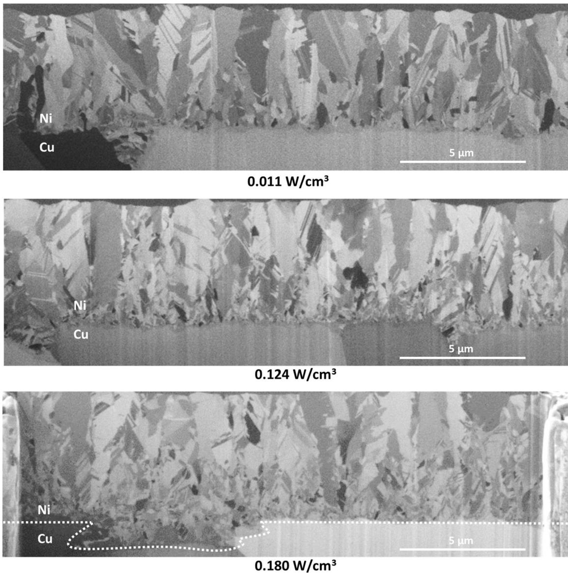
**Figure 4.18.** FIB-SEM images of the cross-section of Ni coatings deposited under ultrasound at  $0.011$ ,  $0.124$  and  $0.180 \text{ W/cm}^3$ . Electrodeposition time: 14 minutes. Current density:  $4 \text{ A/dm}^2$ .
