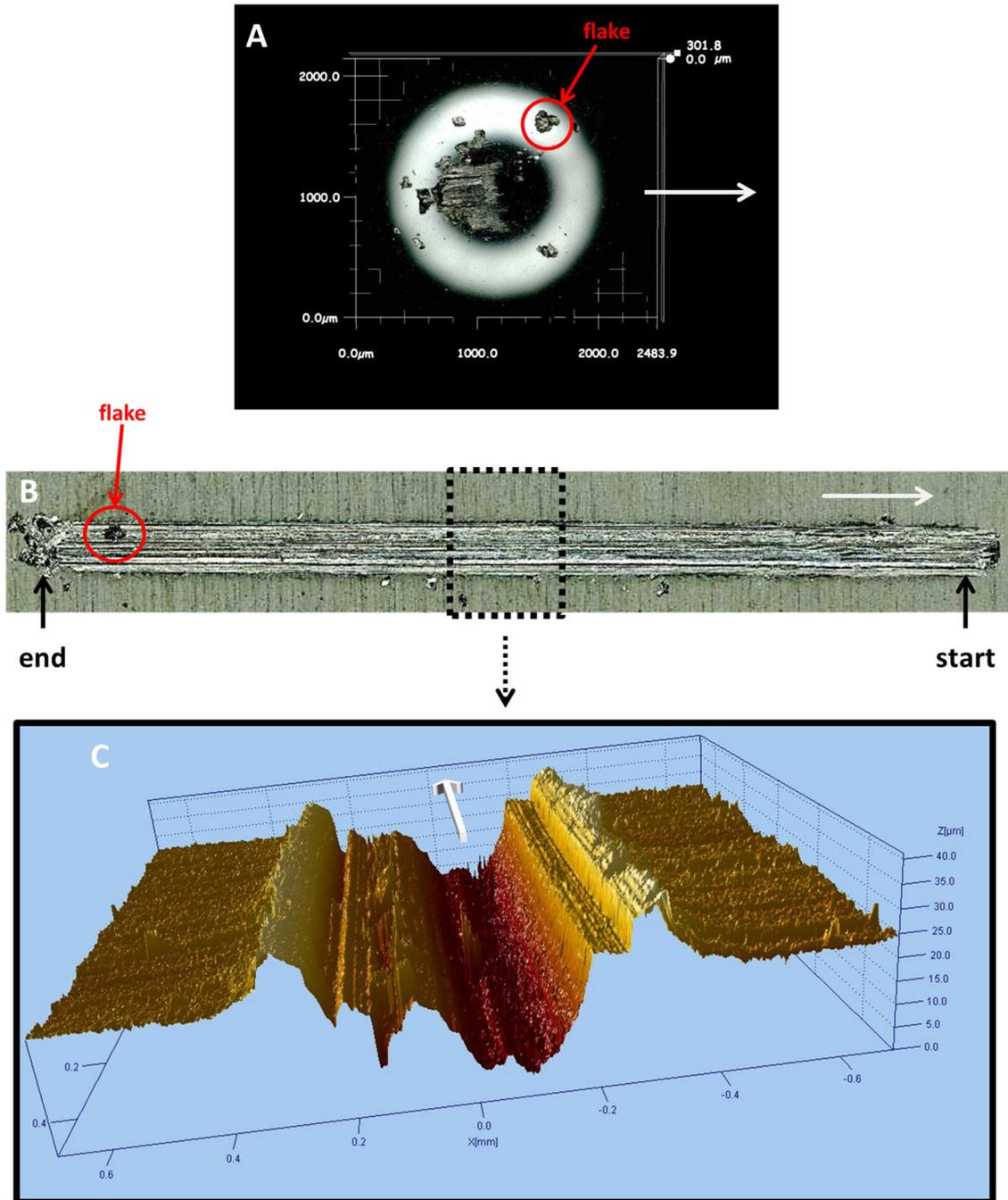
**Figure 6.24.** Images of the test ball and the wear track left by the test ball on a Ni/hBN composite coating electrodeposited under ultrasound at  $0.180 \text{ W/cm}^3$  after a non-lubricated scratch test: (A) test ball, (B) wear track left on the sample, (C) 3D depth profile on the middle area of the wear track left on the sample obtained by white light interferometry. The white arrows point the direction of the sample motion.
