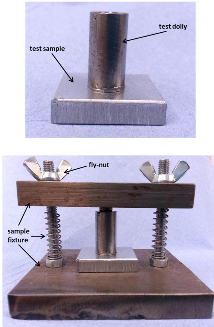
**Figure D.2.** Image showing the assembled test sample and dolly and the sample fixture.
