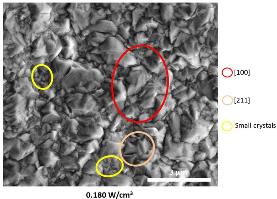
**Figure 4.16.** High magnification FIB-SEM images of the surface of Ni electrodeposited under ultrasound at 0.180 W/cm<sup>3</sup>. Electrodeposition time: 14 minutes. Current density: 4 A/dm<sup>2</sup>. Some of the crystals with a surface
