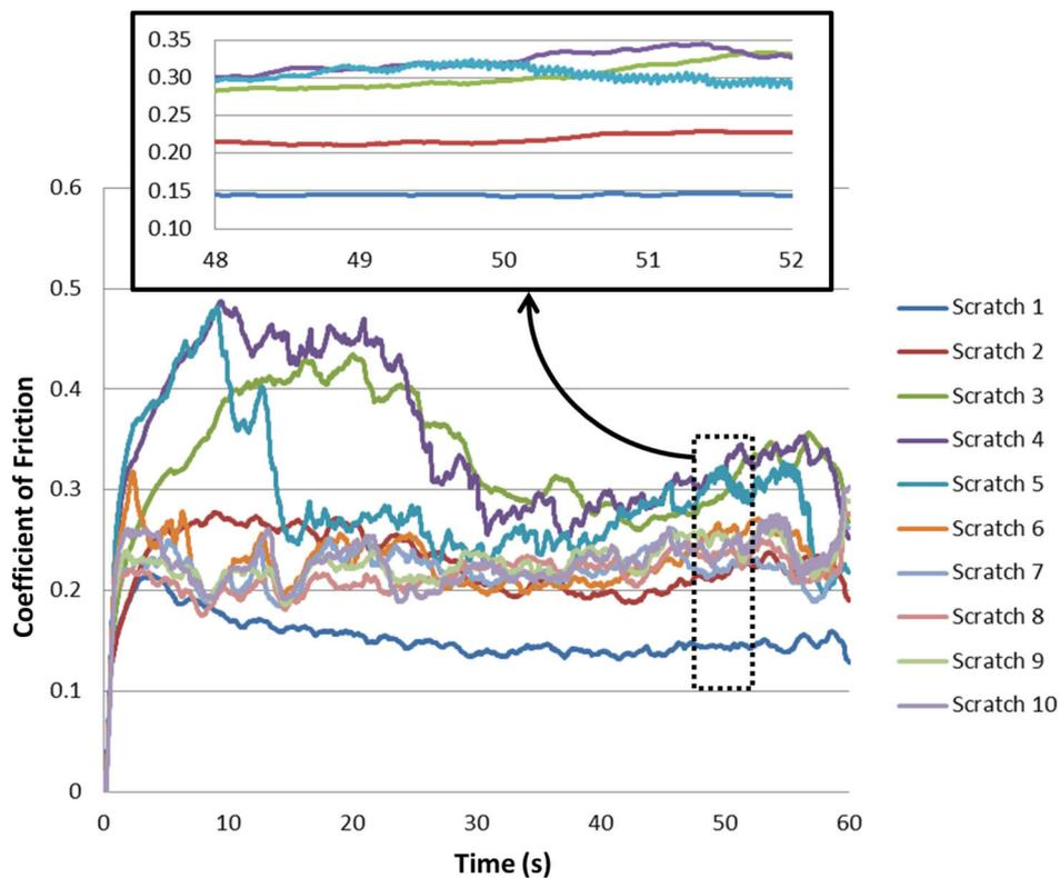
**Figure 6.22.** CoF measured during a non-lubricated scratch test (10 continuous scratches) performed on a Ni/hBN composite coating electrodeposited under ultrasound at 0.180 W/cm<sup>3</sup>. Zoomed-in graph shows when stick-slip friction started to occur (only scratches 1 to 5 are shown for better visibility).
