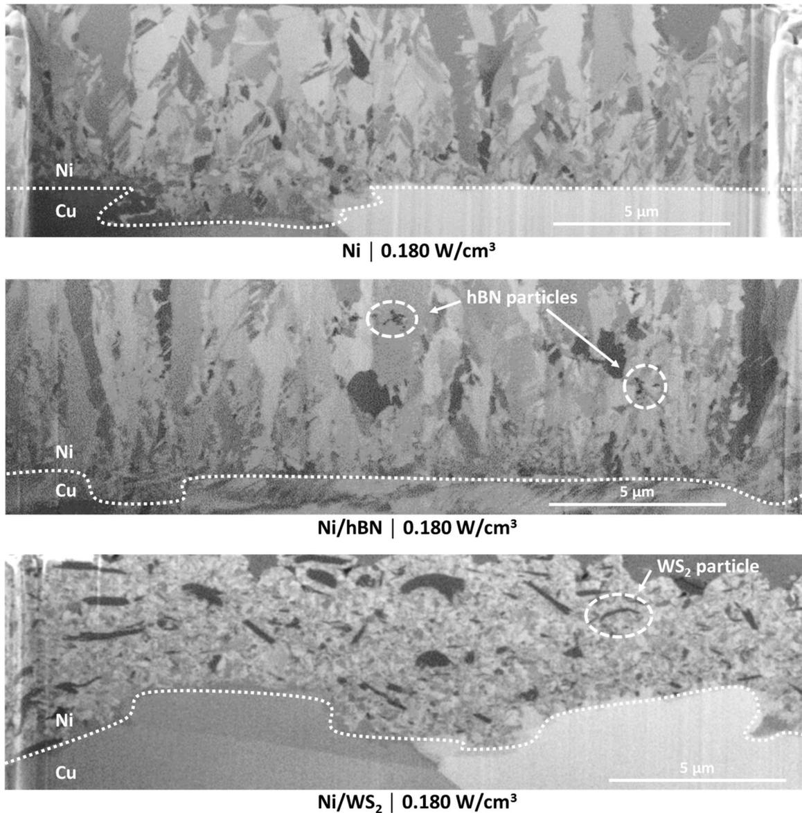
**Figure 5.30.** FIB-SEM images of the cross-section of Ni/hBN and Ni/WS<sub>2</sub> composite coatings electrodeposited under ultrasound at 0.180 W/cm<sup>3</sup>. Images of Ni coatings electrodeposited under ultrasound at 0.180 W/cm<sup>3</sup> are included for comparison purposes. Electrodeposition time: 14 minutes. Current density: 4 A/dm<sup>2</sup>.
