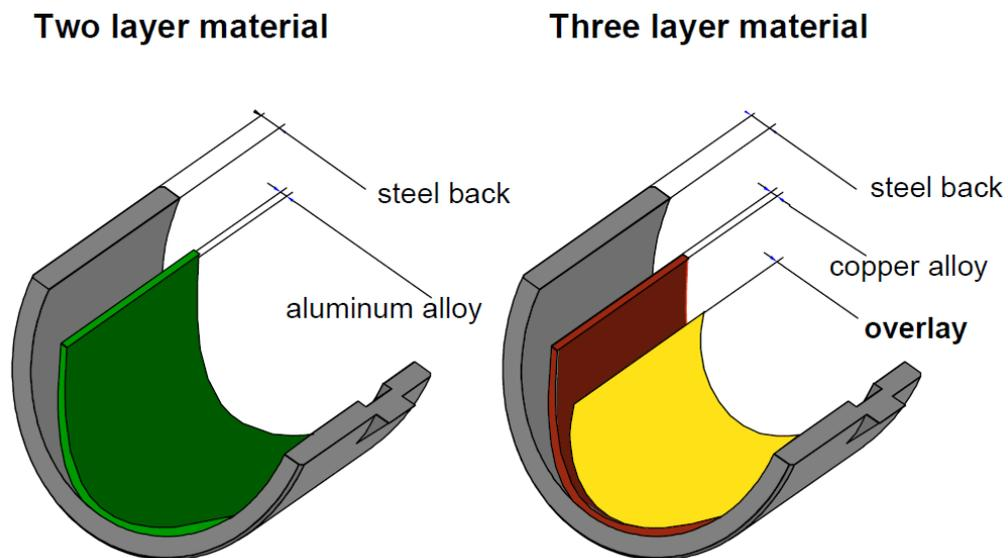
**Figure 1.4.** Layer construction of engine bearing materials. Adapted from [11].
