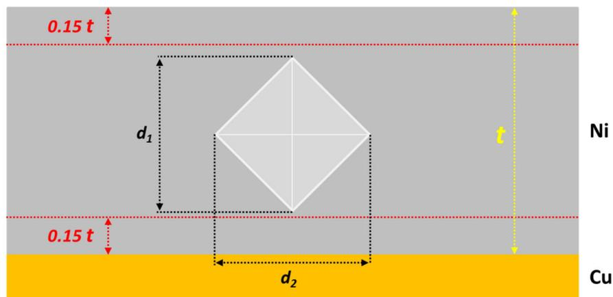
**Figure 3.4.** Diagram showing the diamond shape and the location of indentations within the coating in the Vickers microhardness tests performed on all the coatings selected for hardness tests. Thickness  $t$  was 6-7  $\mu\text{m}$  for all the samples tested during this research.
