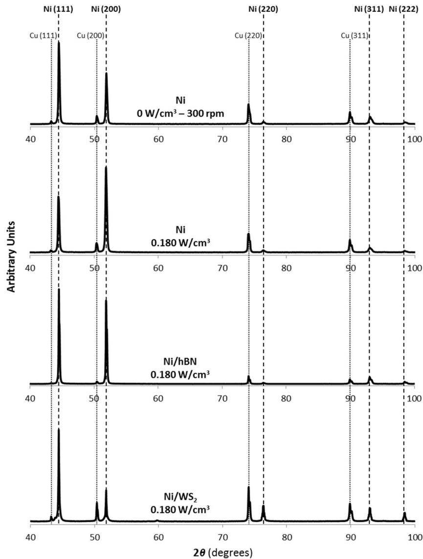
**Figure 5.20.** XRD spectra of Ni/hBN and Ni/WS<sub>2</sub> composite coatings electrodeposited under ultrasound at 0.180 W/cm<sup>3</sup> on Cu substrates. XRD spectra for pure Ni coatings electrodeposited under either mechanical agitation at 300 rpm or ultrasound at 0.180 W/cm<sup>3</sup> are included for comparison purposes. Electrodeposition time: 14 minutes. Current density: 4 A/dm<sup>2</sup>.
