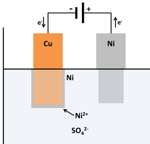
**Figure 2.1.** Electrodeposition of a metal (Ni) from a solution containing a metal salt (NiSO<sub>4</sub>).
