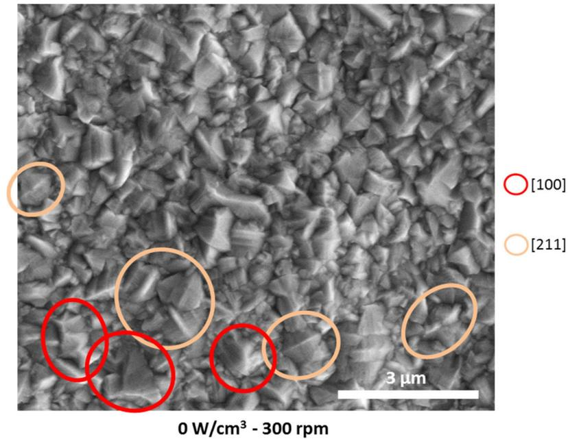
**Figure 4.13.** High magnification FIB-SEM images of the surface of Ni electrodeposited under mechanical agitation. Electrodeposition time: 14 minutes. Current density: 4 A/dm<sup>2</sup>. Some of the crystals with a surface morphology similar to that of Ni crystals with different orientations reported by other authors [7,8,14,31] are highlighted with different colours.
