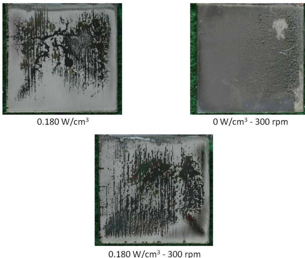
**Figure 5.17.** Examples of Ni/MoS<sub>2</sub> composite coatings electrodeposited on Cu substrates under different conditions: ultrasound at 0.180 W/cm<sup>3</sup>, mechanical agitation at 300 rpm and combined ultrasound/mechanical agitation at 0.180 W/cm<sup>3</sup> – 300 rpm. Moisture (water) stains can also be seen near upper edges of some of the samples. Electrodeposition time: 14 minutes. Current density: 4 A/dm<sup>2</sup>.
