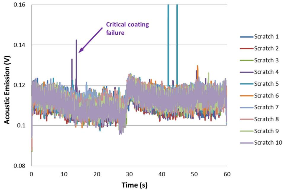
**Figure 6.20.** Acoustic emission recorded during a non-lubricated scratch test (10 continuous scratches) performed on a Ni coating electrodeposited under ultrasound at  $0.180 \text{ W/cm}^3$ .
