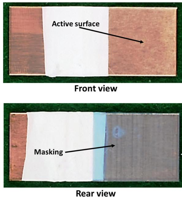
**Figure 3.2.** Cu substrates with masked back side employed in the electrodeposition experiments.
