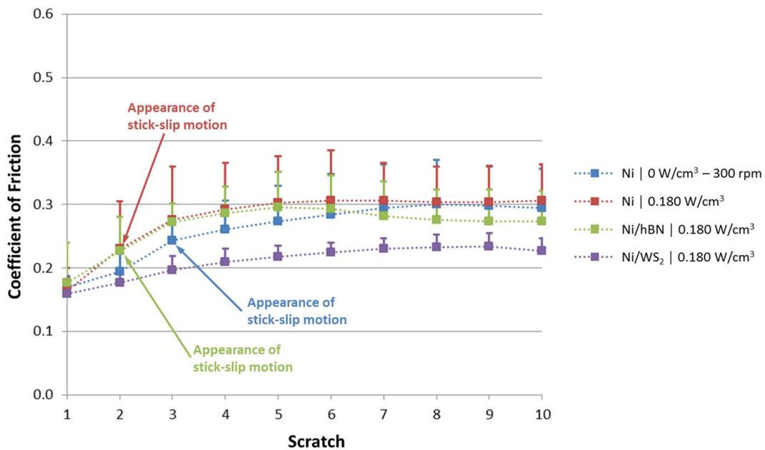
**Figure 6.13.** Average CoF estimated from a lubricated scratch test (10 continuous scratches) performed on different Ni-based coatings. Bars indicate maximum CoF values recorded during each scratch.
