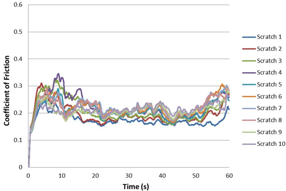
**Figure 6.25.** CoF measured during a non-lubricated scratch test (10 continuous scratches) performed on a Ni/WS<sub>2</sub> composite coating electrodeposited under ultrasound at 0.180 W/cm<sup>3</sup>.
