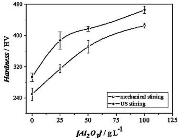
**Figure 2.9.** Effect of Al<sub>2</sub>O<sub>3</sub> concentration in the electrolyte on the hardness of Ni/Al<sub>2</sub>O<sub>3</sub> composite coating obtained under mechanical stirring and ultrasonic (US) stirring. Adapted from Ref. [101].
