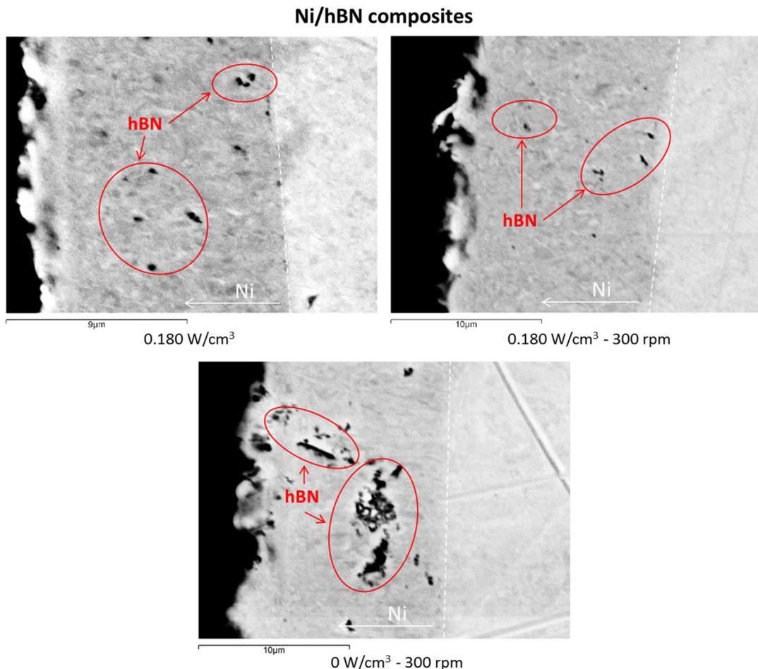
**Figure 5.16.** SEM BSE analysis of the cross-section of Ni/hBN composite coatings plated on Cu substrates under different plating conditions: ultrasound at  $0.180 \text{ W/cm}^3$ , mechanical agitation at  $300 \text{ rpm}$  and combined ultrasound/mechanical agitation at  $0.180 \text{ W/cm}^3 - 300 \text{ rpm}$ . Coatings shown here were electrodeposited for
