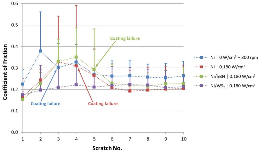
**Figure 6.28.** Average CoF estimated from a non-lubricated scratch test (10 continuous scratches) performed on different Ni-based coatings. Bars indicate maximum CoF values recorded during each scratch.
