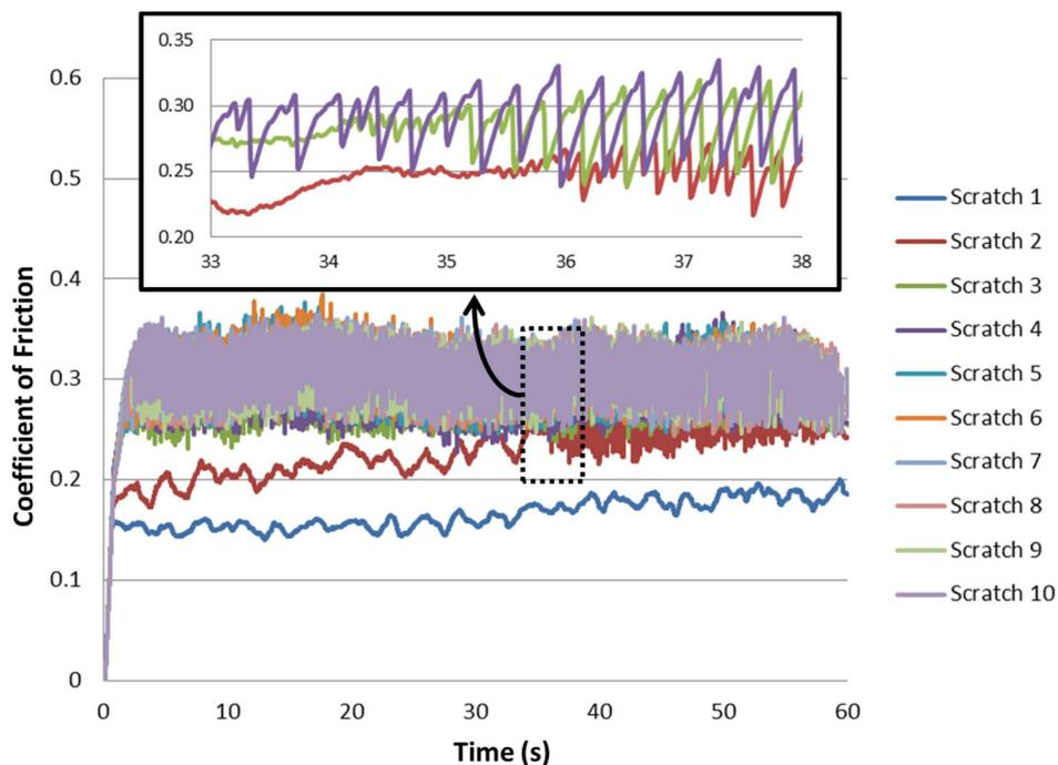
**Figure 6.4.** CoF measured during a lubricated scratch test (10 continuous scratches) performed on a Ni coating electrodeposited under ultrasound at  $0.180 \text{ W/cm}^3$ . Zoomed-in graph shows when stick-slip motion started to occur (only scratches 1 to 4 are shown for better visibility).
