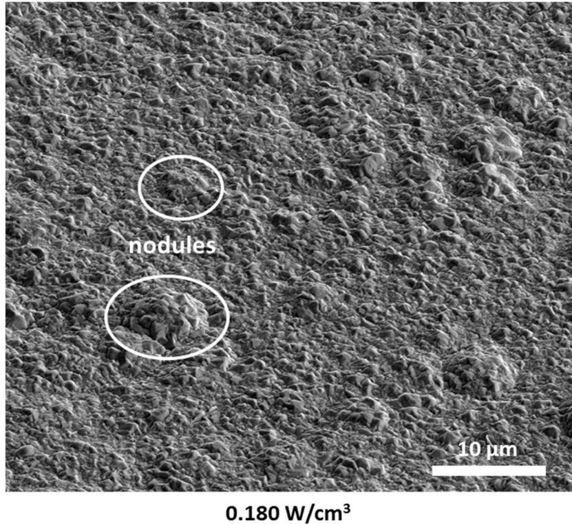
**Figure 4.10.** Tilted FIB-SEM image of the surface of Ni electrodeposited under ultrasound at 0.180 W/cm<sup>3</sup>. Electrodeposition time: 14 minutes. Current density: 4 A/dm<sup>2</sup>.
