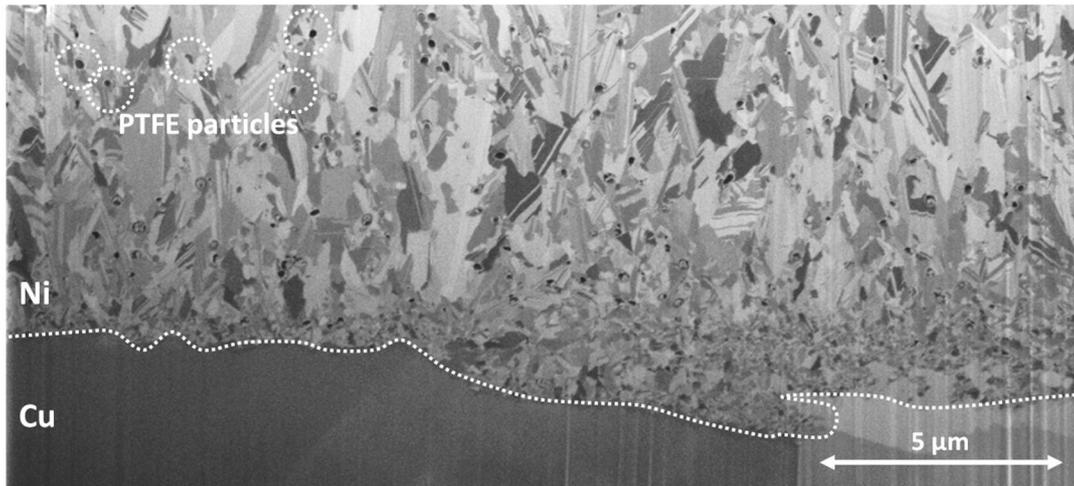
**Figure 8.1.** FIB-SEM image of the cross-section of a Ni/PTFE composite coating electrodeposited from a Ni Watts bath under current development.
