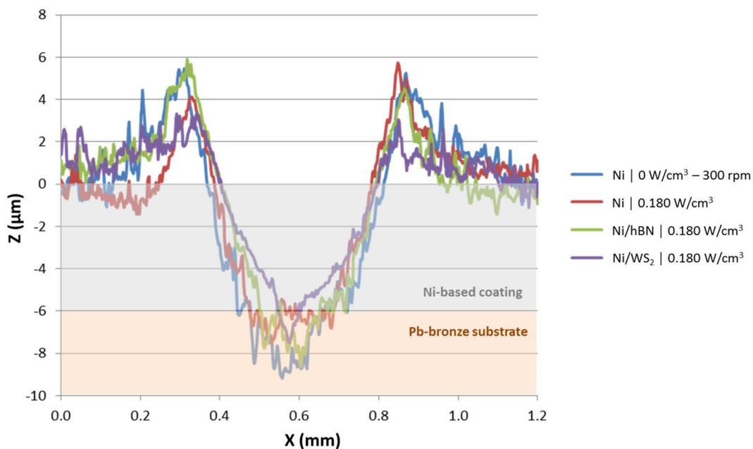
**Figure 6.14.** Cross-sectional depth profile measured at the middle of the wear track left by the test ball during a lubricated scratch test (10 continuous scratches) performed on different Ni-based coatings. Data from 3D depth profiles obtained by white light interferometry.
