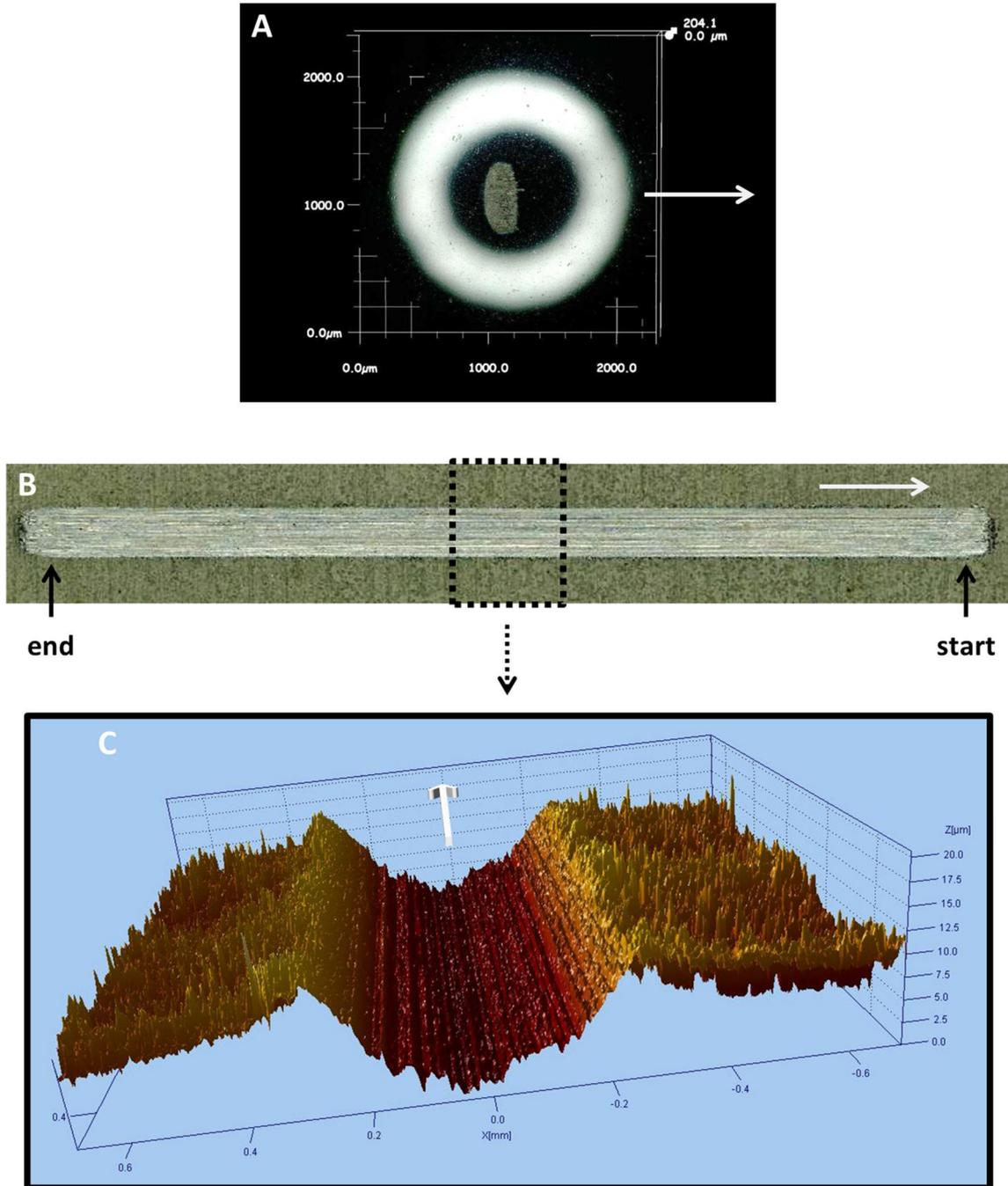
**Figure 6.3.** Images of the test ball and the wear track left by the test ball on a Ni coating electrodeposited under mechanical agitation at 300 rpm after a lubricated scratch test: (A) test ball, (B) wear track left on the sample, (C) 3D depth profile on the middle area of the wear track left on the sample obtained by white light interferometry. The white arrows point the direction of the sample motion.
