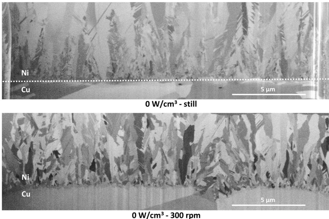
**Figure 4.17.** FIB-SEM images of the cross-section of Ni coatings deposited under silent/still conditions and mechanical agitation at 300 rpm. Electrodeposition time: 14 minutes. Current density: 4 A/dm<sup>2</sup>.
