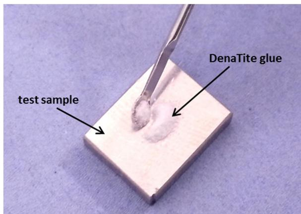
**Figure D.1.** Image showing where the DenaTite glue is spread over the surface of the test sample.
