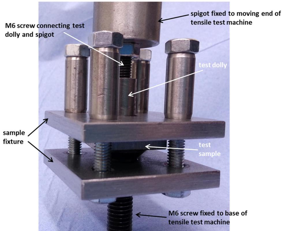
**Figure D.4.** Image showing the assembled test sample and dolly fixed in the housing that is then connected to the Hounsfield 5000 tensile test machine before the start of the bonding test.
