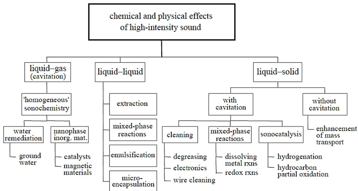
**Figure 2.3.** Classification of the chemical and physical effects of ultrasound. Adapted from Ref. [56].
