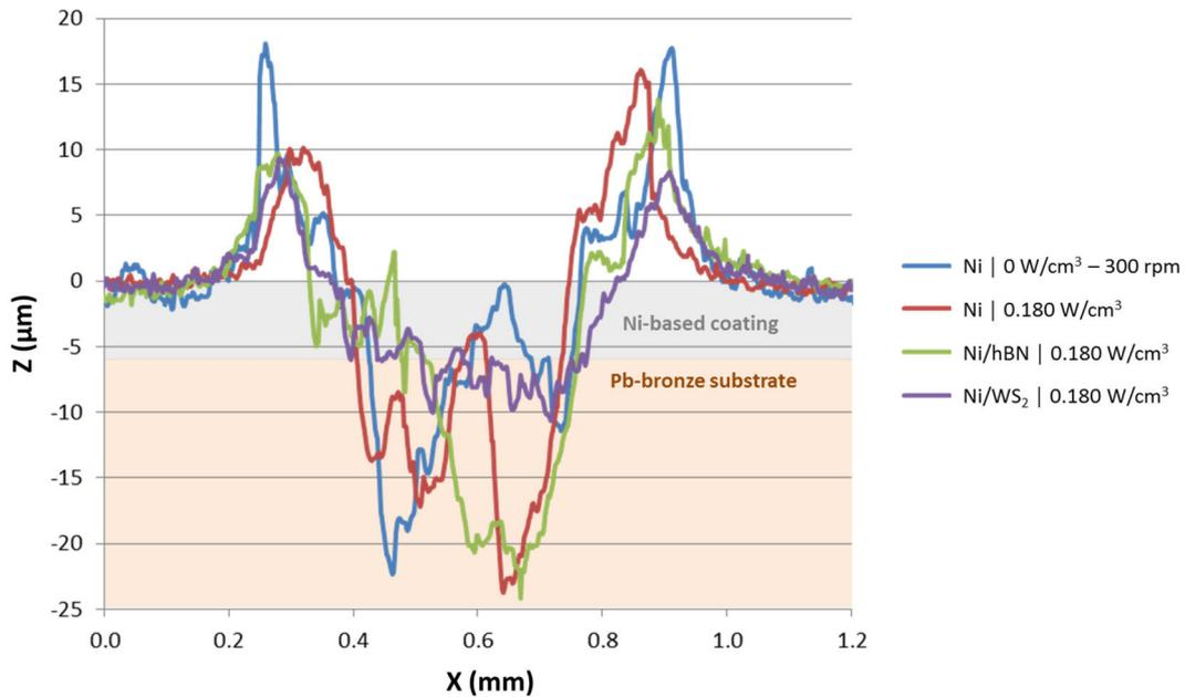
**Figure 6.29.** Depth profile measured at the middle of the wear track left by the test ball during a non-lubricated scratch test (10 continuous scratches) performed on different Ni-based coatings. Data from 3D depth profiles obtained by white light interferometry.
