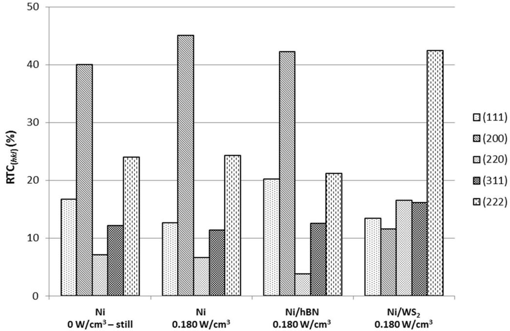
**Figure 5.22.**  $RTC_{(hkl)}$  coefficients estimated for (111), (200), (311) and (222) Ni crystal planes observed in Ni/hBN and Ni/WS<sub>2</sub> coatings electrodeposited on Cu under ultrasound at 0.180 W/cm<sup>3</sup>.  $RTC_{(hkl)}$  coefficients corresponding to pure Ni coatings electrodeposited under either mechanical agitation at 300 rpm or ultrasound at 0.180 W/cm<sup>3</sup> are included for comparison purposes. Electrodeposition time: 14 minutes. Current density: 4 A/dm<sup>2</sup>.
