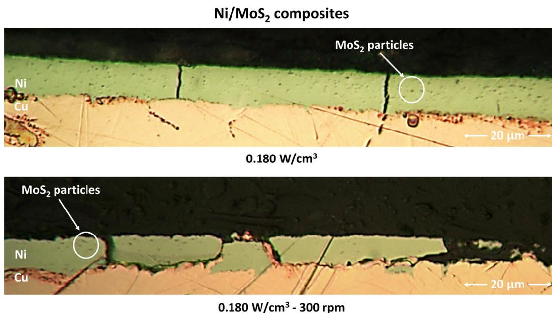
**Figure 5.18.** Examples of cross-section images of Ni/MoS<sub>2</sub> composite coatings electrodeposited on Cu substrates under different plating conditions ultrasound at 0.180 W/cm<sup>3</sup> and combined ultrasound/mechanical agitation at 0.180 W/cm<sup>3</sup> - 300 rpm. Coatings shown here were electrodeposited for longer times (24 minutes) in order to achieve thicker coatings for easier observation of the particles. Current density: 4 A/dm<sup>2</sup>.
