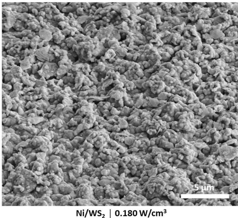
**Figure 5.25.** Tilted FIB-SEM image of the surface of a Ni/WS<sub>2</sub> composite coating electrodeposited under ultrasound at 0.180 W/cm<sup>3</sup>. Electrodeposition time: 14 minutes. Current density: 4 A/dm<sup>2</sup>.
