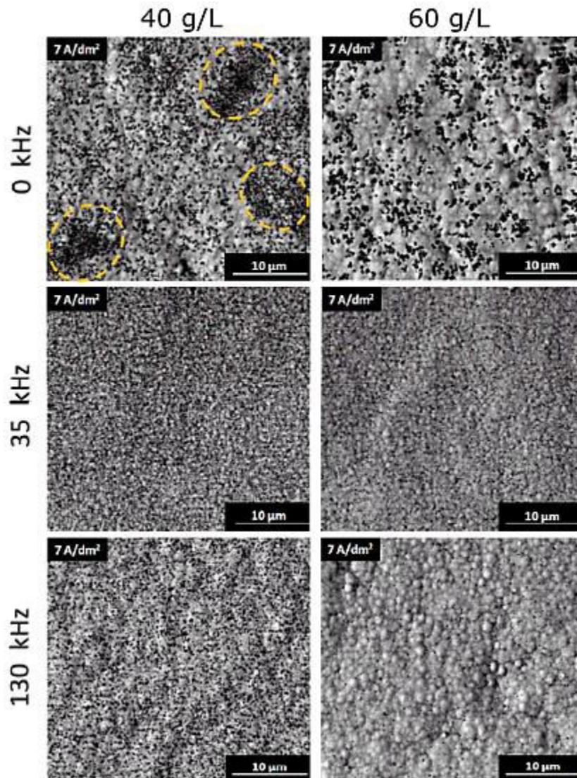
**Figure 2.10.** SEM images of surface morphology of Ni-W/Al<sub>2</sub>O<sub>3</sub> composites electrodeposited under different ultrasonic frequency from baths with different particle concentration. Adapted from Ref. [119].
