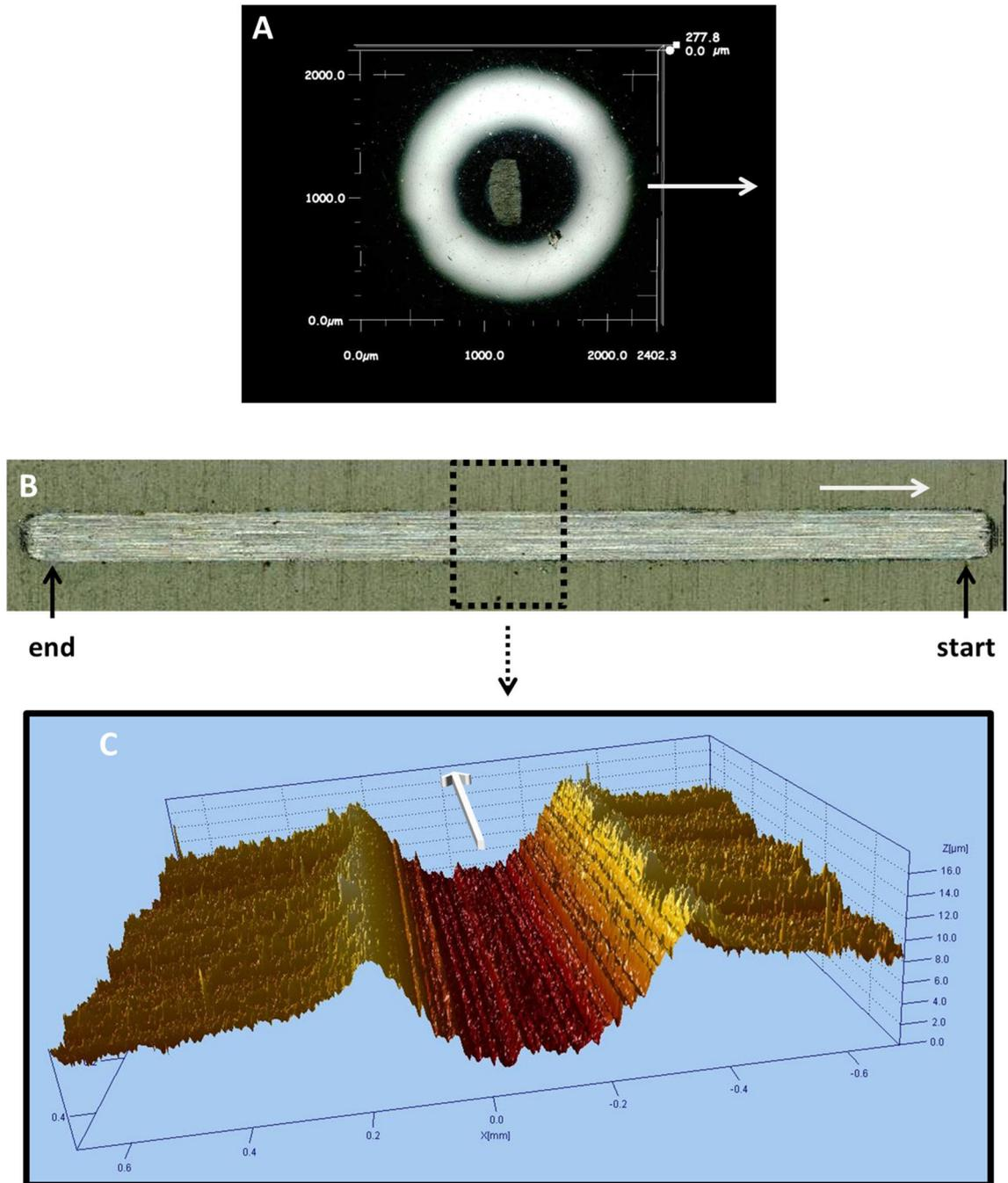
**Figure 6.6.** Images of the test ball and the wear track left by the test ball on a Ni coating electrodeposited under ultrasound at  $0.180 \text{ W/cm}^3$  after a lubricated scratch test: (A) test ball, (B) wear track left on the sample, (C) 3D depth profile on the middle area of the wear track left on the sample obtained by white light interferometry. The white arrows point the direction of the sample motion.
