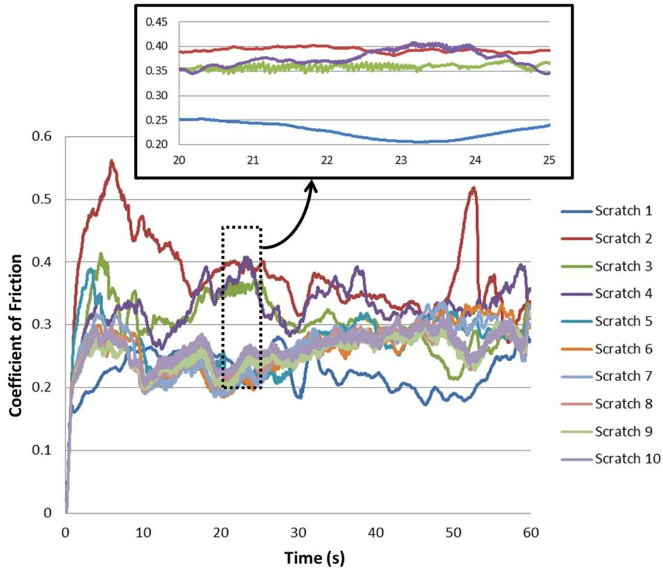
**Figure 6.16.** CoF measured during a non-lubricated scratch test (10 continuous scratches) performed on a Ni coating electrodeposited under mechanical agitation at 300 rpm. Zoomed-in graph shows when stick-slip friction started to occur (only scratches 1 to 4 are shown for better visibility).
