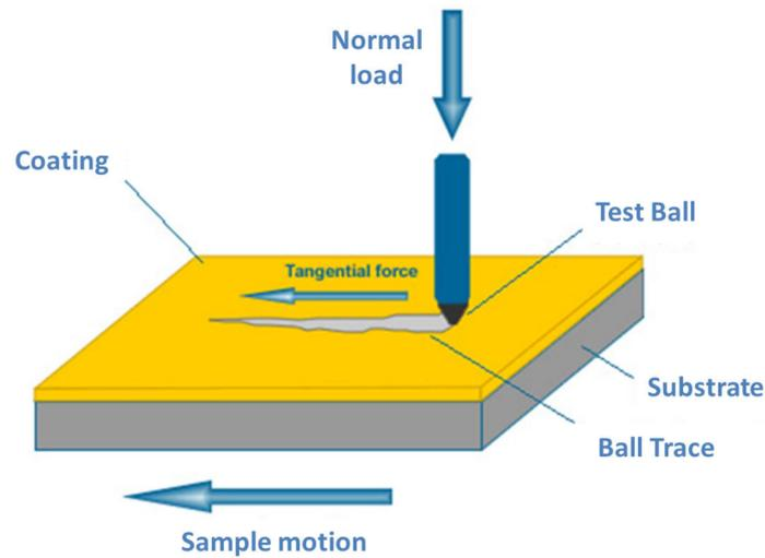
**Figure 3.5.** Schematic diagram of a 'scratch' test.
