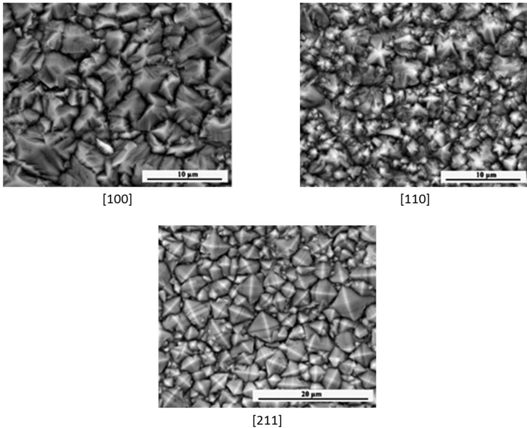
**Figure 4.11.** SEM surface micrographs presenting the typical morphology of pure Ni crystallites with [100], [110], and [210] preferred orientations. Adapted from Ref. [8].
