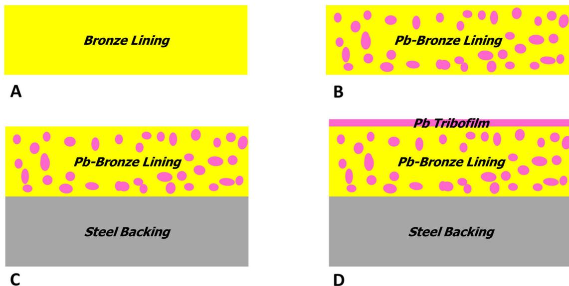
**Figure 1.5.** Evolution of basic bronze bearing materials: (A) bronze lining, (B) Pb-bronze lining, (C) Pb-bronze lining supported on steel, and (D) Pb-bronze lining supported on steel with a lead film formed on top. Adapted from [3].
