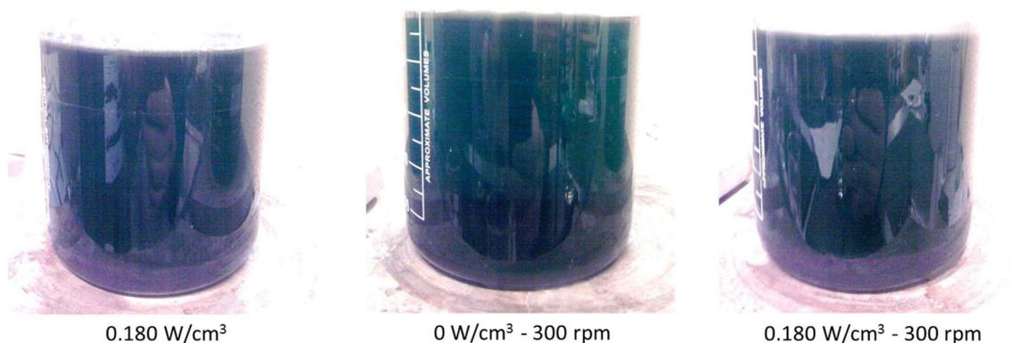
**Figure 5.9.** Appearance of Ni Watts bath + MoS<sub>2</sub> dispersions (15 g/L of MoS<sub>2</sub> particles) 240 minutes after dispersing the particles for 30 minutes in the electrolyte under different conditions: ultrasound at 0.180 W/cm<sup>3</sup>,
