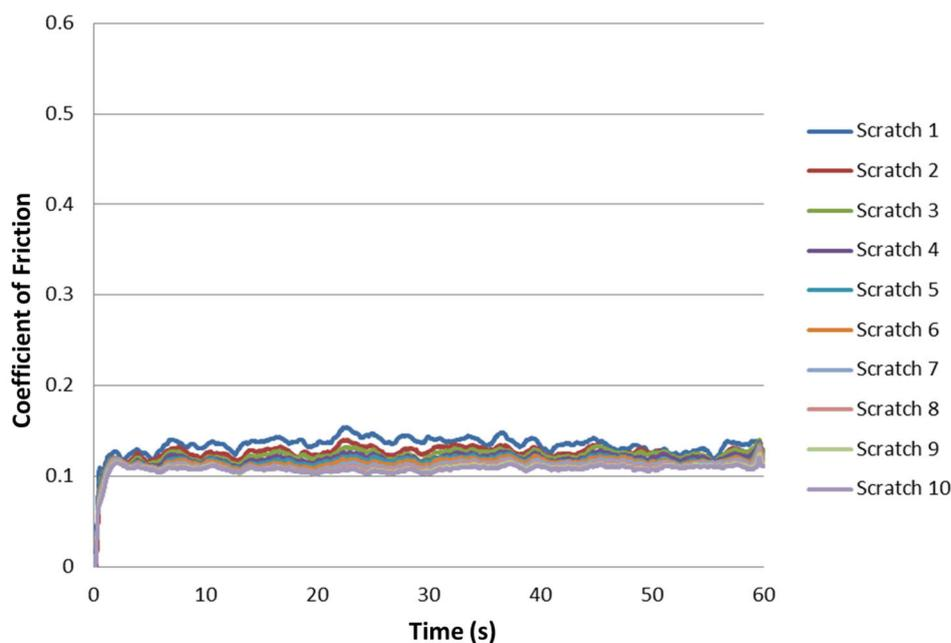
**Figure 8.3.** CoF measured during a non-lubricated scratch test (10 continuous scratches) performed on a Ni/PTFE composite coating electrodeposited from a Ni Watts bath under current development.
