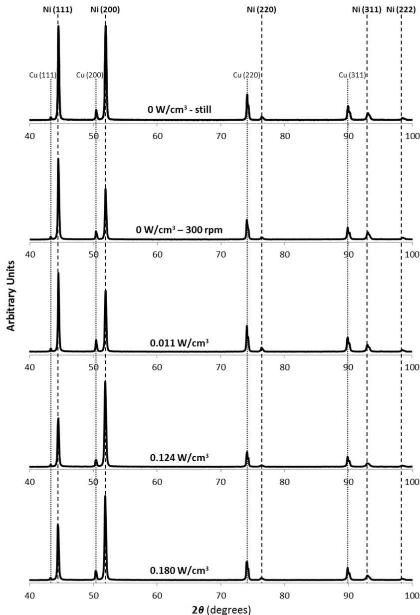
**Figure 4.3.** XRD spectra of Ni coatings electrodeposited on Cu substrates under different conditions: silent/still, mechanical agitation at 300 rpm and ultrasonic agitation at 0.011, 0.124 and 0.180 W/cm<sup>3</sup>. Peaks related to the Cu substrate are also highlighted. Electrodeposition time: 14 minutes. Current density: 4 A/dm<sup>2</sup>.
