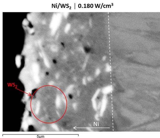
**Figure 5.13.** SEM BSE images of the cross-section of Ni/WS<sub>2</sub> composite coatings electrodeposited on Cu substrates under ultrasound at 0.180 W/cm<sup>3</sup>. Electrodeposition time: 14 minutes. Current density: 4 A/dm<sup>2</sup>.
