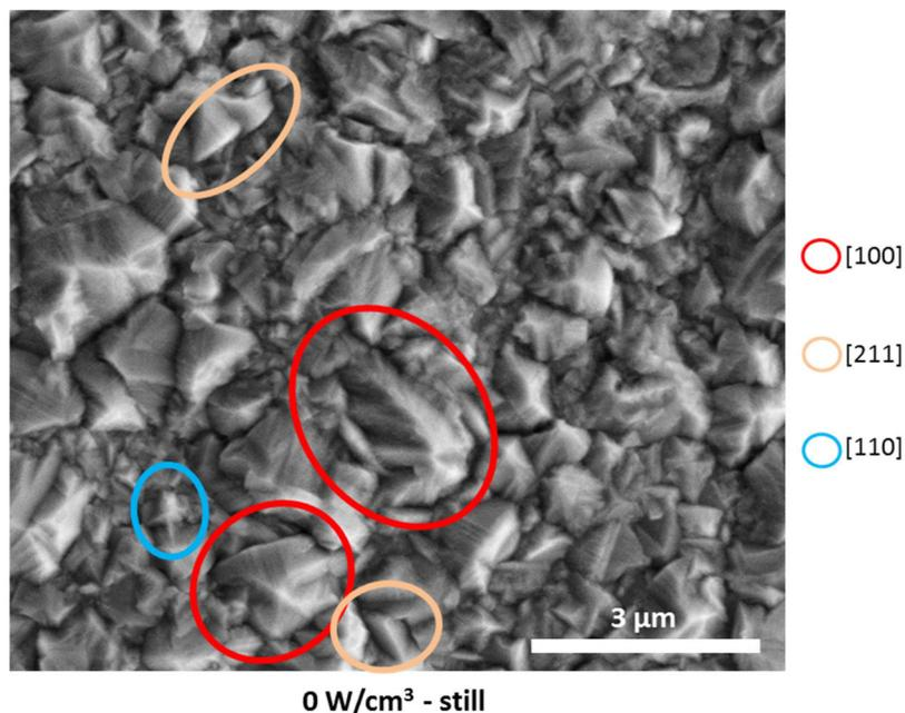
**Figure 4.12.** High magnification FIB-SEM images of the surface of Ni electrodeposited under silent/still conditions. Electrodeposition time: 14 minutes. Current density: 4 A/dm<sup>2</sup>. Some of the crystals with a surface
