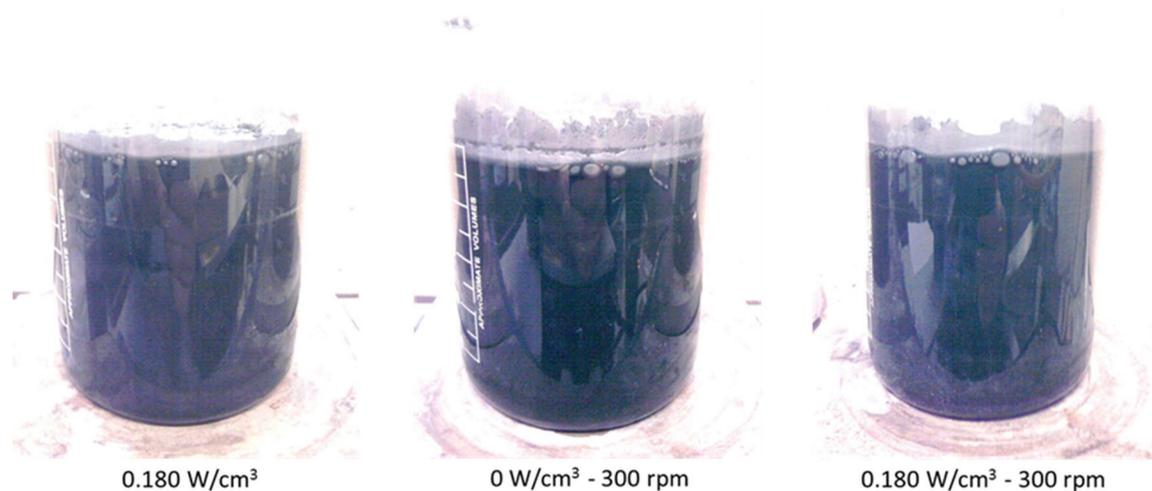
**Figure 5.1.** Appearance of Ni Watts bath + WS<sub>2</sub> dispersions (15 g/L of WS<sub>2</sub> particles) immediately after dispersing the particles for 30 minutes in the electrolyte under different conditions: ultrasound at 0.180 W/cm<sup>3</sup>, mechanical agitation at 300 rpm and combined ultrasound/mechanical agitation at 0.180 W/cm<sup>3</sup> – 300 rpm. Images were edited (50% increase in brightness) to show the quality of the dispersion.
