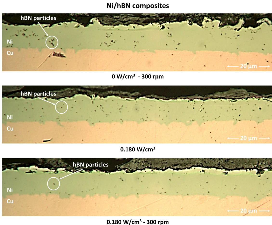
**Figure 5.15.** Examples of cross-section images of Ni/hBN composite coatings plated on Cu substrates under different plating conditions: ultrasound at 0.180 W/cm<sup>3</sup>, mechanical agitation at 300 rpm and combined
