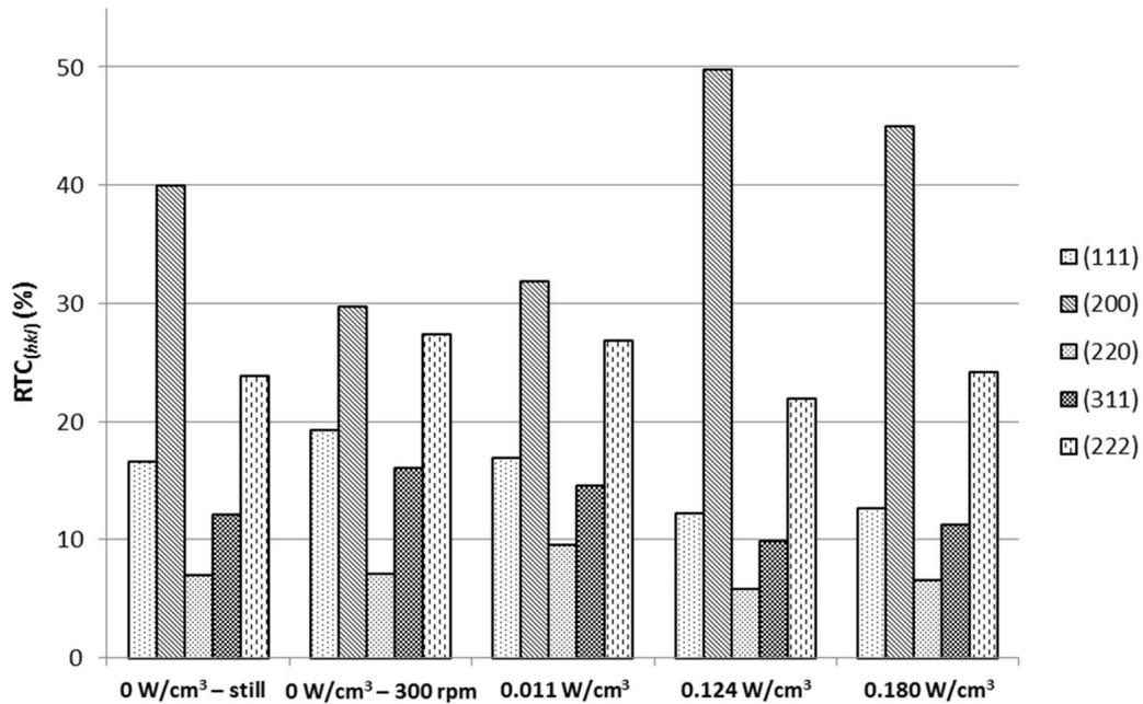
**Figure 4.4.**  $\text{RTC}_{(hkl)}$  estimated for the different crystal planes observed in Ni coatings electrodeposited under different conditions: silent/still, mechanical agitation at 300 rpm and ultrasonic agitation at 0.011, 0.124 and  $0.180 \text{ W/cm}^3$ .
