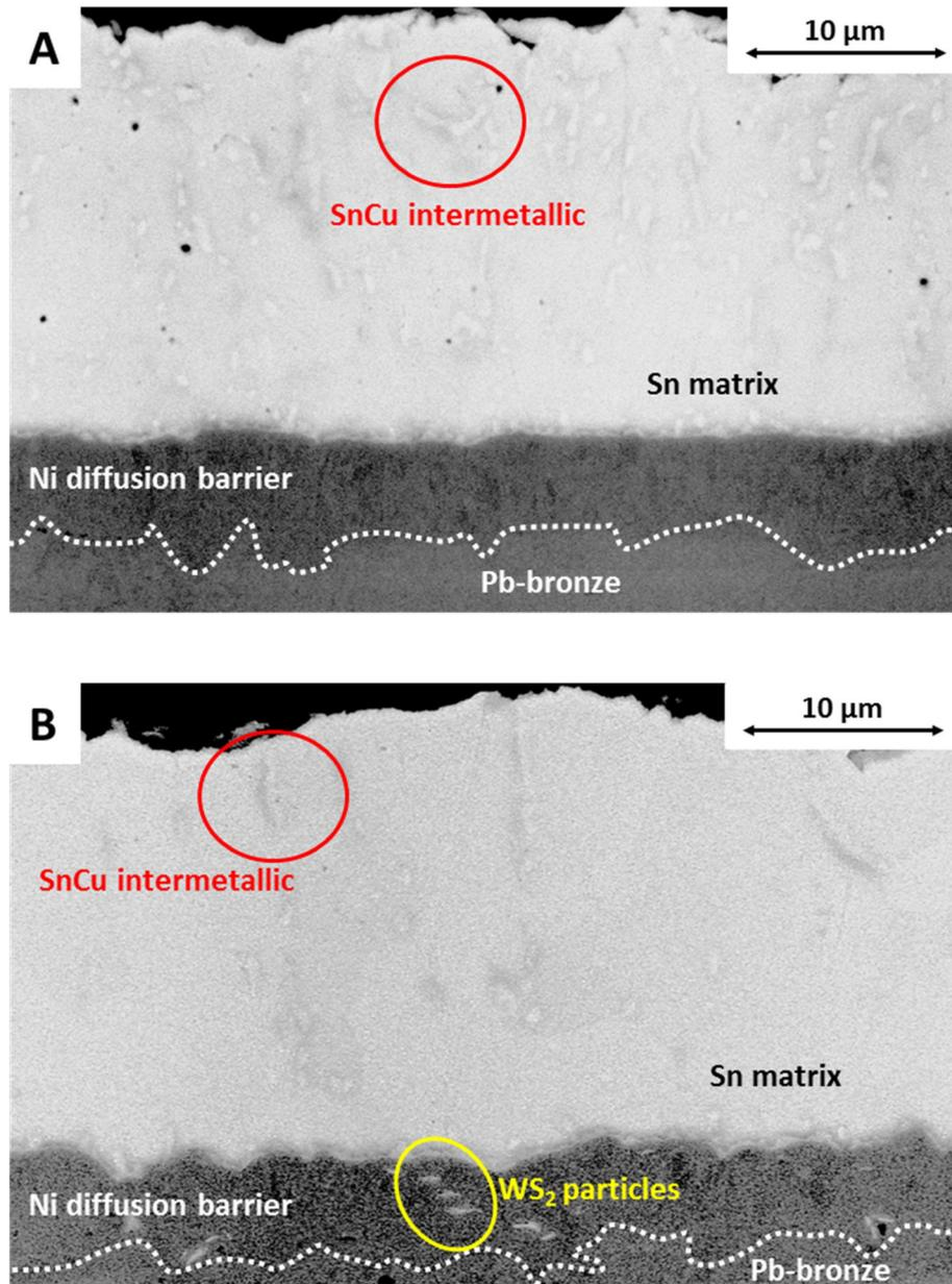
**Figure 7.5.** FEG-SEM cross-section images of samples simulating real bearing systems as plated. Samples consisted of a steel backing, a Pb-bronze lining deposited over the steel backing, a Ni-based diffusion barrier layer (either a Ni deposit produced under mechanical agitation or a Ni/WS<sub>2</sub> composites electrodeposited under ultrasound) over the lining, and an electroplated Sn-Cu overlay on top.
