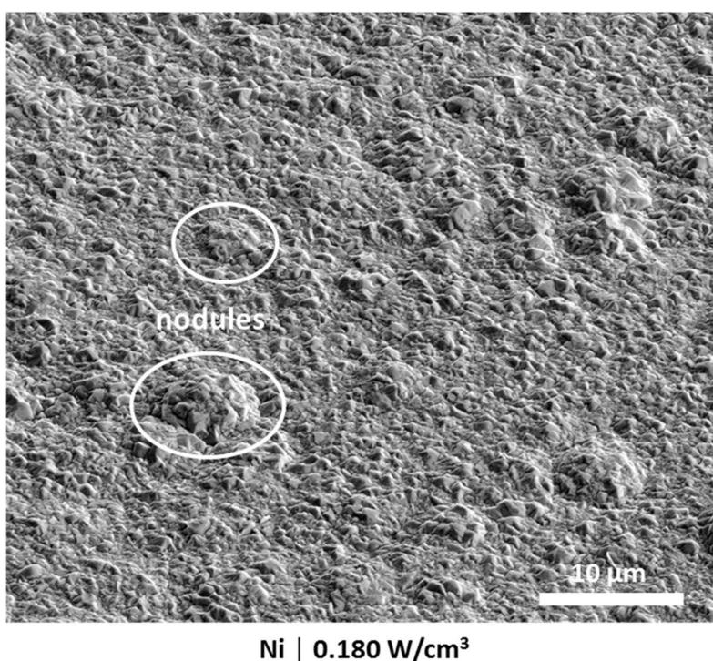
**Figure 5.24.** Tilted FIB-SEM image of the surface of a Ni coating electrodeposited under ultrasound at 0.180 W/cm<sup>3</sup>. Electrodeposition time: 14 minutes. Current density: 4 A/dm<sup>2</sup>.
