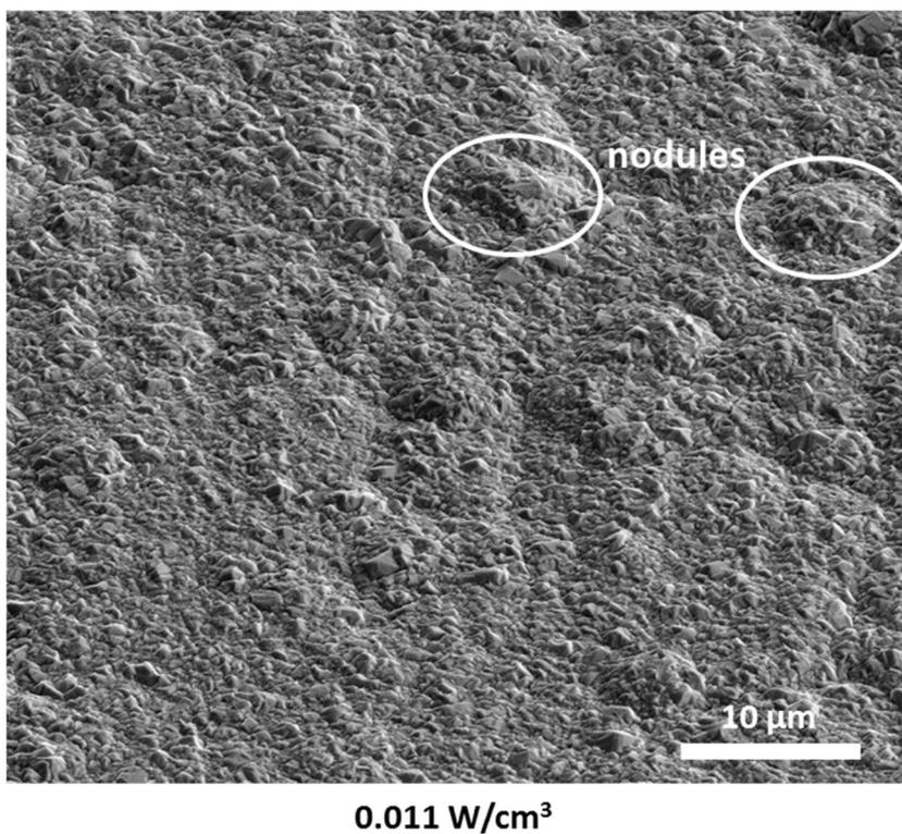
**Figure 4.8.** Tilted FIB-SEM image of the surface of Ni electrodeposited under ultrasound at 0.011 W/cm<sup>3</sup>. Electrodeposition time: 14 minutes. Current density: 4 A/dm<sup>2</sup>.
