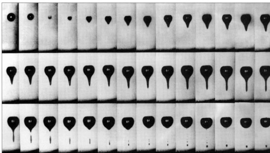
**Figure 2.7.** Example of a bubble collapsing near a solid surface and the formation of a micro-jet. Adapted from Ref. [90].
