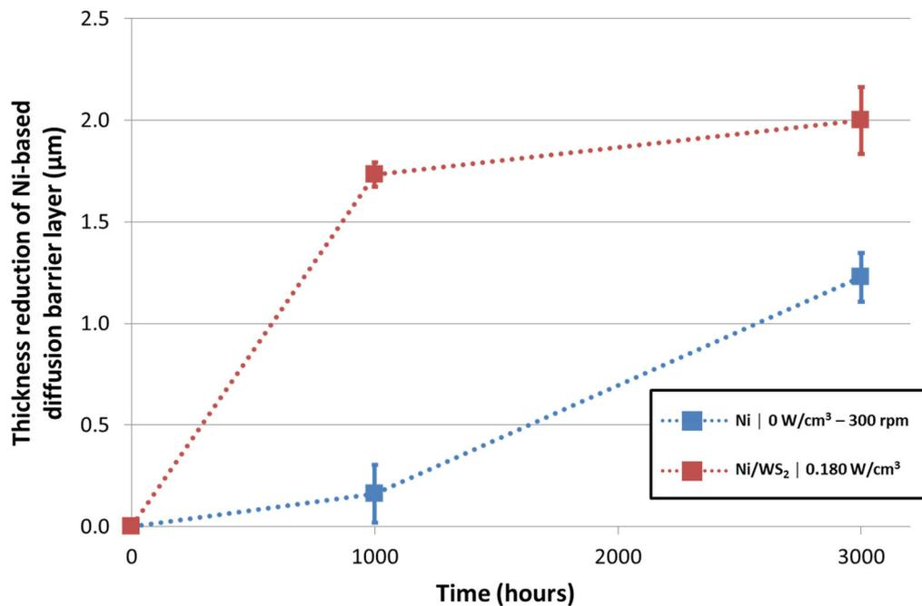
**Figure 7.9.** Reduction of the thickness of the interlayer vs. heat-treatment time for samples simulating real bearing systems. Samples consisted of a steel backing, a Pb-bronze lining deposited over the steel backing, a Ni-based diffusion barrier layer (either a Ni deposit produced under mechanical agitation or a Ni/WS<sub>2</sub> composites electrodeposited under ultrasound) over the lining, and an electroplated Sn-Cu overlay on top.
