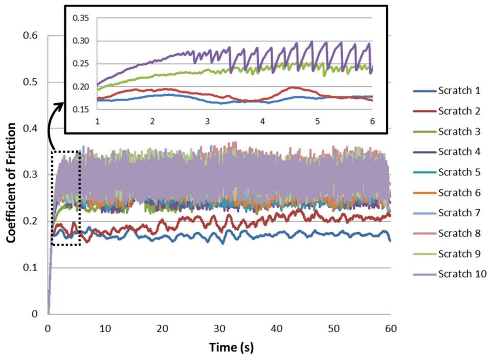
**Figure 6.1.** CoF measured during a lubricated scratch test (10 continuous scratches) performed on a Ni coating electrodeposited under mechanical agitation at 300 rpm. Zoomed-in graph shows when stick-slip motion started to occur (only scratches 1 to 4 are shown for better visibility).
