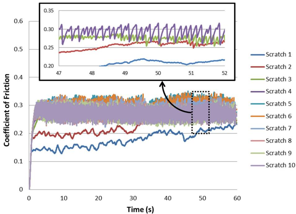
**Figure 6.7.** CoF measured during a lubricated scratch test (10 continuous scratches) performed on a Ni/hBN composite coating electrodeposited under ultrasound at  $0.180 \text{ W/cm}^3$ . Zoomed-in graph shows when stick-slip friction started to occur (only scratches 1 to 4 are shown for better visibility).
