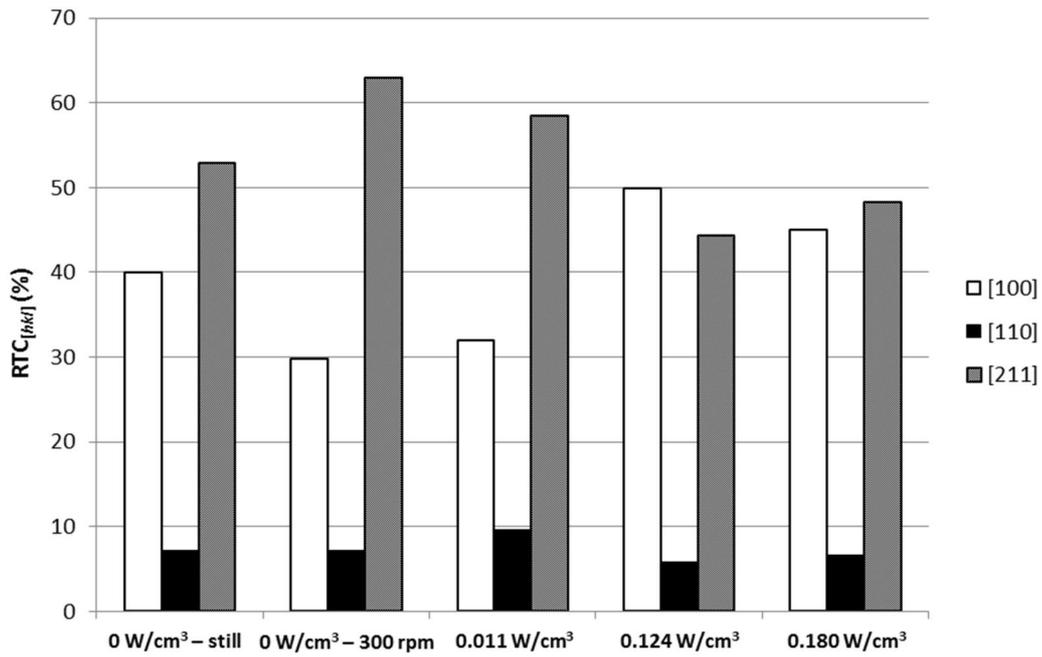
**Figure 4.5.**  $RTC_{[hkl]}$  estimated for [100], [110] and [211] orientations in Ni coatings electrodeposited under different conditions: silent/still, mechanical agitation at 300 rpm and ultrasonic agitation at 0.011, 0.124 and 0.180 W/cm<sup>3</sup>.
