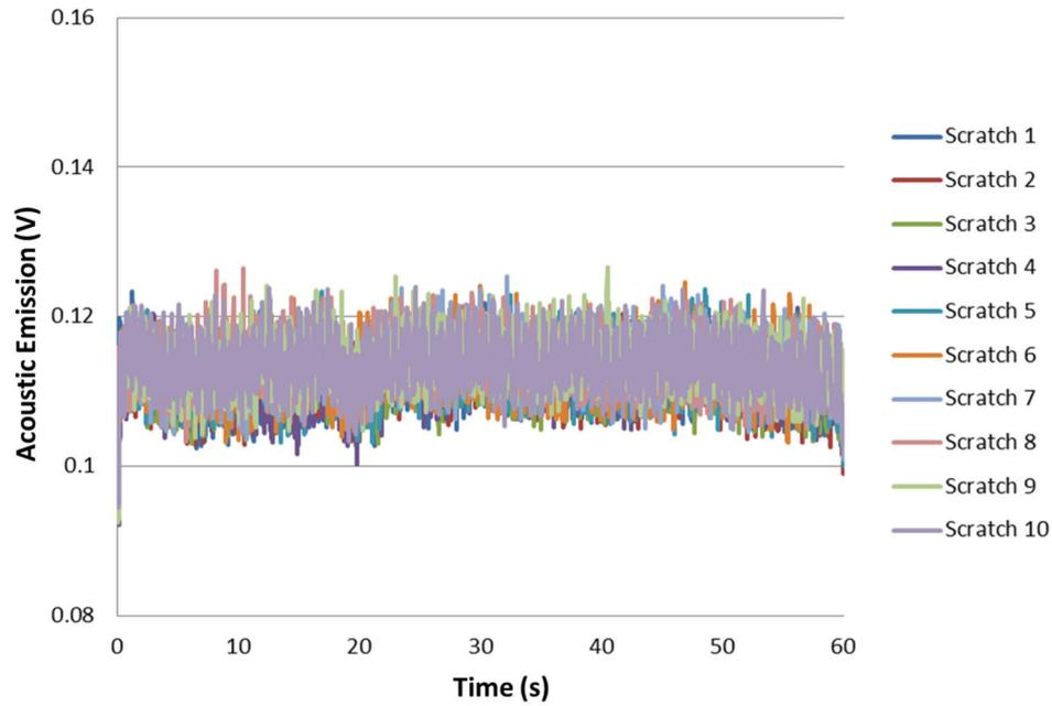
**Figure 6.8.** Acoustic emission recorded during a lubricated scratch test (10 continuous scratches) performed on a Ni/hBN composite coating electrodeposited under ultrasound at  $0.180 \text{ W/cm}^3$ .
