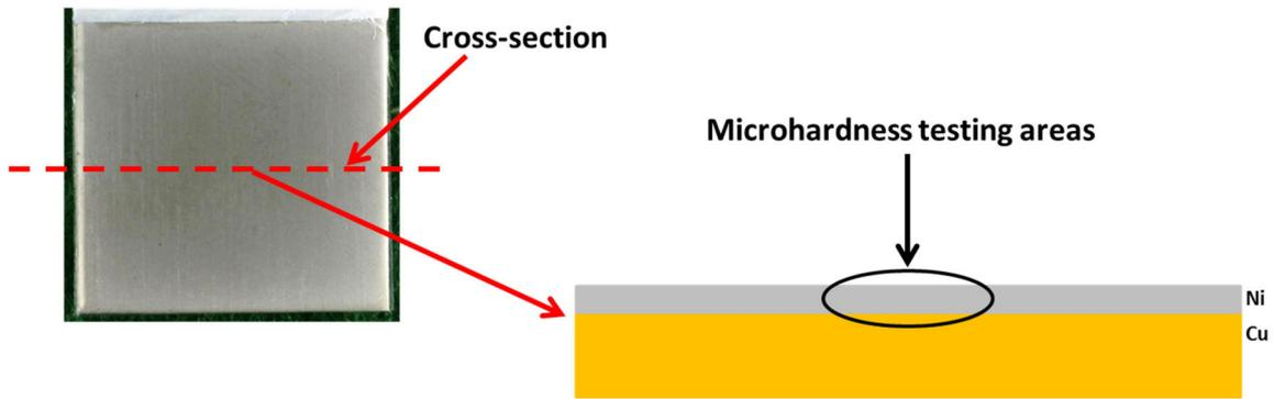
**Figure 3.3.** Area of the electroplated Ni-based coatings deposited on thick Cu substrates where microhardness was measured.
