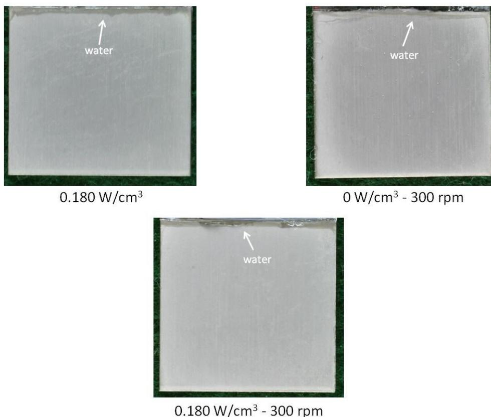
**Figure 5.14.** Examples of Ni/hBN composite coatings plated on Cu substrates under different conditions: ultrasound at 0.180 W/cm<sup>3</sup>, mechanical agitation at 300 rpm and combined ultrasound/mechanical agitation at 0.180 W/cm<sup>3</sup> - 300 rpm. Moisture (water) stains can also be seen near upper edges of the samples. Electrodeposition time: 14 minutes. Current density: 4 A/dm<sup>2</sup>.
