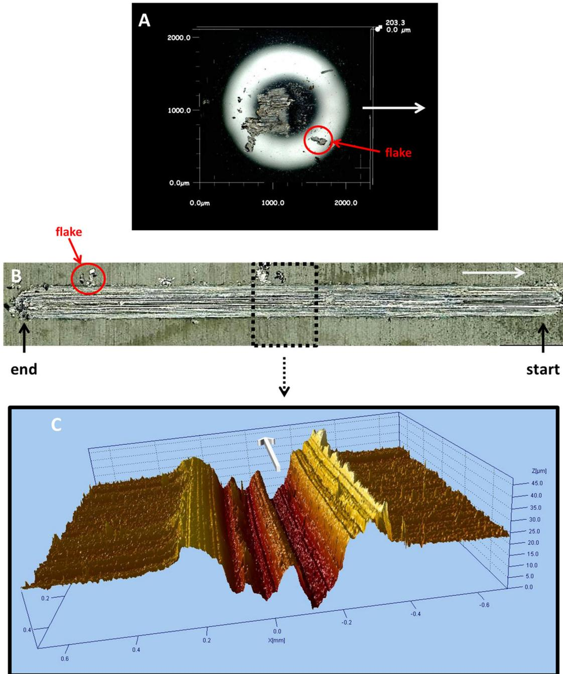
**Figure 6.21.** Images of the test ball and the wear track left by the test ball on a Ni coating electrodeposited under ultrasound at  $0.180 \text{ W/cm}^3$  after a non-lubricated scratch test: (A) test ball, (B) wear track left on the sample, (C) 3D depth profile on the middle area of the wear track left on the sample obtained by white light interferometry. The white arrows point the direction of the sample motion.
