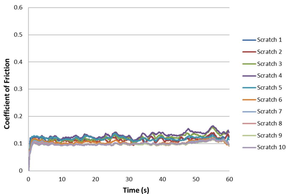
**Figure 8.2.** CoF measured during a lubricated scratch test (10 continuous scratches) performed on a Ni/PTFE composite coating electrodeposited from a Ni Watts bath under current development.
