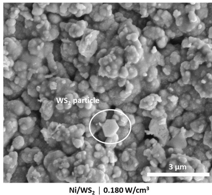
**Figure 5.28.** High magnification FIB-SEM image of the surface of a Ni/WS<sub>2</sub> composite coating electrodeposited under ultrasound at 0.180 W/cm<sup>3</sup>. Electrodeposition time: 14 minutes. Current density: 4 A/dm<sup>2</sup>.
