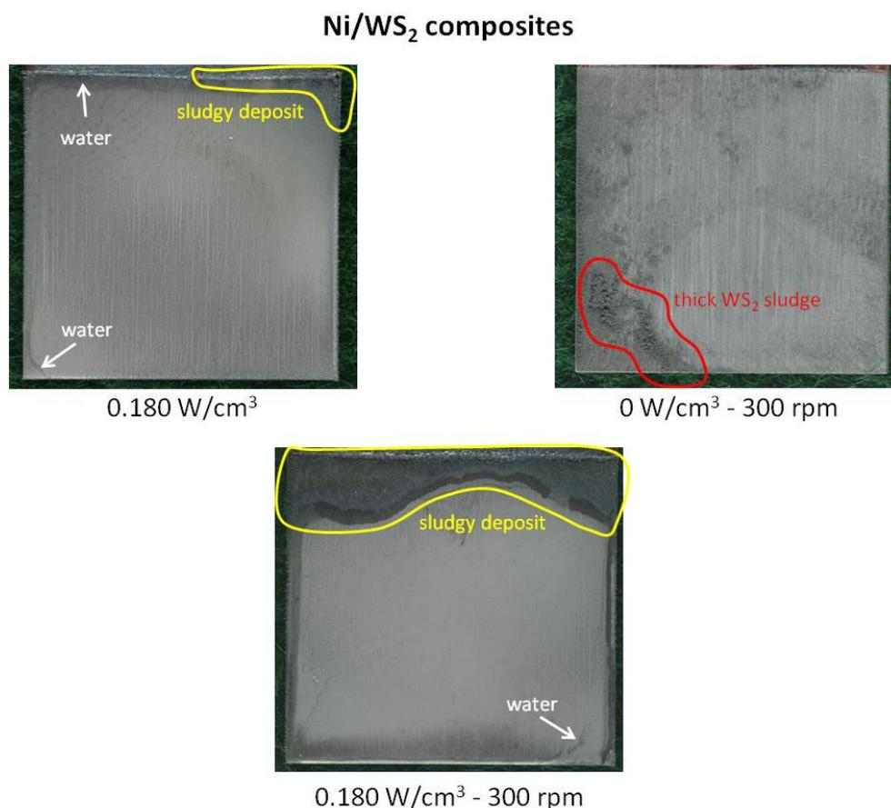
**Figure 5.11.** Examples of Ni/WS<sub>2</sub> composite coatings electrodeposited on Cu substrates under different conditions: ultrasound at 0.180 W/cm<sup>3</sup>, mechanical agitation at 300 rpm and combined ultrasound/mechanical
