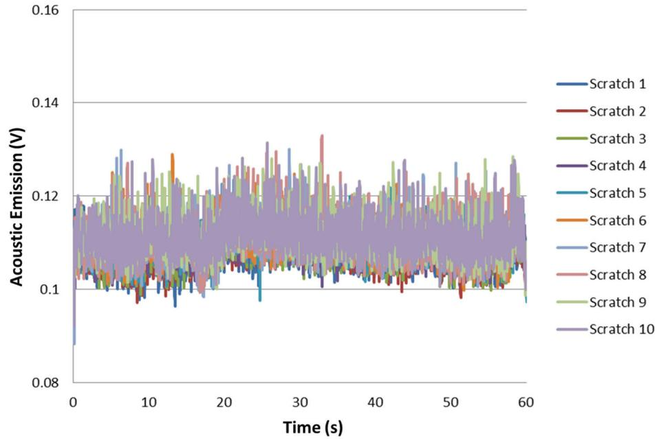
**Figure 6.2.** Acoustic emission recorded during a lubricated scratch test (10 continuous scratches) performed on a Ni coating electrodeposited under mechanical agitation at 300 rpm.
