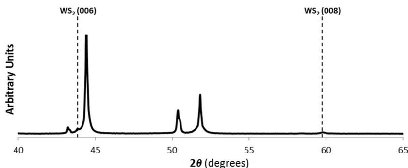
**Figure 5.21.** Zoomed XRD spectra of a Ni/WS<sub>2</sub> composite coating electrodeposited under ultrasound at 0.180 W/cm<sup>3</sup> on Cu substrates. Scan rate = 0.1 degree/s. (006) and (008) crystal planes associated to the presence of WS<sub>2</sub> are highlighted. Electrodeposition time: 14 minutes. Current density: 4 A/dm<sup>2</sup>.
