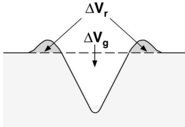
**Figure 6.15.** Schematic diagram of the cross-sectional profile of the wear track formed by abrasive wear showing  $\Delta V_r$  and  $\Delta V_g$ . Adapted from [4].
