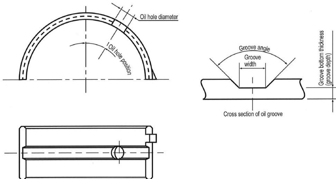
**Figure 1.3.** Definition of oil hole and oil groove in a half-shell bearing. Adapted from [4].
