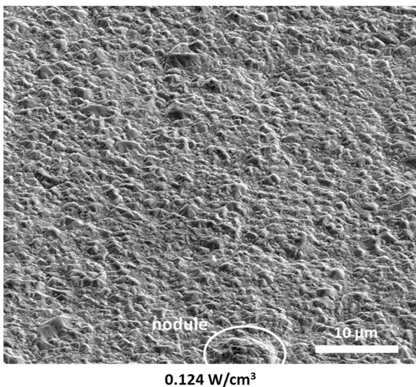
**Figure 4.9.** Tilted FIB-SEM image of the surface of Ni electrodeposited under ultrasound at 0.124 W/cm<sup>3</sup>. Electrodeposition time: 14 minutes. Current density: 4 A/dm<sup>2</sup>.
