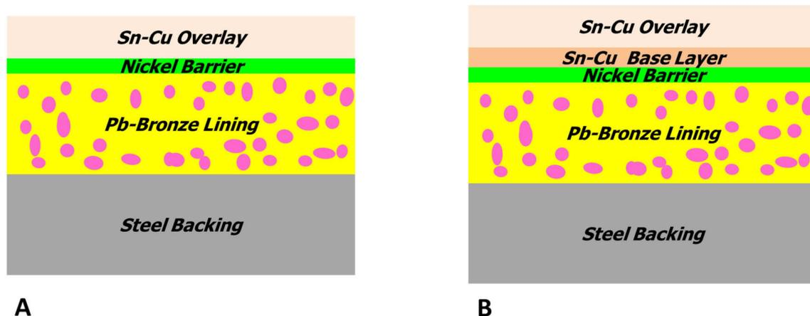
**Figure 1.7.** Pb-free, Sn-based overlays electrodeposited on bronze-based bearing materials: (A) Sn-Cu overlay, (B) Sn-Cu multilayer system. Adapted from [3].
