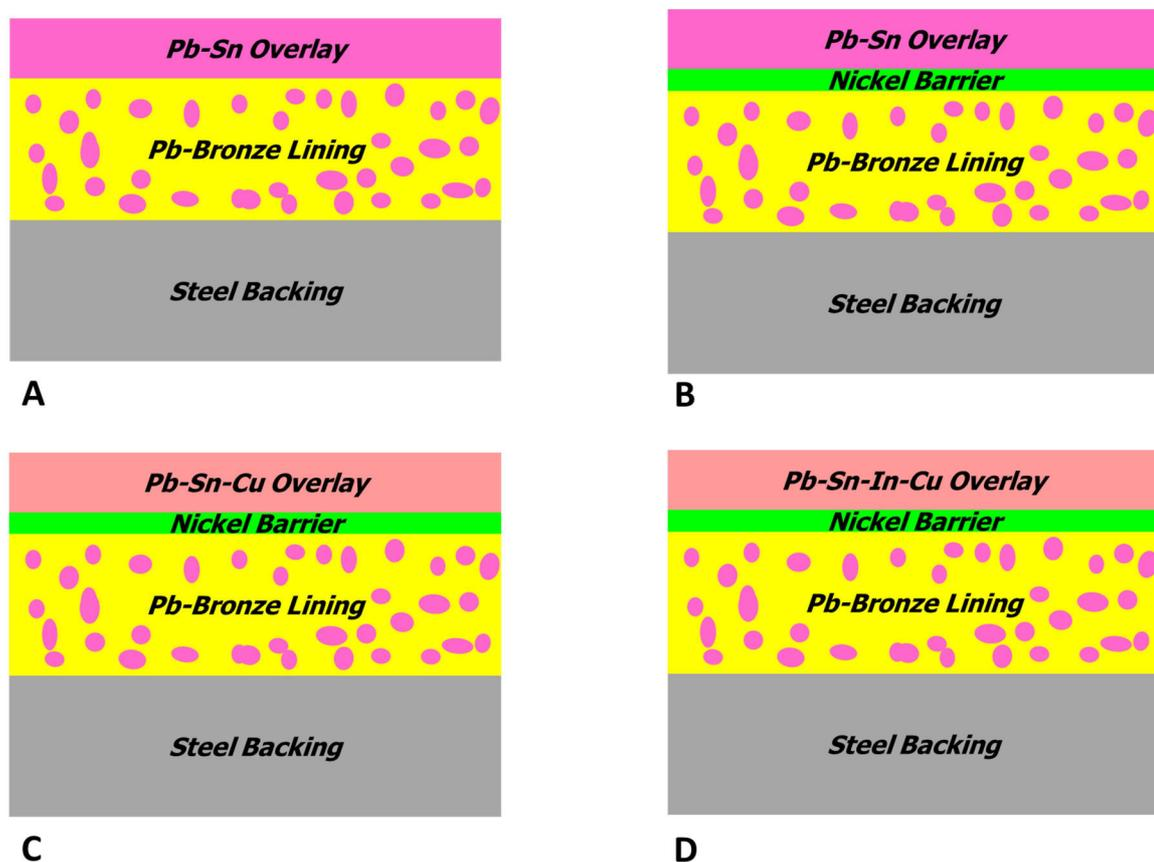
**Figure 1.6.** Evolution of Pb-based overlays electrodeposited on bronze-based bearing materials: (A) Pb-Sn overlay, (B) Pb-Sn overlay with a Ni interlayer, (C) addition of Cu to the Pb-Sn overlay, and (D) addition of In to the Pb-Sn-Cu overlay. Adapted from [3].
