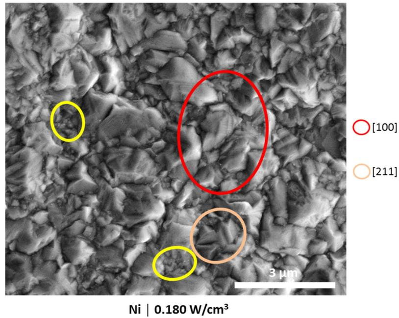
**Figure 5.27.** High magnification FIB-SEM image of the surface of a Ni coating electrodeposited under ultrasound at 0.180 W/cm<sup>3</sup>. Electrodeposition time: 14 minutes. Current density: 4 A/dm<sup>2</sup>. Some of the crystals with a surface morphology similar to that of Ni crystals with different orientations reported by other authors [19,25,27,28] are highlighted with different colours.
