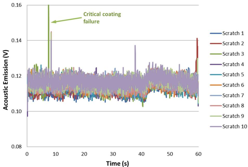
**Figure 6.17.** Acoustic emission recorded during a non-lubricated scratch test (10 continuous scratches) performed on a Ni coating electrodeposited under mechanical agitation at 300 rpm.
