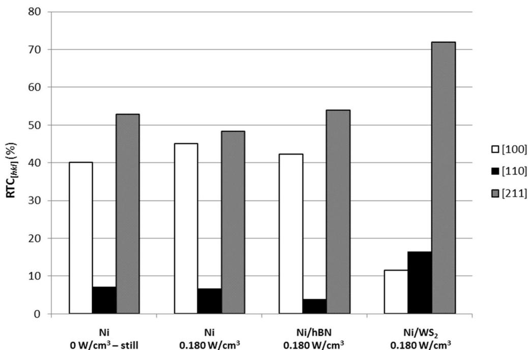
**Figure 5.23.**  $RTC_{[hkl]}$  coefficients estimated for [100], [110], and [211] Ni crystal planes observed in Ni/hBN and Ni/WS<sub>2</sub> coatings electrodeposited on Cu under ultrasound at 0.180 W/cm<sup>3</sup>.  $RTC_{[hkl]}$  coefficients corresponding to pure Ni coatings electrodeposited under either mechanical agitation at 300 rpm or ultrasound at 0.180 W/cm<sup>3</sup> are included for comparison purposes. Electrodeposition time: 14 minutes. Current density: 4 A/dm<sup>2</sup>.
