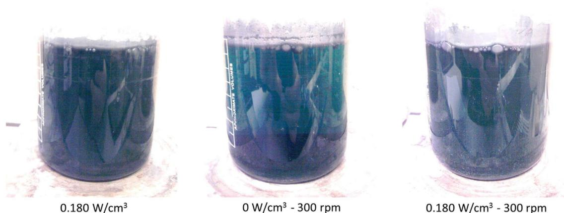
**Figure 5.2.** Appearance of Ni Watts bath + WS<sub>2</sub> dispersions (15 g/L of WS<sub>2</sub> particles) 60 minutes after dispersing the particles for 30 minutes in the electrolyte under different conditions: ultrasound at 0.180 W/cm<sup>3</sup>, mechanical agitation at 300 rpm and combined ultrasound/mechanical agitation at 0.180 W/cm<sup>3</sup> – 300 rpm.. Images were edited (50% increase in brightness) to show the quality of the dispersion.
