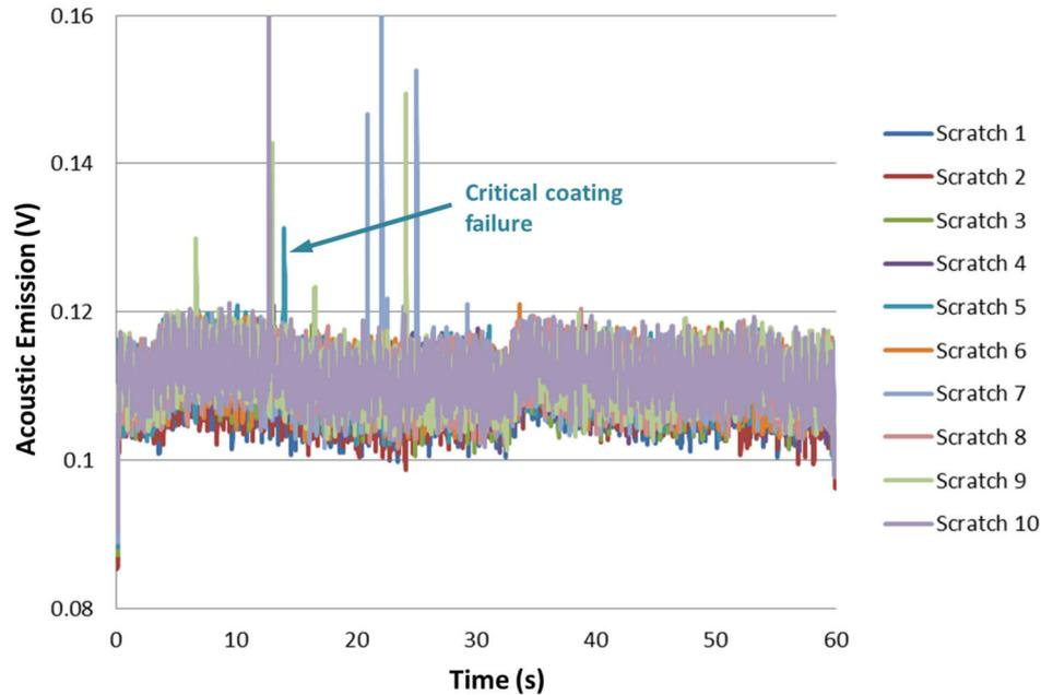
**Figure 6.23.** Acoustic emission recorded during a non-lubricated scratch test (10 continuous scratches) performed on a Ni/hBN composite coating electrodeposited under ultrasound at  $0.180 \text{ W/cm}^3$ .
