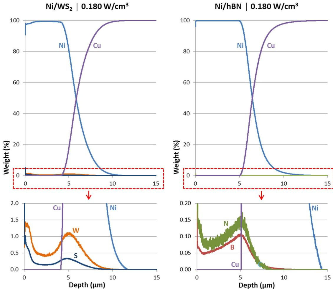
**Figure 5.19.** GD-OES depth profiles of the presence of different atoms (Ni, Cu, W, S, B, and N) in a Ni/WS<sub>2</sub> composite coating (left) and a Ni/hBN composite coating (right) electrodeposited under ultrasound at 0.180 W/cm<sup>3</sup>. Electrodeposition time: 14 minutes. Current density: 4 A/dm<sup>2</sup>. The detection of Ni far beyond the actual thickness of the coatings is due to the characteristic interface broadening generally observed in GD-OES depth profile measurements
