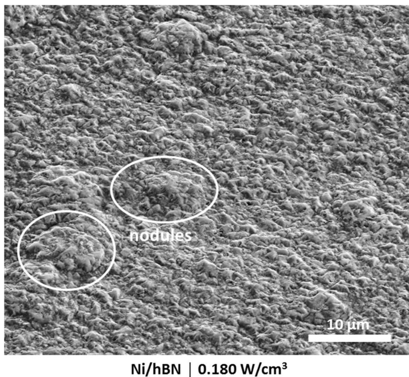
**Figure 5.26.** Tilted FIB-SEM image of the surface of a Ni/hBN composite coating electrodeposited under ultrasound at 0.180 W/cm<sup>3</sup>. Electrodeposition time: 14 minutes. Current density: 4 A/dm<sup>2</sup>.
