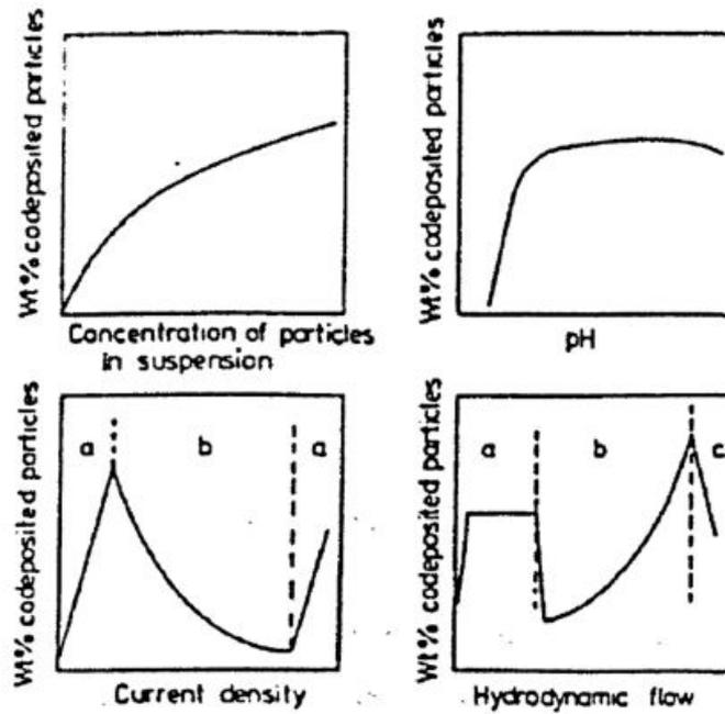
**Figure 2.2.** General effects of the concentration of particles in the electrolyte, pH, current density (a: charge transfer overvoltage, b: concentration overvoltage) and the hydrodynamic flow (a: laminar regime, b: transition zone, c: turbulent regime) on the electrodeposition of metal composite coatings with embedded particles. Adapted from Ref. [52].
