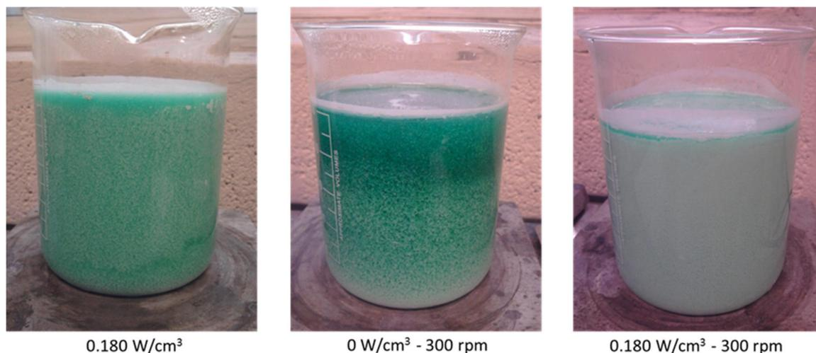
**Figure 5.5.** Appearance of Ni Watts bath + hBN dispersions (15 g/L of hBN particles) immediately after dispersing the particles for 30 minutes in the electrolyte under different conditions: ultrasound at 0.180 W/cm<sup>3</sup>, mechanical agitation at 300 rpm and combined ultrasound/mechanical agitation at 0.180 W/cm<sup>3</sup> – 300 rpm.
