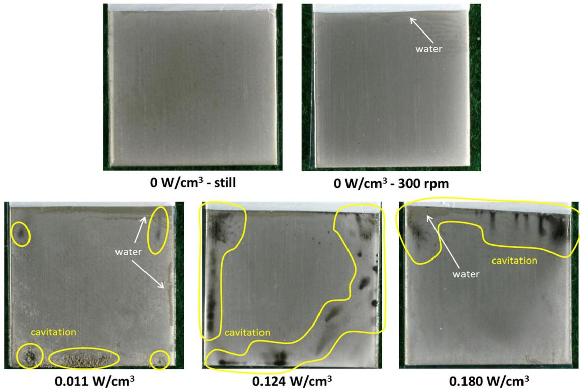
**Figure 4.1.** Examples of Ni coatings electrodeposited on Cu substrates under different conditions: silent/still, mechanical agitation at 300 rpm and ultrasonic agitation at 0.011, 0.124 and 0.180 W/cm<sup>3</sup>. Moisture (water) stains can also be seen near the edges in some of the samples. Electrodeposition time: 14 minutes. Current density: 4 A/dm<sup>2</sup>.
