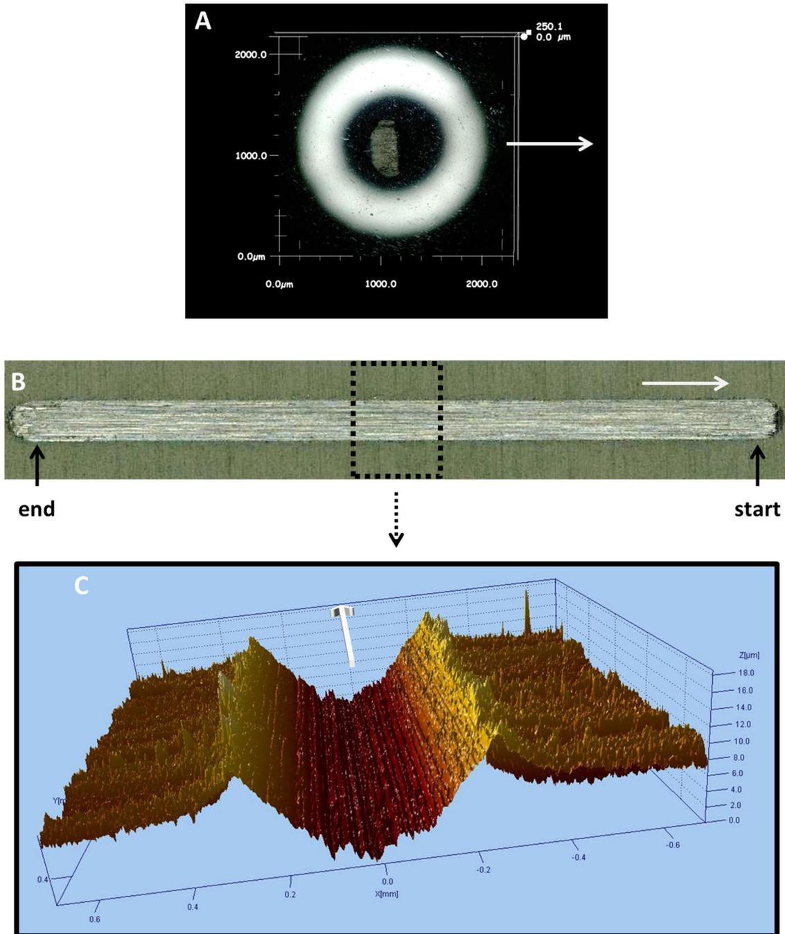
**Figure 6.9.** Images of the test ball and the wear track left by the test ball on a Ni/hBN composite coating electrodeposited under ultrasound at  $0.180 \text{ W/cm}^3$  after a lubricated scratch test: (A) test ball, (B) wear track left on the sample, (C) 3D depth profile on the middle area of the wear track left on the sample obtained by white light interferometry. The white arrows point the direction of the sample motion.
