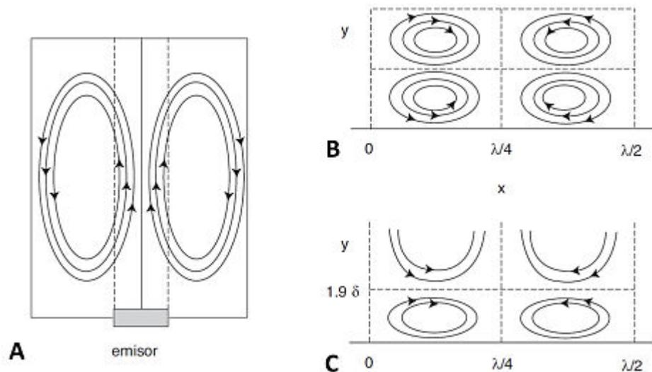
**Figure 2.6.** Acoustic streaming flow patterns in different areas: (A) bulk solution, (B) solid surface, and (C) diffusion boundary layer. Adapted from Ref. [87].
