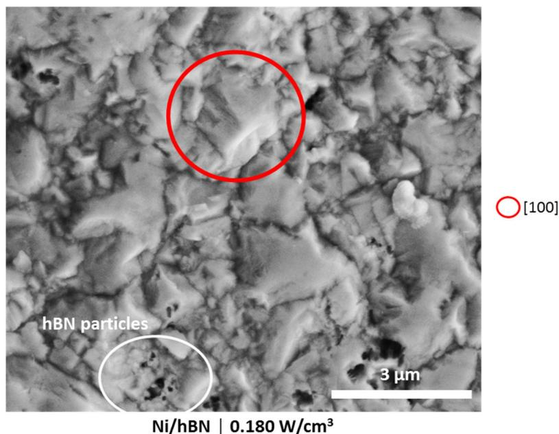
**Figure 5.29.** High magnification FIB-SEM image of the surface of a Ni/hBN composite coating electrodeposited under ultrasound at  $0.180 \text{ W/cm}^3$ . Electrodeposition time: 14 minutes. Current density:  $4 \text{ A/dm}^2$ . Some of the crystals with a surface morphology similar to that of Ni crystals with different orientations reported by other authors [19,25,27,28] are highlighted with different colours.
