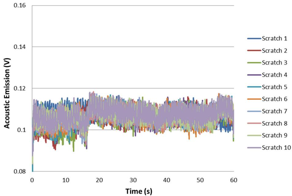
**Figure 6.11.** Acoustic emission recorded during a lubricated scratch test (10 continuous scratches) performed on a Ni/WS<sub>2</sub> composite coating electrodeposited under ultrasound at 0.180 W/cm<sup>3</sup>.
