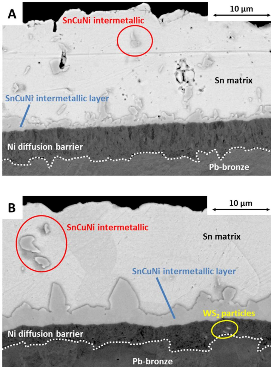
**Figure 7.6.** FEG-SEM cross-section images of samples simulating real bearing systems after 1000 hours at 130 °C. Samples consisted of a steel backing, a Pb-bronze lining deposited over the steel backing, a Ni-based diffusion barrier layer (either a Ni deposit produced under mechanical agitation or a Ni/WS<sub>2</sub> composites electrodeposited under ultrasound) over the lining, and an electroplated Sn-Cu overlay on top.
