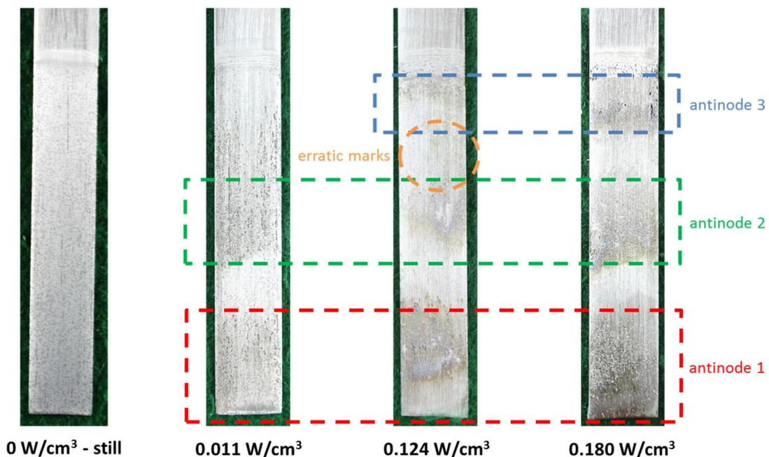
**Figure 4.2.** Final appearance of the Ni anodes for plating experiments (around 360 minutes) at different ultrasonic powers.
