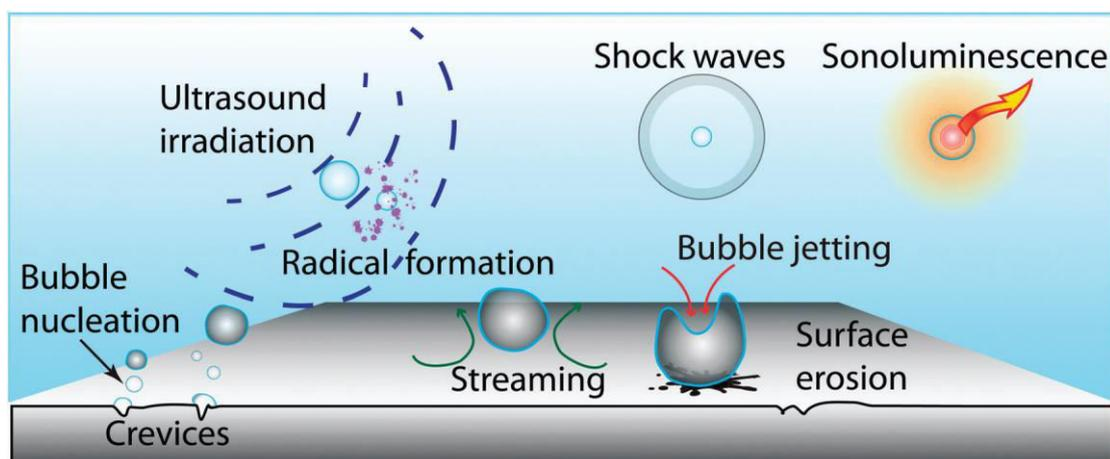
**Figure 2.5.** Schematic representation of the main effects of cavitation induced by ultrasound irradiation. Adapted from Ref. [64].
