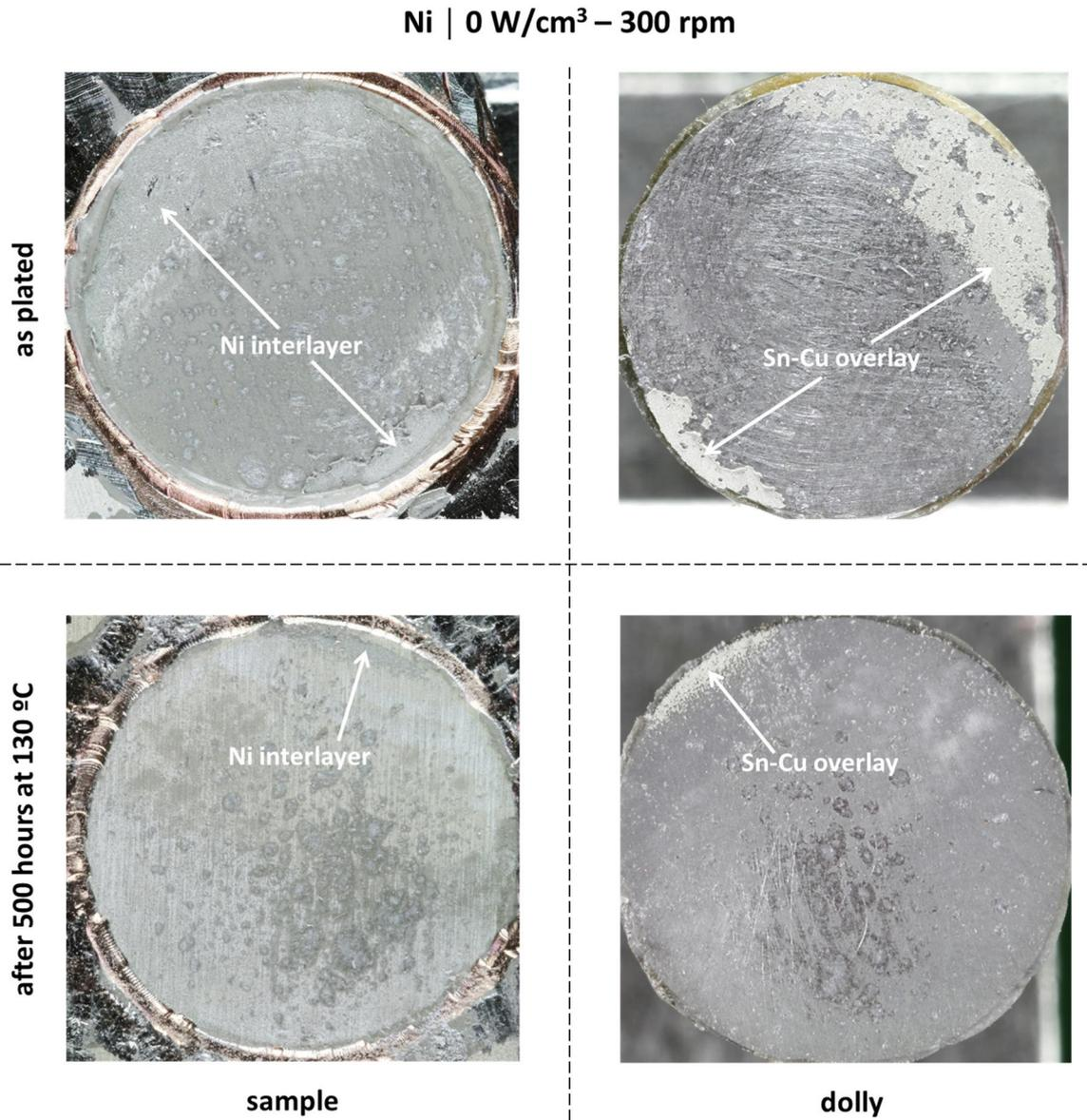
**Figure 7.2.** Images of the surface of samples and dollies after bonding tests performed on samples simulating real bearing systems consisting of a steel backing, a Pb-bronze lining deposited over the steel backing, a Ni diffusion barrier layer electrodeposited over the lining under mechanical agitation at 300 rpm, and an electroplated Sn-Cu overlay on top.
