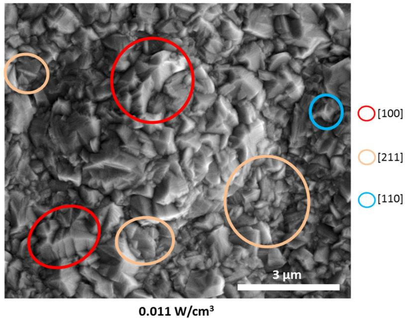
**Figure 4.14.** High magnification FIB-SEM images of the surface of Ni electrodeposited under ultrasound at 0.011 W/cm<sup>3</sup>. Electrodeposition time: 14 minutes. Current density: 4 A/dm<sup>2</sup>. Some of the crystals with a surface
