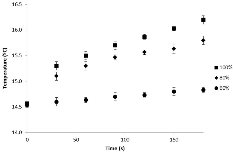
**Figure A.1.** Evolution of  $T$  vs.  $t$  time in 0.5 l of deionised water contained in a 0.6 l beaker containing submersed in an Ultrawave QS12 ultrasonic bath.
