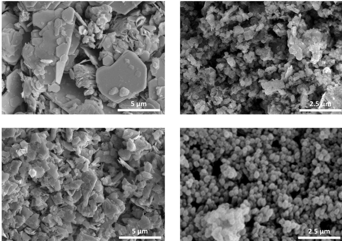
**Figure 3.3.** SEM images of the different lubricant particles used in the present research project: A)  $\text{WS}_2$ , B) hBN, C)  $\text{MoS}_2$  and D) PTFE.
