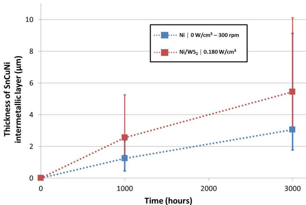
**Figure 7.8.** Thickness of the SnCuNi intermetallic layer vs. heat-treatment time for samples simulating real bearing systems. Samples consisted of a steel backing, a Pb-bronze lining deposited over the steel backing, a Ni-based diffusion barrier layer (either a Ni deposit produced under mechanical agitation or a Ni/WS<sub>2</sub> composites electrodeposited under ultrasound) over the lining, and an electroplated Sn-Cu overlay on top.
