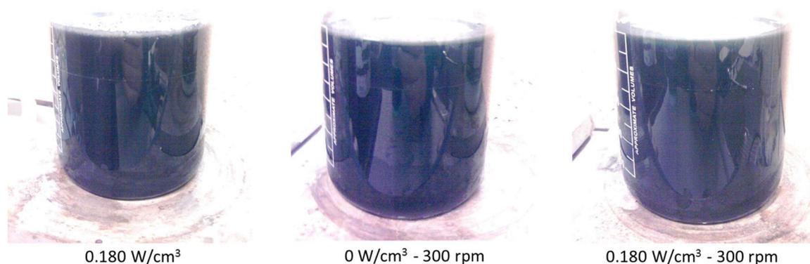
**Figure 5.8.** Appearance of Ni Watts bath + MoS<sub>2</sub> dispersions (15 g/L of MoS<sub>2</sub> particles) immediately after dispersing the particles for 30 minutes in the electrolyte under different conditions: ultrasound at 0.180 W/cm<sup>3</sup>, mechanical agitation at 300 rpm and combined ultrasound/mechanical agitation at 0.180 W/cm<sup>3</sup> – 300 rpm. Images were edited (50% increase in brightness) to show the quality of the dispersion.
