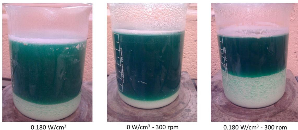
**Figure 5.6.** Appearance of Ni Watts bath + hBN dispersions (15 g/L of hBN particles) 30 minutes after dispersing the particles for 30 minutes in the electrolyte under different conditions: ultrasound at  $0.180 \text{ W/cm}^3$ , mechanical agitation at 300 rpm and combined ultrasound/mechanical agitation at  $0.180 \text{ W/cm}^3 - 300 \text{ rpm}$ .
