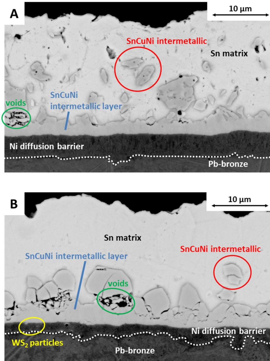
**Figure 7.7.** FEG-SEM cross-section images of samples simulating real bearing systems after 3000 hours at 130 °C. Samples consisted of a steel backing, a Pb-bronze lining deposited over the steel backing, a Ni-based diffusion barrier layer (either a Ni deposit produced under mechanical agitation or a Ni/WS<sub>2</sub> composites electrodeposited under ultrasound) over the lining, and an electroplated Sn-Cu overlay on top.
