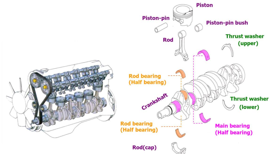
**Figure 1.1.** Diagram of an automotive engine showing different types of bearings. Adapted from [5].
