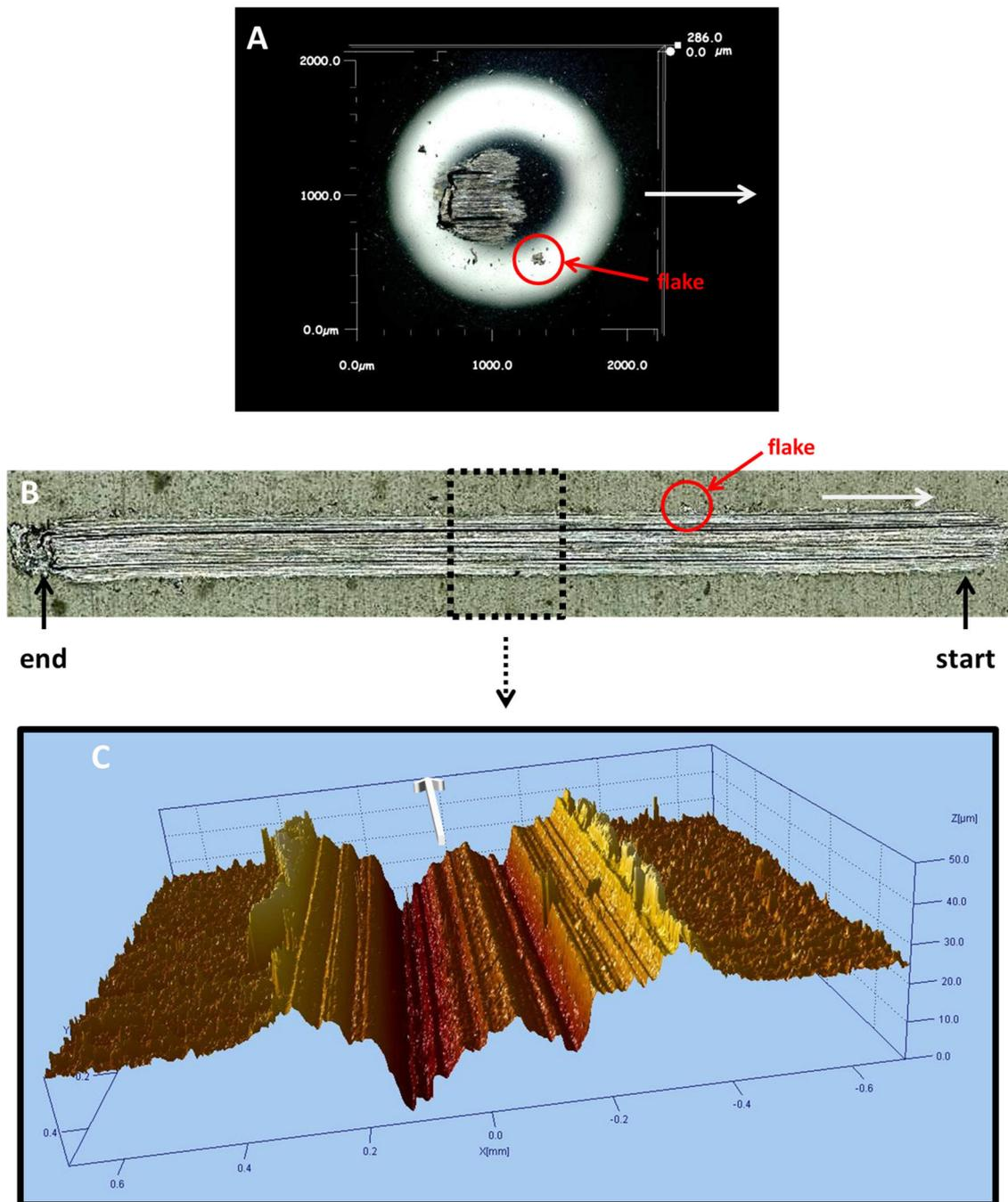
**Figure 6.18.** Images of the test ball and the wear track left by the test ball on a Ni coating electrodeposited under mechanical agitation at 300 rpm after a non-lubricated scratch test: (A) test ball, (B) wear track left on the sample, (C) 3D depth profile on the middle area of the wear track left on the sample obtained by white light interferometry. The white arrows point the direction of the sample motion.
