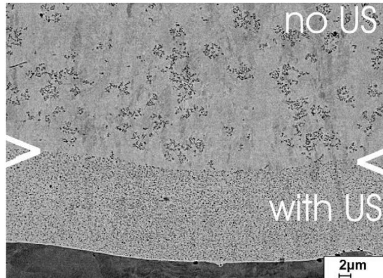
**Figure 2.8.** Well-dispersed particles under ultrasound conditions (lower part from substrate up to the markers ><) and nano-particle agglomeration under silent conditions (upper part). Adapted from Ref. [97].
