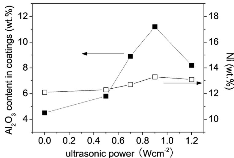
**Figure 2.11.** Influence of ultrasonic power on the nano-alumina contents in Zn-Ni/ $\text{Al}_2\text{O}_3$  nanocomposite coatings and Ni contents in the Zn-Ni matrix of composite coatings. Adapted from Ref. [122].
