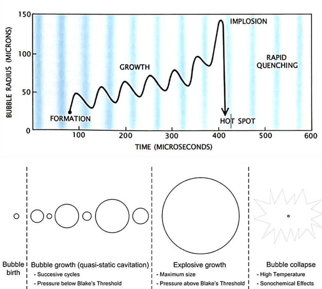
**Figure 2.4.** Bubble growth and implosion in a liquid irradiated with ultrasound. Large alternating stresses within the irradiated liquid form by setting an ultrasonic field which generates positive (blue colour in upper image) and negative (white colour in upper image) pressure areas. Adapted from Refs. [59] and [60].
