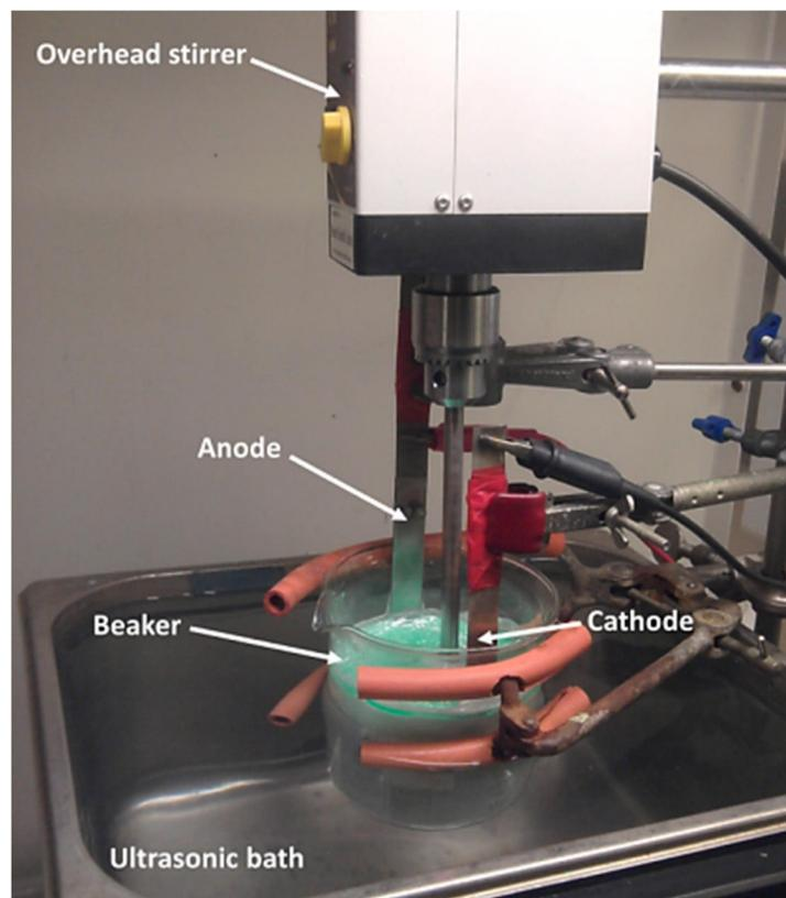
**Figure 3.1.** Experimental set-up for small scale electroplating experiments.
