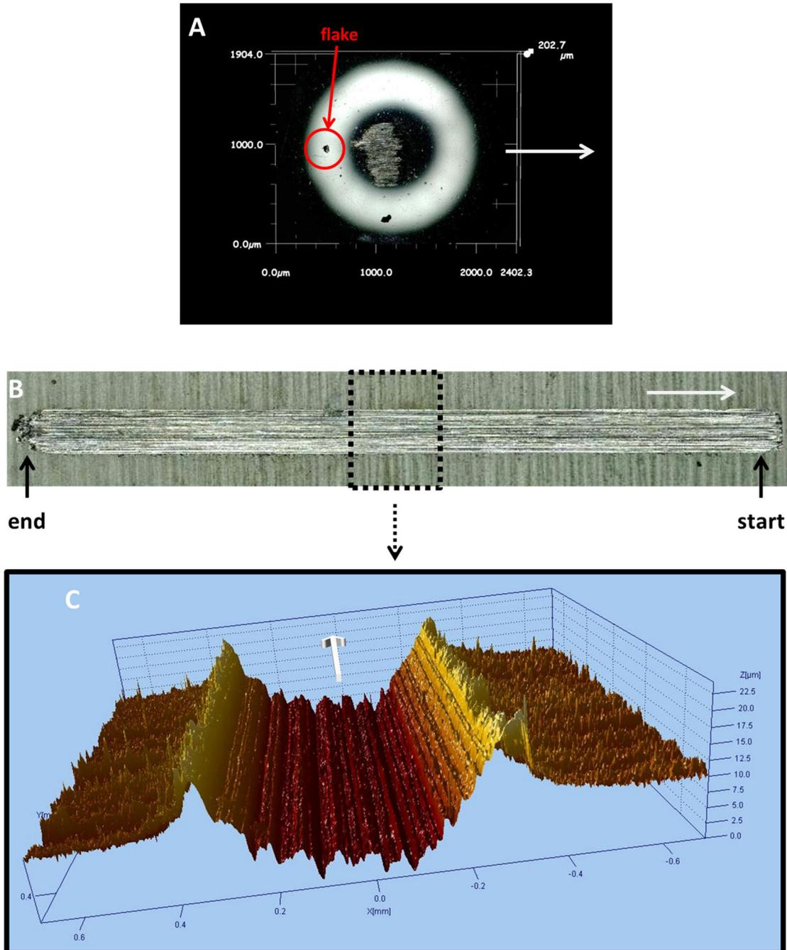
**Figure 6.27.** Images of the test ball and the wear track left by the test ball on a Ni/WS<sub>2</sub> composite coating electrodeposited under ultrasound at 0.180 W/cm<sup>3</sup> after a lubricated scratch test: (A) test ball, (B) wear track left on the sample, (C) 3D depth profile on the middle area of the wear track left on the sample obtained by white light interferometry. The white arrows point the direction of the sample motion.
