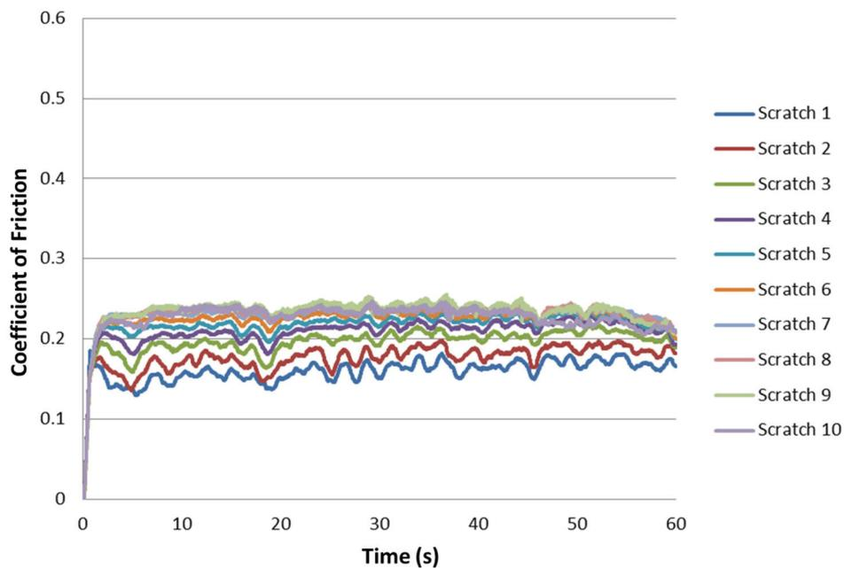
**Figure 6.10.** CoF measured during a lubricated scratch test (10 continuous scratches) performed on a Ni/WS<sub>2</sub> composite coating electrodeposited under ultrasound at 0.180 W/cm<sup>3</sup>.
