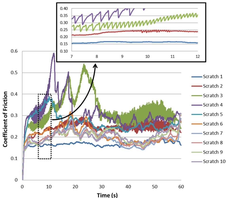
**Figure 6.19.** CoF measured during a non-lubricated scratch test (10 continuous scratches) performed on a Ni coating electrodeposited under ultrasound at  $0.180 \text{ W/cm}^3$ . Zoomed-in graph shows when stick-slip friction started to occur (only scratches 1 to 4 are shown for better visibility).
