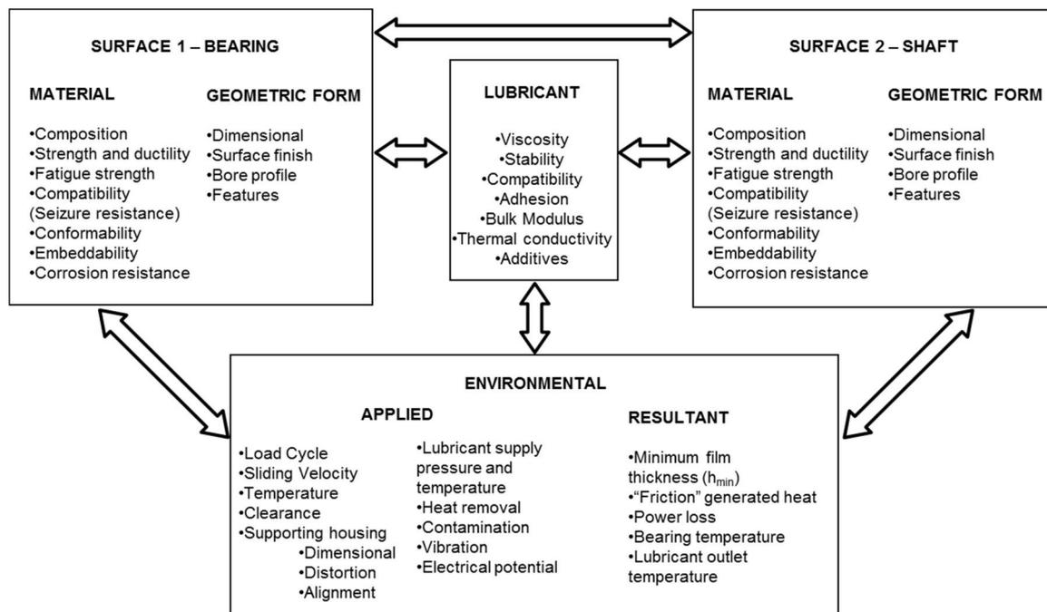
Figure 1.2. Interactions between components and environment in a bearing system. Adapted from [6].
