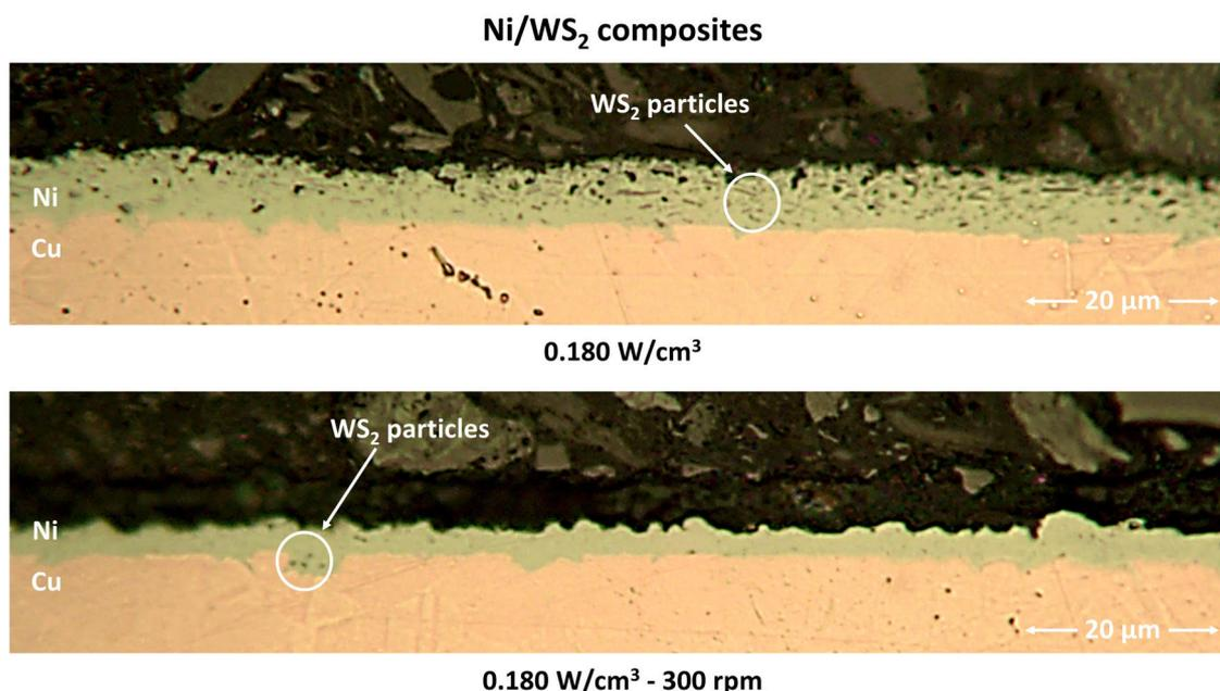
**Figure 5.12.** Examples of cross-section images of Ni/WS<sub>2</sub> composite coatings electrodeposited on Cu substrates under different plating conditions: ultrasound at  $0.180 \text{ W/cm}^3$ , mechanical agitation at  $300 \text{ rpm}$  and combined ultrasound/mechanical agitation at  $0.180 \text{ W/cm}^3 - 300 \text{ rpm}$ . Electrodeposition time: 14 minutes. Current density:  $4 \text{ A/dm}^2$ .
