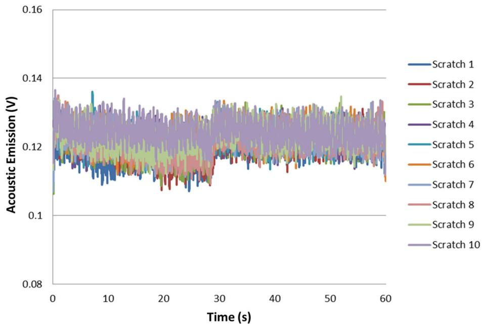
**Figure 6.26.** Acoustic emission recorded during a non-lubricated scratch test (10 continuous scratches) performed on a Ni/WS<sub>2</sub> composite coating electrodeposited under ultrasound at 0.180 W/cm<sup>3</sup>.
