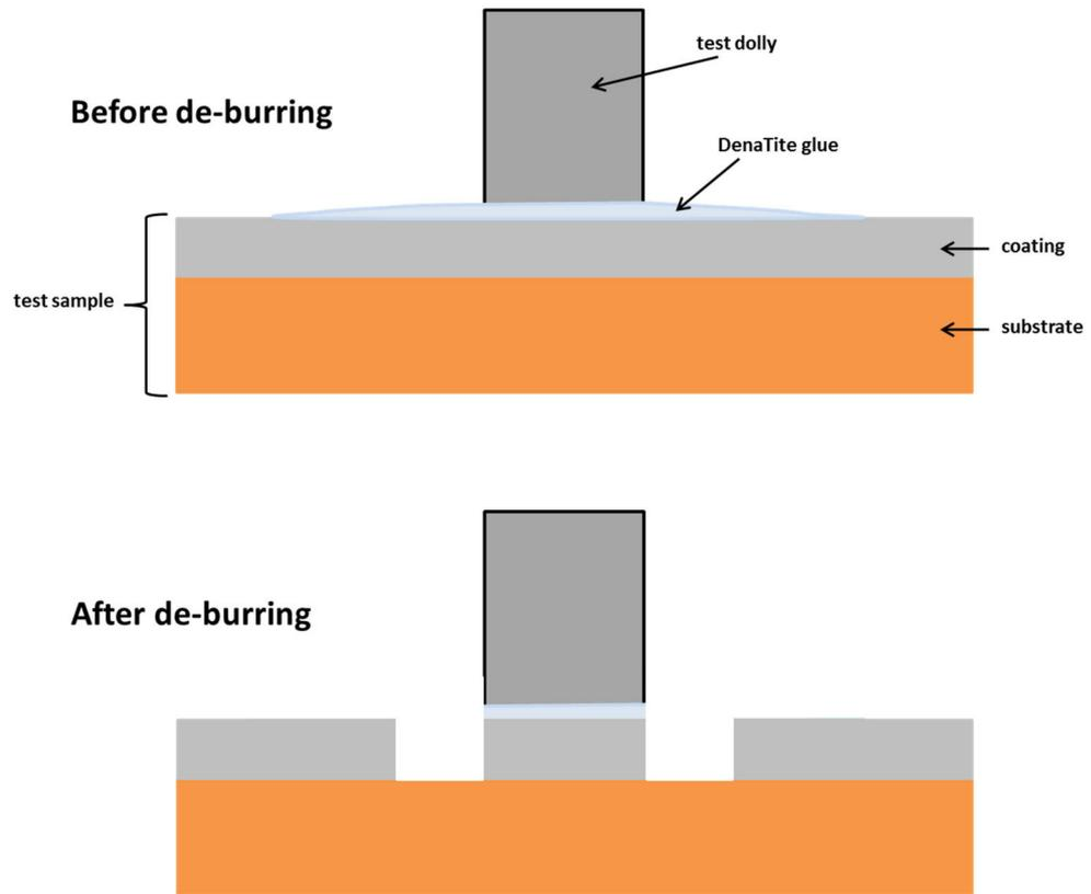
**Figure D.3.** Diagram showing the cross-section of a assembled test sample and dolly before and after de-burring once the DenaTite glue is cured.
