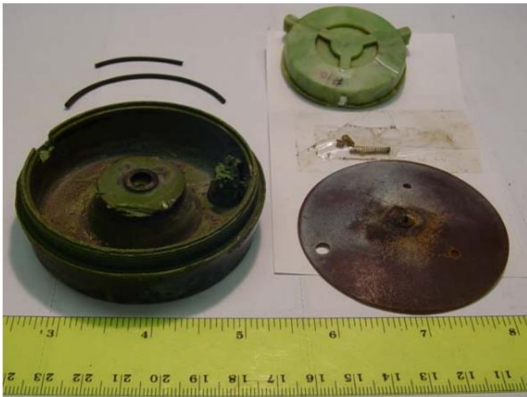
Figure 20 Type72A disassembled (United States Department of State and Office of Weapons Removal and Abatement, 2009)
