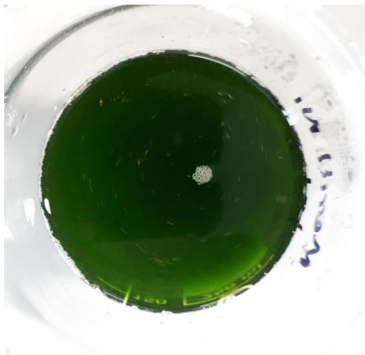
Figure 6.4. Image of the surface beaker containing LICE nickel electrolyte with 10.0 g/l of Tween 20 and 1.0 g/l of turmeric.
