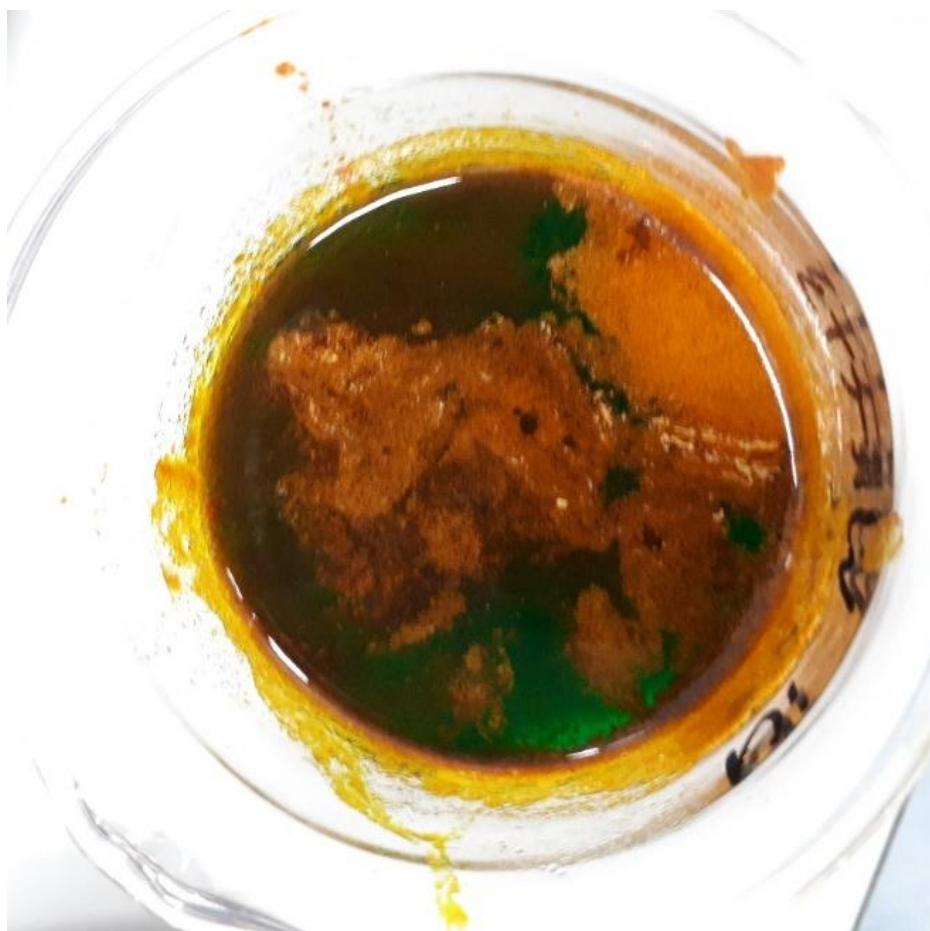
Figure 6.1. Image of the surface of the nickel Watts electrolyte with 10.0 g/l of Tween 20 and 1.0 g/l of turmeric.
