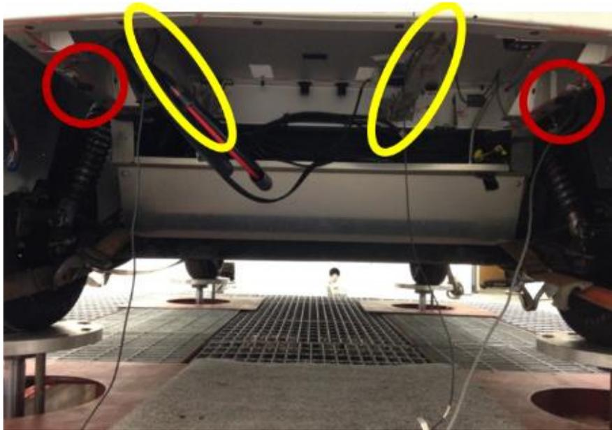
**Figure 8-7 - Chassis Mounted Accelerometers**
