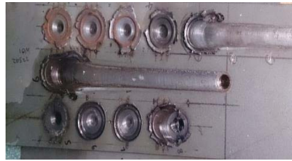
Figure 1: Representation of the positioning of the seven plunge trials for EH46 steel plates.
