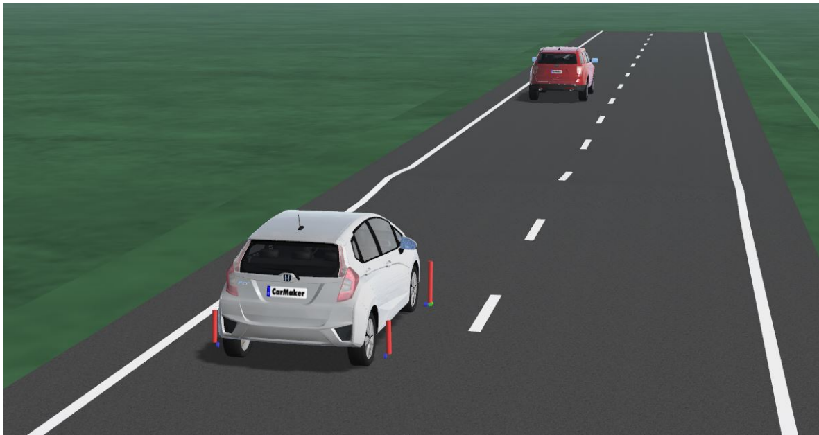
Figure 6. Performance evaluation scenario including ego, target vehicle and a road bump obstacle.
