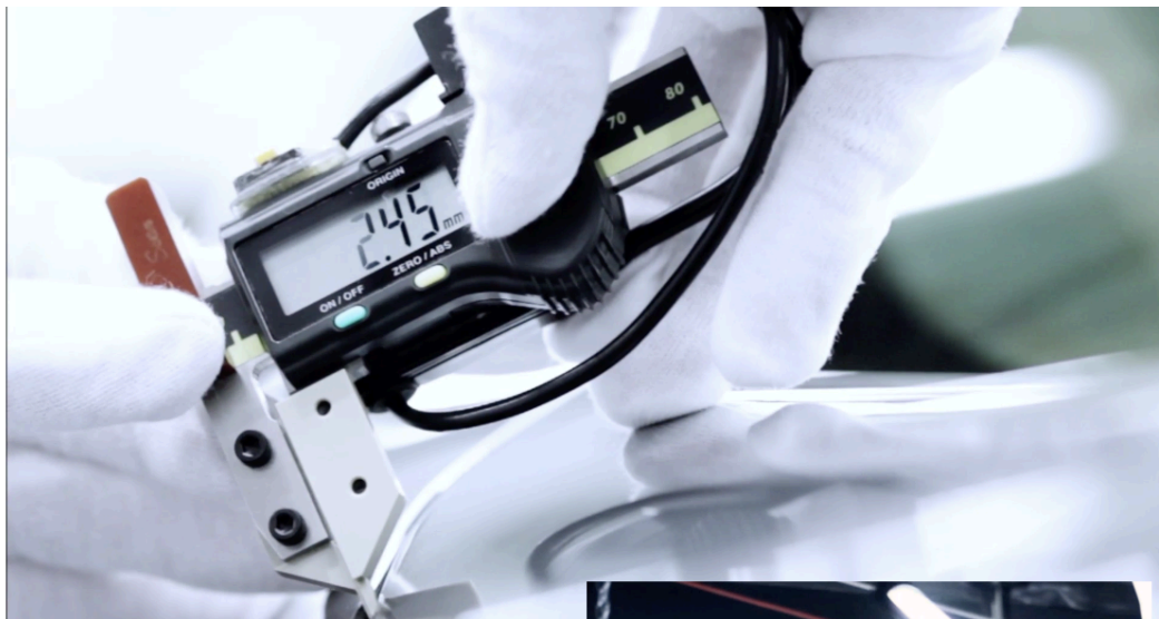
Fig. 2.9 Measuring panel gaps with digital gap gauge calliper (Lexus UK 2019).
