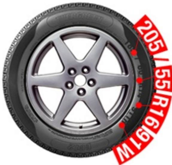
Fig. 5.11. Wheel and tyre sizes (Black Circles 2018)
