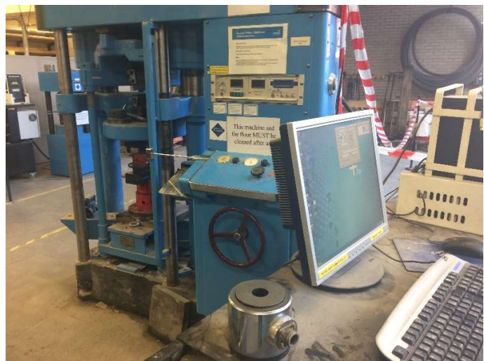
Figure 5.8: Avery Denison 2000 machine linked to a computer
