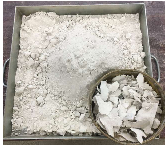
Figure 5.3: Sieving of plasterboard to remove paper
