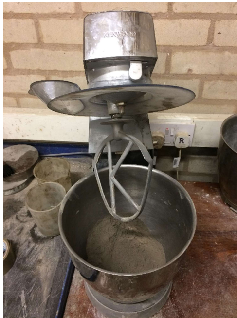
Figure 5.4: KENWOOD machine with sample in the bowl ready to be mixed
