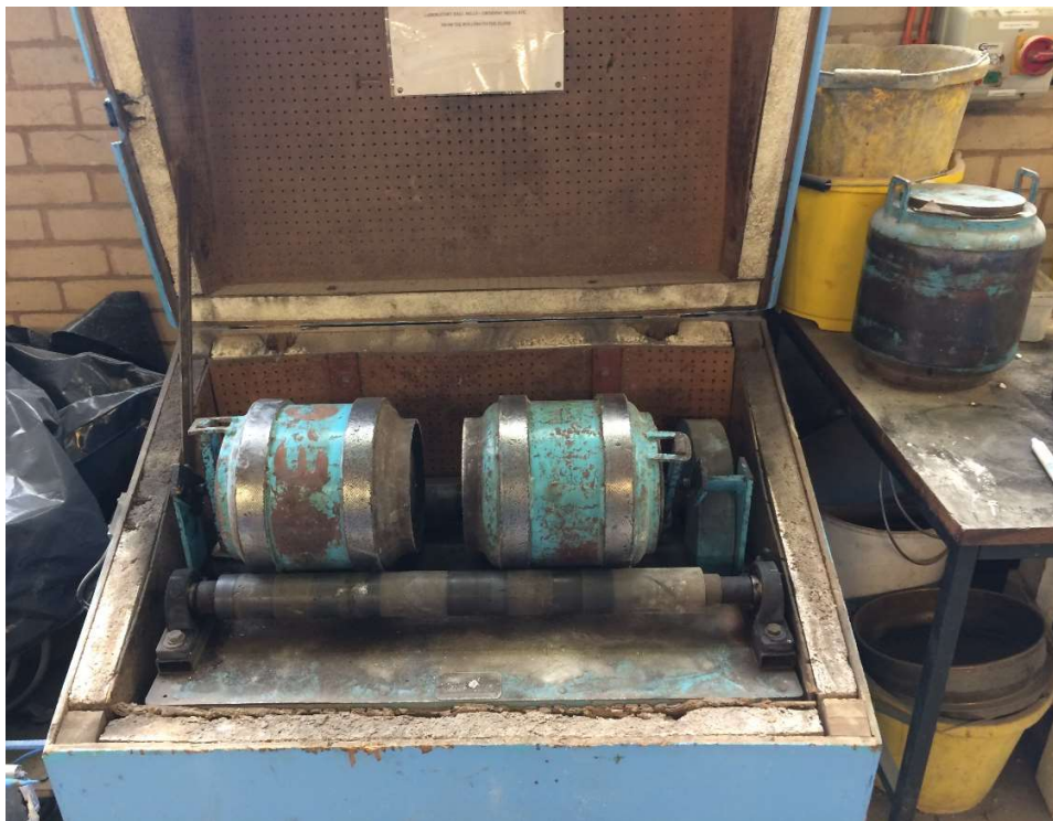
Figure 5.1: Ball Milling Machine
