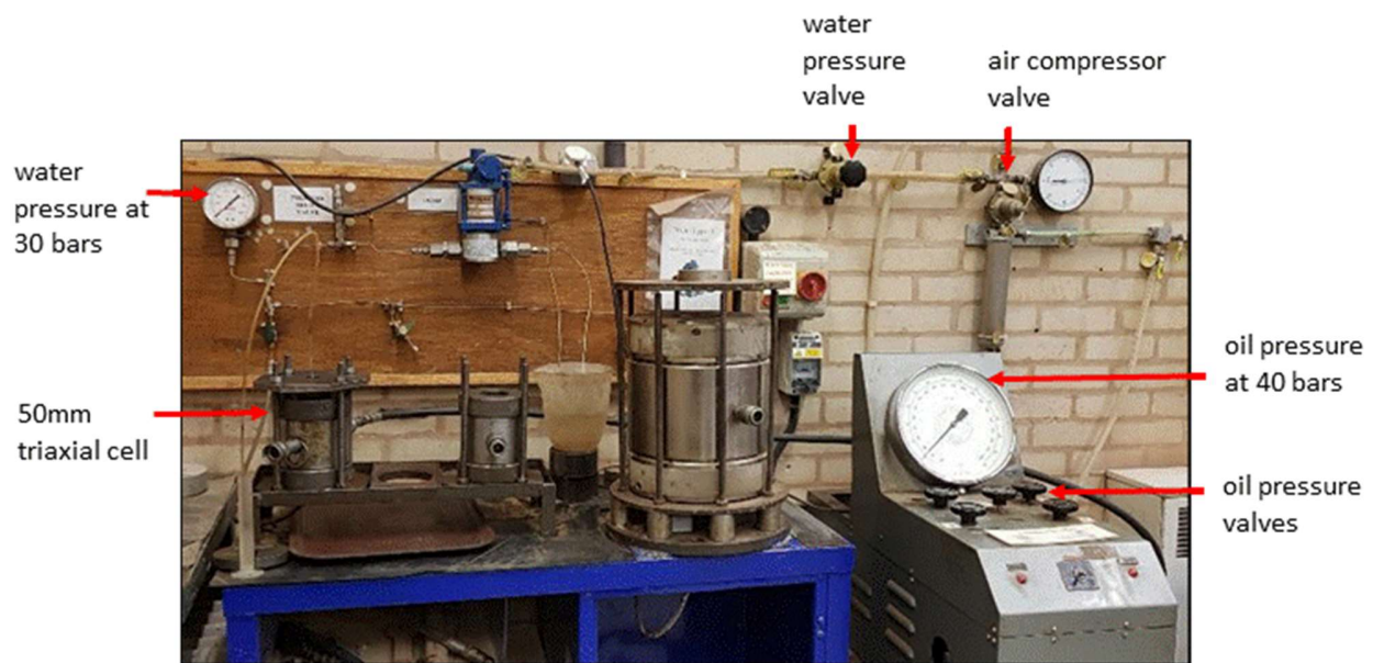
Figure 8.1: High Pressure Flow Test Layout
