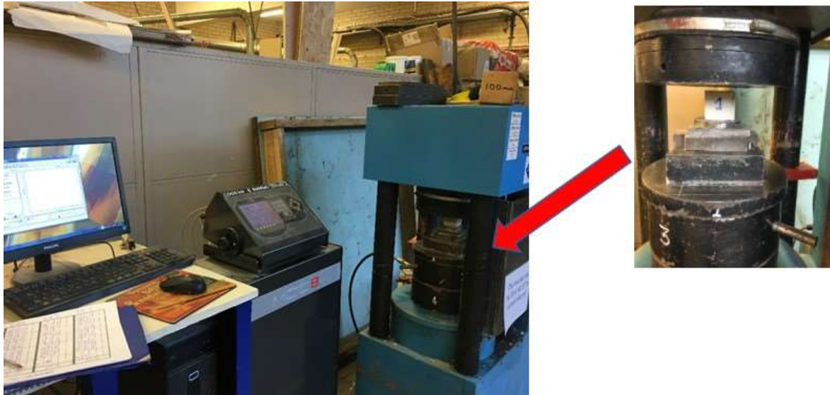
Figure 5.12: Avery Denison 2000 machine linked to a computer
