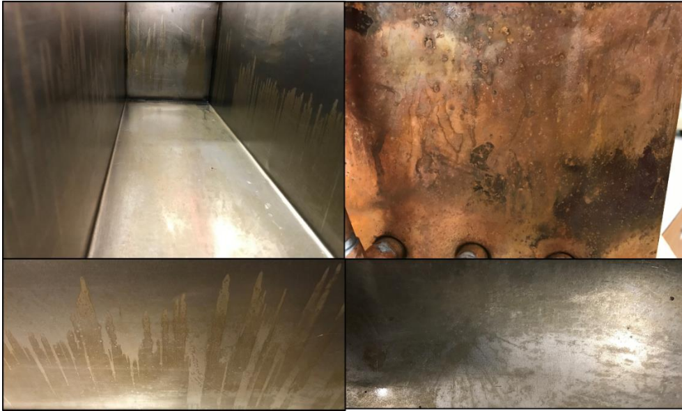
Figure 5-20: Pitting on the surface of the mild steel container and copper fins
