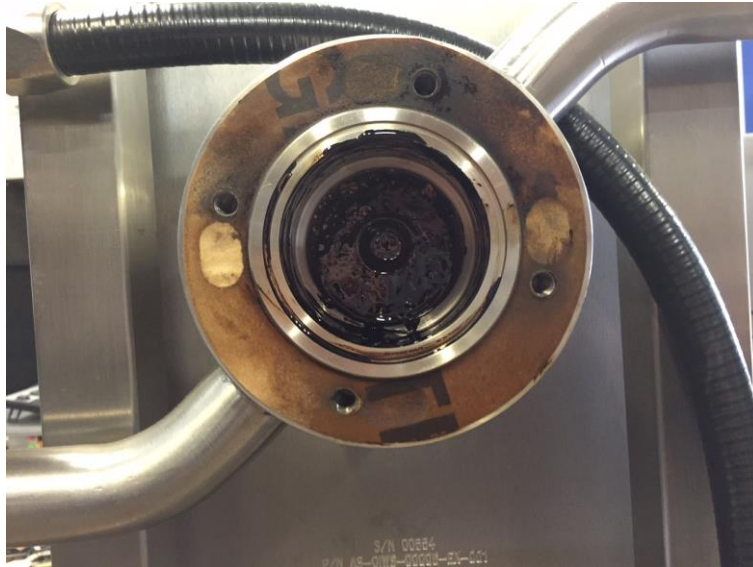
Figure 4.30 – Manual Fouling on LIF Bypass Device
