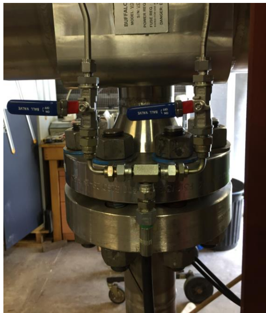
Figure 4.7 – Inline Image Analysis: Cleaning Mechanism Arrangement
