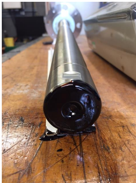
Figure 4.29 – Manual Fouling on Inline LIF
