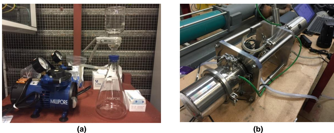
Figure 3.8 – (a) Filtration Based Solids in Water Analysis (b) Malvern Insittec Particle Size Analyser
