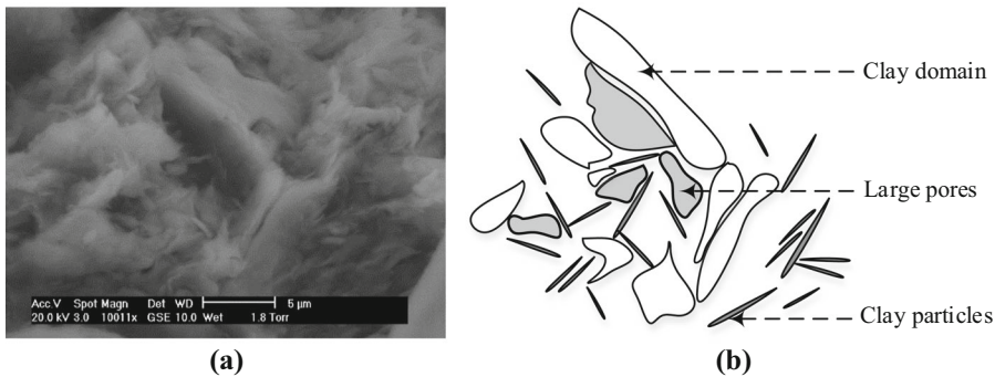
Fig. 6 ESEM micrograph: a soil fabric, b schematic diagram of particles and domains arrangements and presence of large pores in flocculated soil fabric
