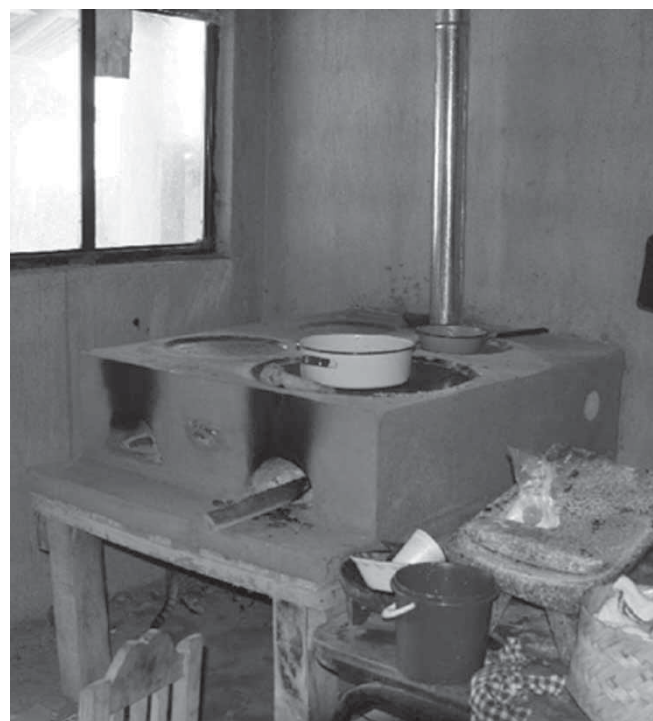
FIGURE 3 A Patsari wood-burning stove. The stove has a closed combustion chamber surrounded by bricks. A flat pottery dish or metal hotplate (called a comal and used for cooking tortillas) is integrally built into the surface of the stove, which has a smaller entrance for feeding fuel and a flue that passes through the roof and conveys the smoke outdoors. Reproduced from [92] with permission.
