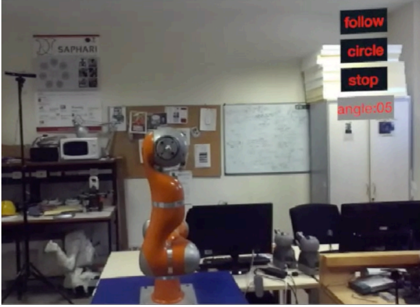
Figure 4: The mixed reality user interface on the Rift HMD screen lenses.
