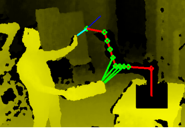
Figure 8: Snapshot of a depth image superposed with the computed distances between control points (green circles) on the robot arm and close objects located in the surveillance area. The picture shows also the computed distance between the end-effector and the human hand obstacle (cyan line), as well as its associated repulsive vector (blue line).
