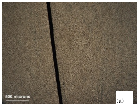
Figure 3-24 Optical micrographs of crack path when the crack propagates in (a) the substrate of Wall-Bi120 and (b) the WAAM made material
