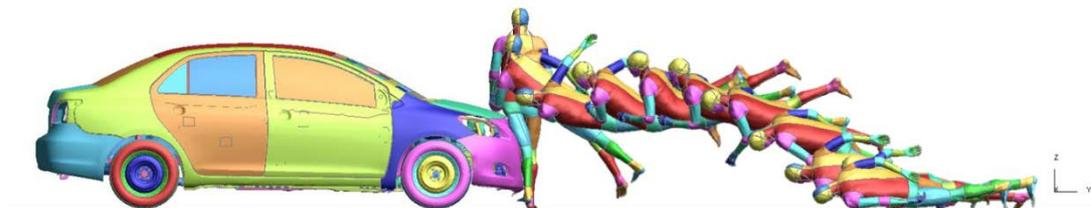
Figure 1: Typical pedestrian kinematics during collision with braking
