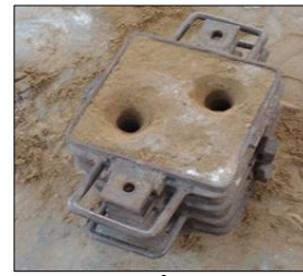
Fig. 8: CO 2 sand mould
