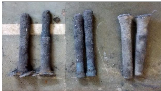
Fig. 10: As – cast specimen (from left) in green sand mold, dry sand mold and CO 2 mold
