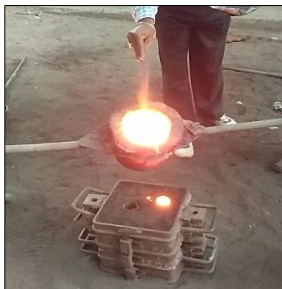
Fig. 3: Fe-Si alloy addition
