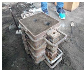
Fig. 6: Green sand mould
