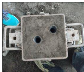
Fig. 7: Dry sand mould
