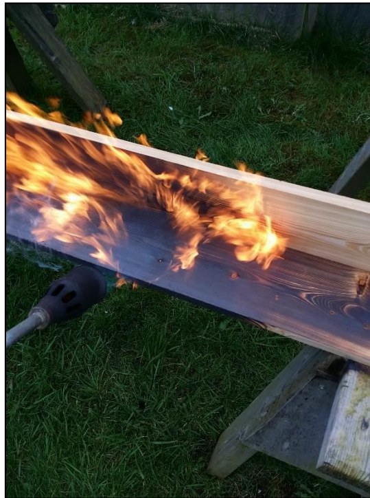
Figure 29 Charring with propane torch
