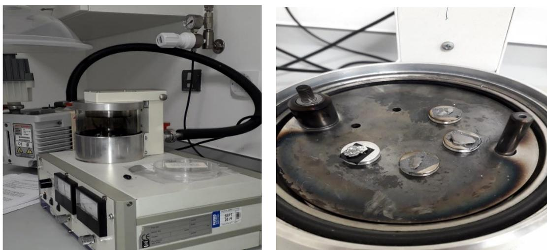
Figure 3.6 Sample preparation for SEM analysis using the sputter coater
