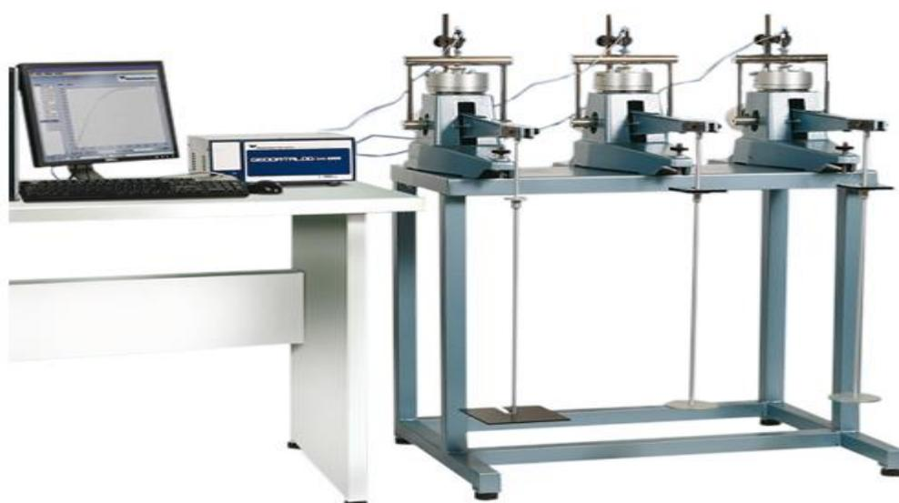
Figure 3.4 Automated oedometer used in the laboratory
