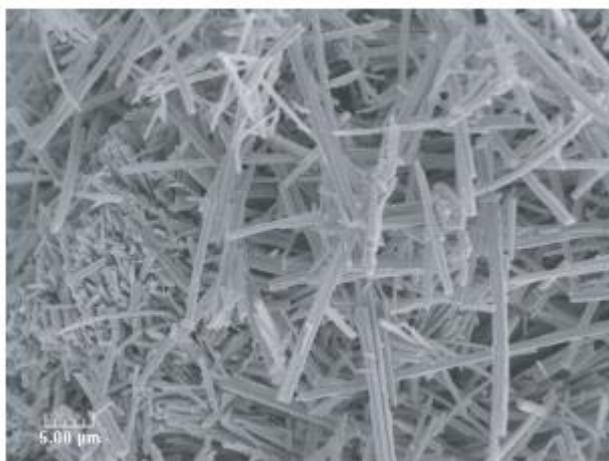
Figure 2.15 SEM showing the growth of needle-shaped crystals (modified after Nair and Little (2011))
