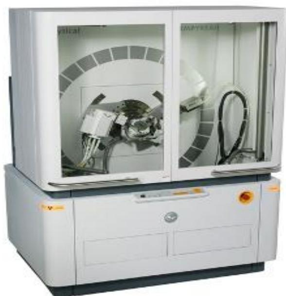
Figure 3.8 X-ray diffraction equipment.
