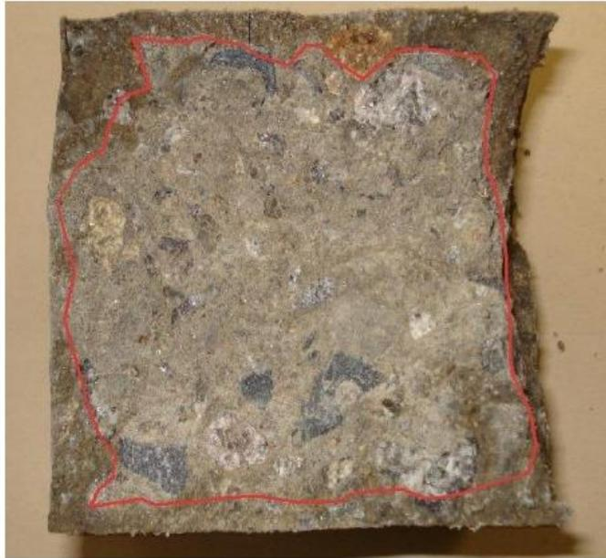
Figure 2.20 Impenetrable soil resulting from modification by RoadCEM (modified after Marjanovic et al. (2009))
