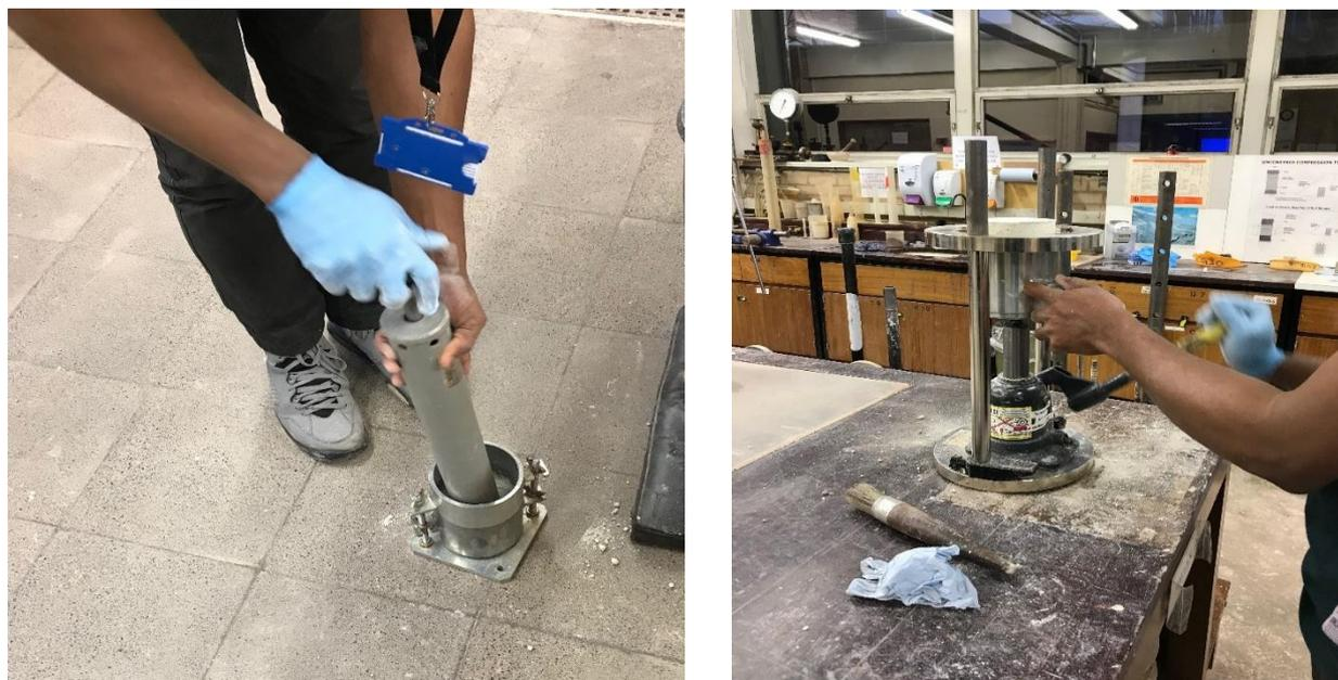
Figure 3.3 Laboratory standard proctor compaction and sample extraction from mould
