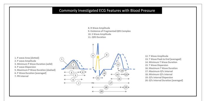
FIGURE 2 | The graphical definition of common ECG wave features seen in this review of 35 articles. QT intervals in numbers 8 to 11 are corrected for heart rate into QTc intervals by applying a formula such as Bazett's (QTc =  $QT/\sqrt{RR}$  interval) (11) or Hodge's formula [QTc = QT + 1.75 (heart rate – 60)] (12). Note that the two ECG signal segments (solid and dashed) are collected from the same subject.
