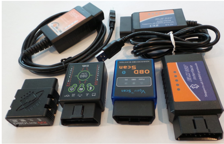
Fig. 4.1 Examples of wired and wireless ELM OBD dongles, used to read and write data via a vehicle's CAN bus
