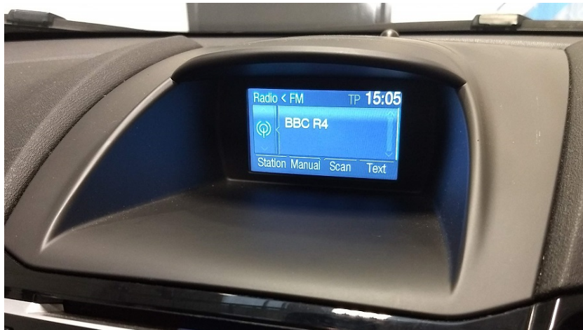
Fig. 9.1 The display ECU in the laboratory vehicle, a variety of messages are displayed in response to occupants operating the vehicle
