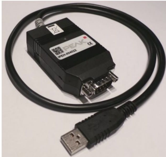
Fig. 5.3 The PEAK-System USB (PC) to CAN interface device used during the development and use of the fuzzer
