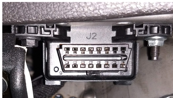
Fig. 2.6 An OBD port in a vehicle
