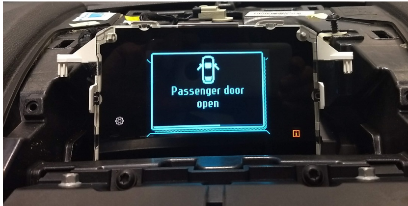
Fig. 9.8 The bench ToE display ECU in the laboratory vehicle, the obtained display ECU is a lower specification component than the one fitted to the lab car, however, it functions correctly (the correct vehicle model and year was used to order the bench ToE, but after removing the vehicle's display ECU it was seen that the twelve character part numbers differed in the last two characters)
