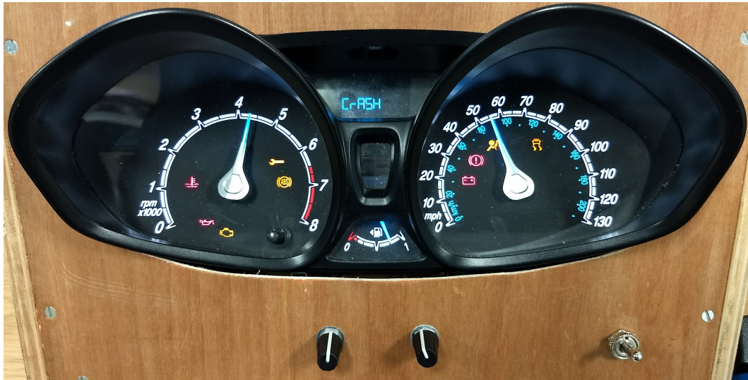
Fig. 6.1 Crashing a vehicle component as a result of fuzzing, the word CrASH appeared in the middle of the display during the fuzz testing and would not clear on a power cycle, unlike the other warning lights
