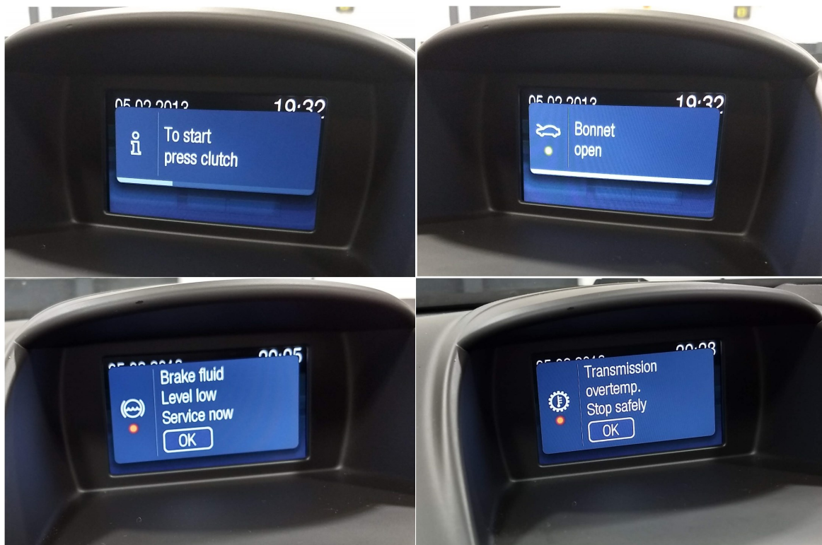
Fig. 9.20 CAN packets discovered from the fuzz testing are injected into the lab vehicle's internal network, note that the lab vehicle required the brake to be pressed to start, the bonnet was closed, the brake fluid level was not low, and the car had not been used as was therefore cold
