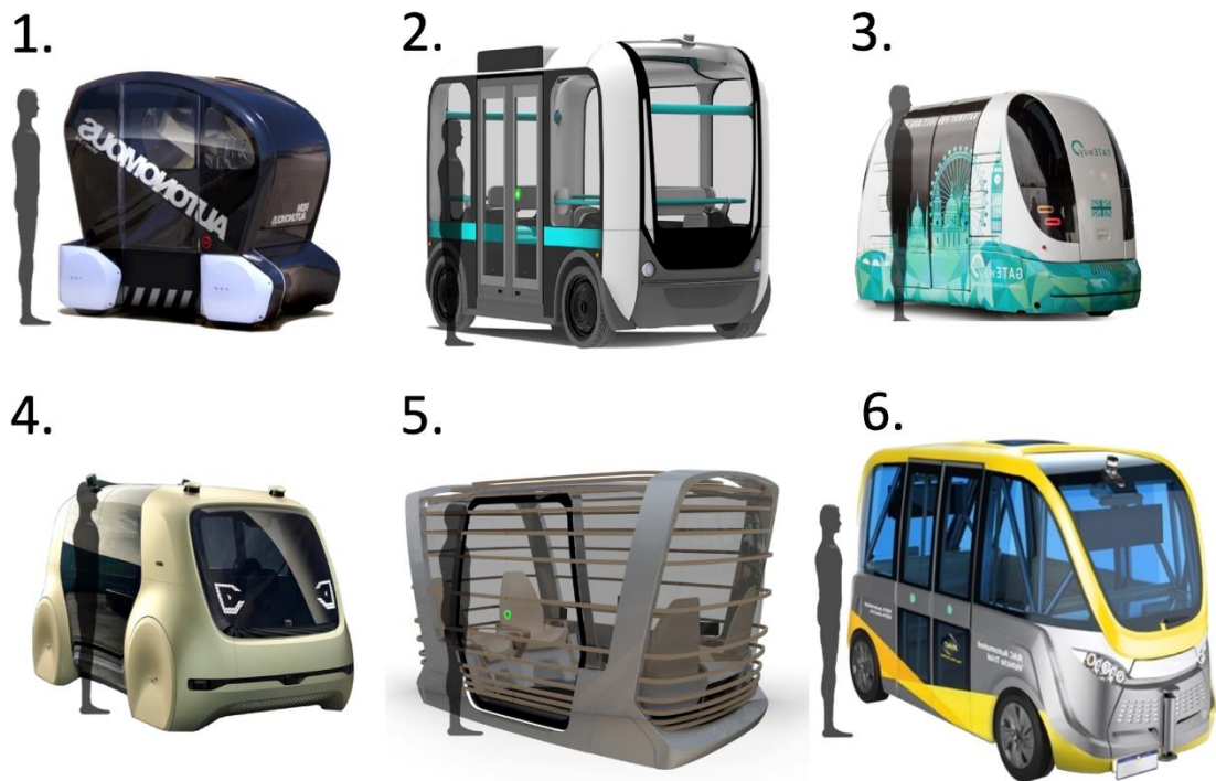
Figure 9.2. Six driverless first and last mile mobility vehicles included in the exterior design review. (1. RDM POD Zero, 2. Olli Local Motors, 3. ULTra Global PRT, 4. SEDRIC VW, 5. MiCar, 6. Navya Arma)
