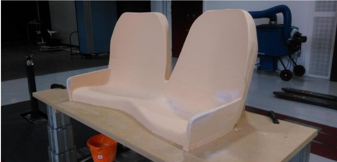
Figure 11.6 (Bench Seat milled out of High-Density Foam)
