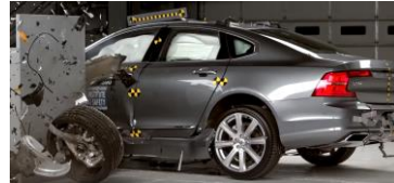
(d) 2017 Volvo S90 small overlap impact test
