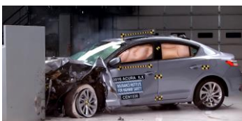
(a) 2016 Acura ILX small overlap impact test
