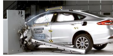
(c) 2017 Ford Fusion small overlap impact test
