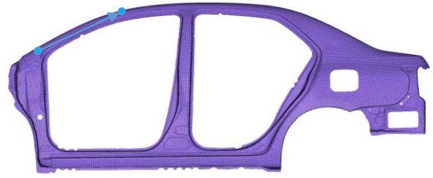
Figure 12. Locations for measuring A-pillar deformation.
