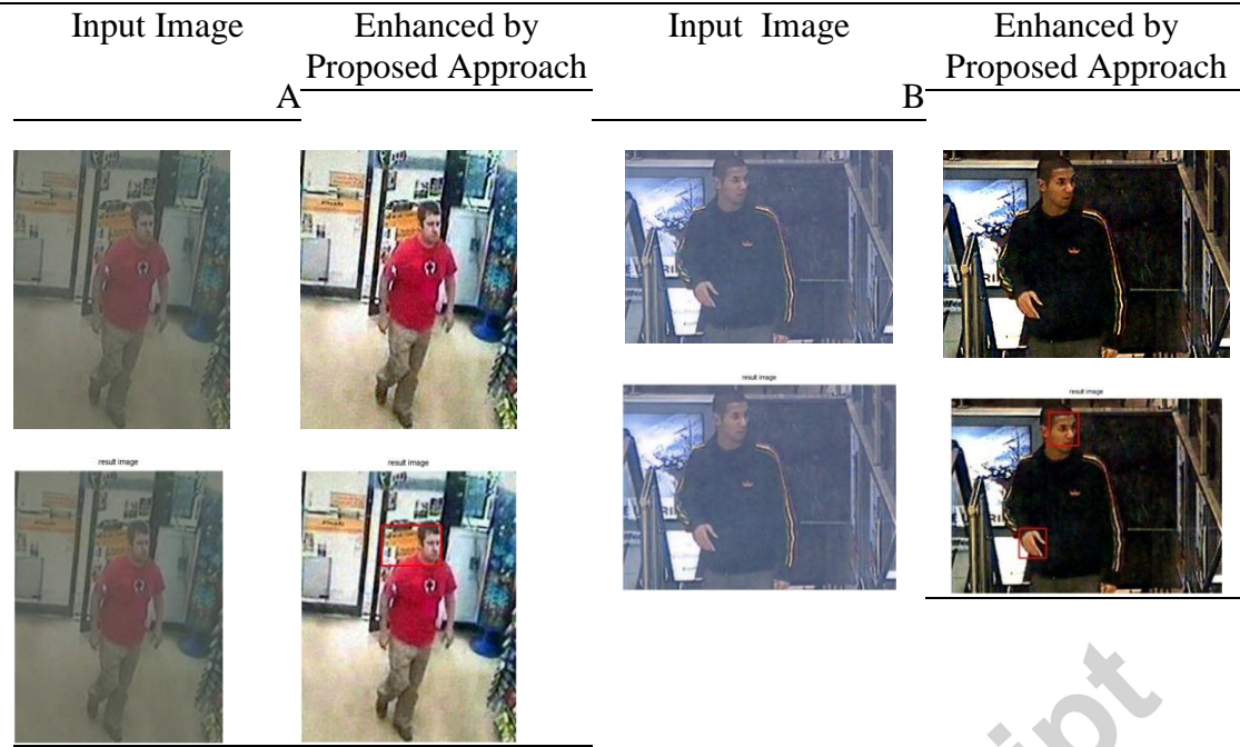
Figure 2: Skin colour based face detection method before and after using the proposed integrated image enhancement approach (A-person is entering into a shop) and (B-person is on an accelerator)
