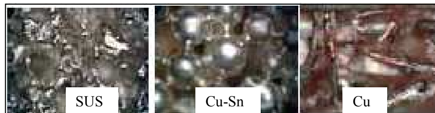
Fig.3. Microphotography of particle-sintered porous metal and fiber-sintered porous metal
