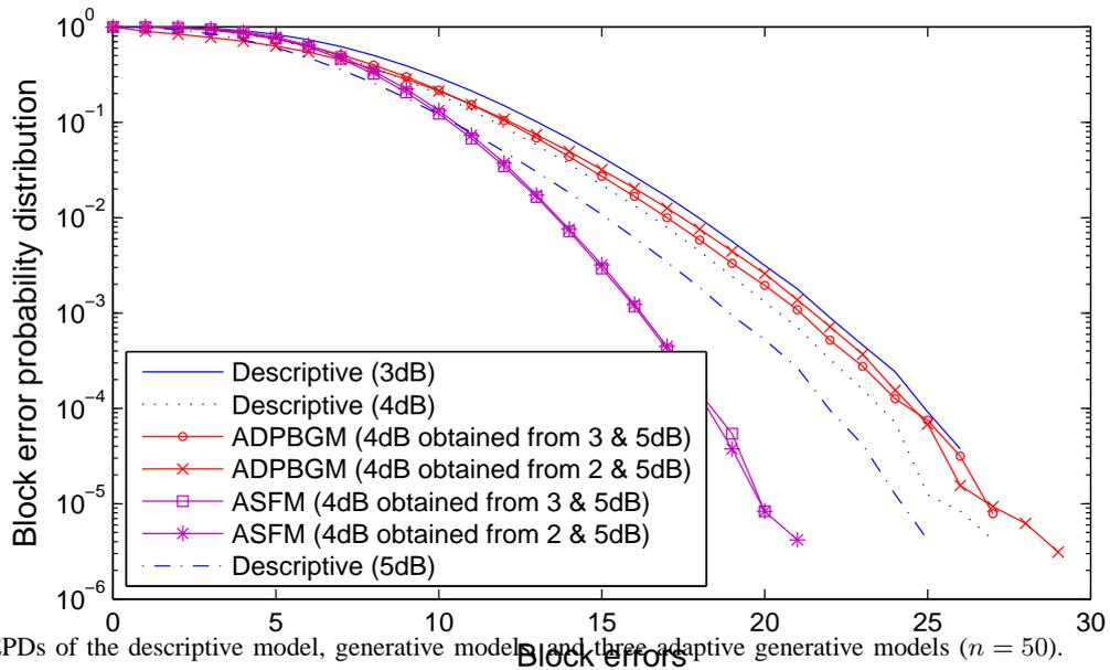
Fig. 8. The BEPDs of the descriptive model, generative models, and three adaptive generative models ( $n = 50$ ).
