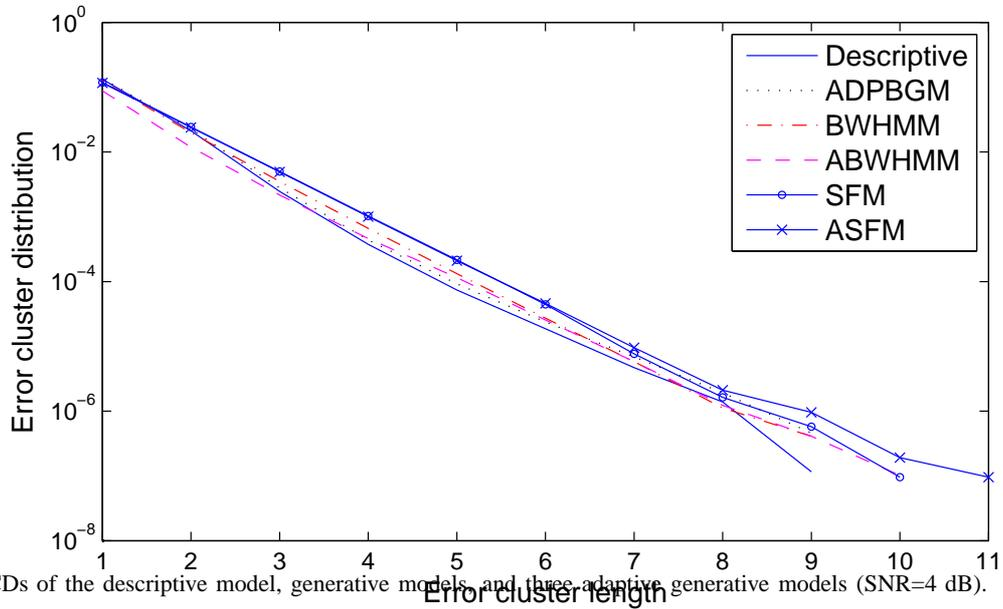
Fig. 3. The ECDs of the descriptive model, generative models, and three adaptive generative models (SNR=4 dB).
