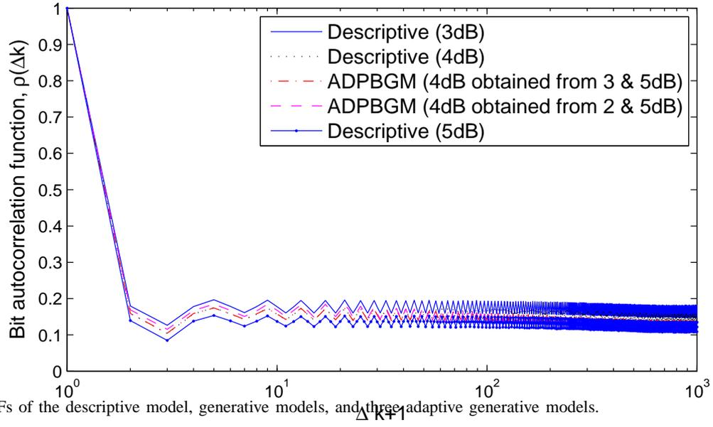
Fig. 9. The BCFs of the descriptive model, generative models, and three adaptive generative models.
