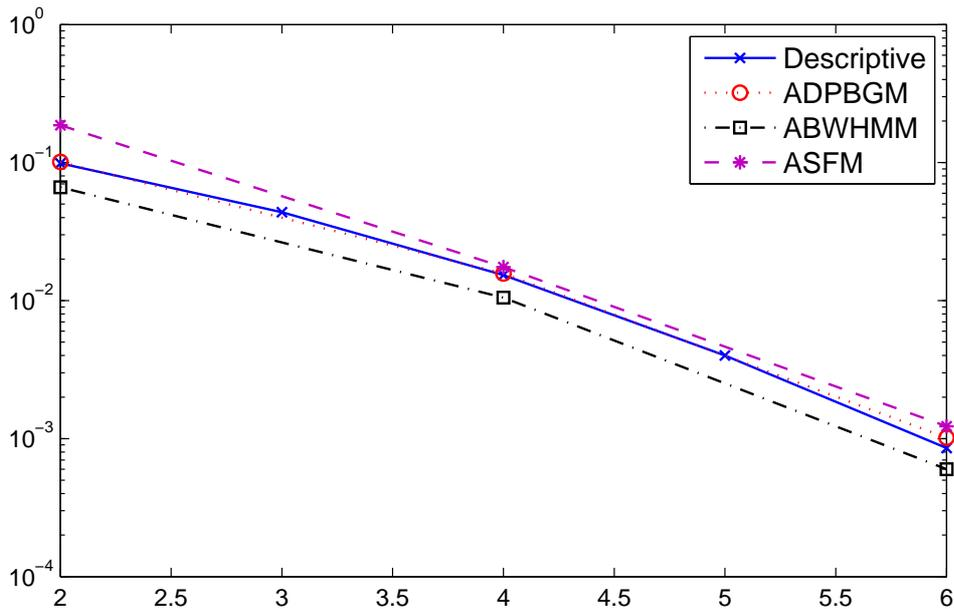
Fig. 12. The coded BER of the descriptive model and three adaptive generative models.
