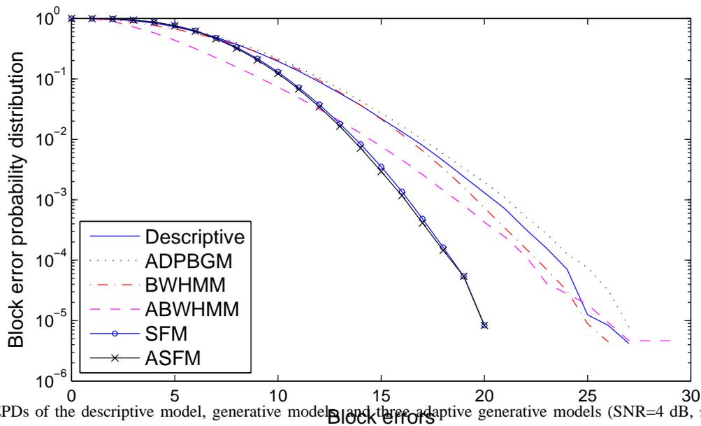
Fig. 4. The BEPDs of the descriptive model, generative models, and three adaptive generative models (SNR=4 dB,  $n = 50$ ).
