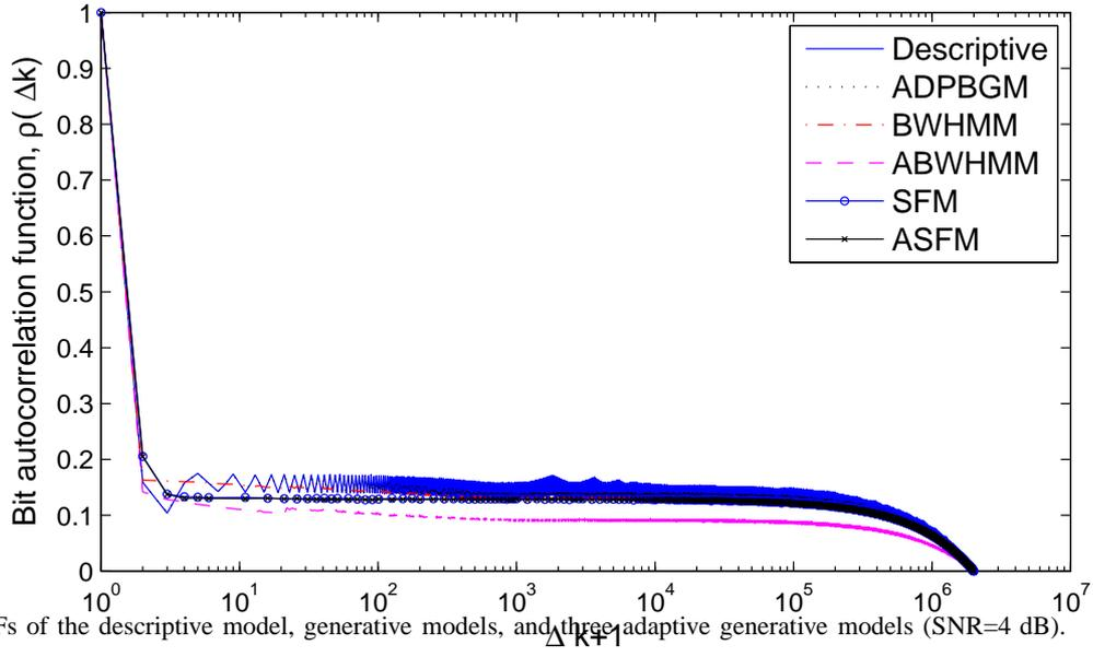
Fig. 5. The BCFs of the descriptive model, generative models, and three adaptive generative models (SNR=4 dB).
