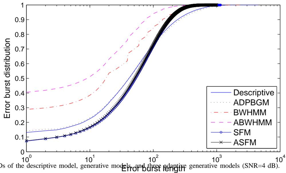
Fig. 6. The EBDs of the descriptive model, generative models, and three adaptive generative models (SNR=4 dB).
