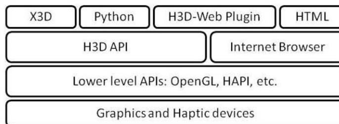
Figure 1. Architecture of a browser-based VE with haptics
