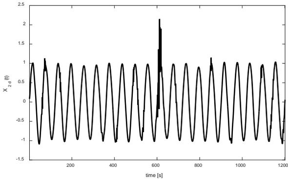
In Fig. 8 the error  $e(t)$  is illustrated;  $e(t)$  is defined by,  $e(t) = X_{2d}(t) - X_{2nn}(t)$ , where  $X_{2nn}(t)$  is the output of the autoregressive neural network. It is evident that an anomalous behavior has taken place in the period  $t \in [600, 620]$  because of the different pattern observed in the envelope's amplitude as shown in Fig 9.
