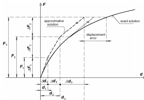
**Figure 2.2:** Incremental loading pattern of the model(Ivančo 2011)
