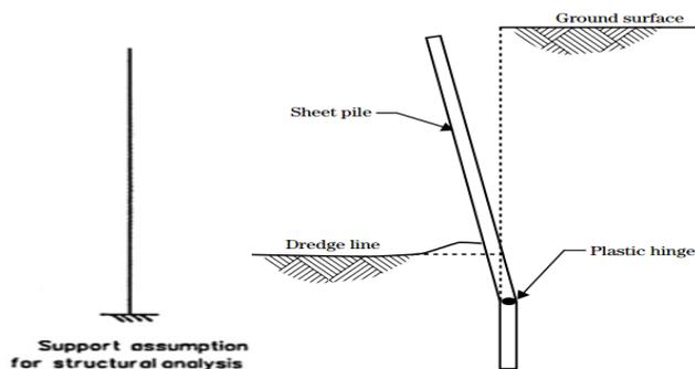
Figure 3.1: Assumed Support and failure for cantilevered sheet pile wall (Technical Supplement 14R 2007)
