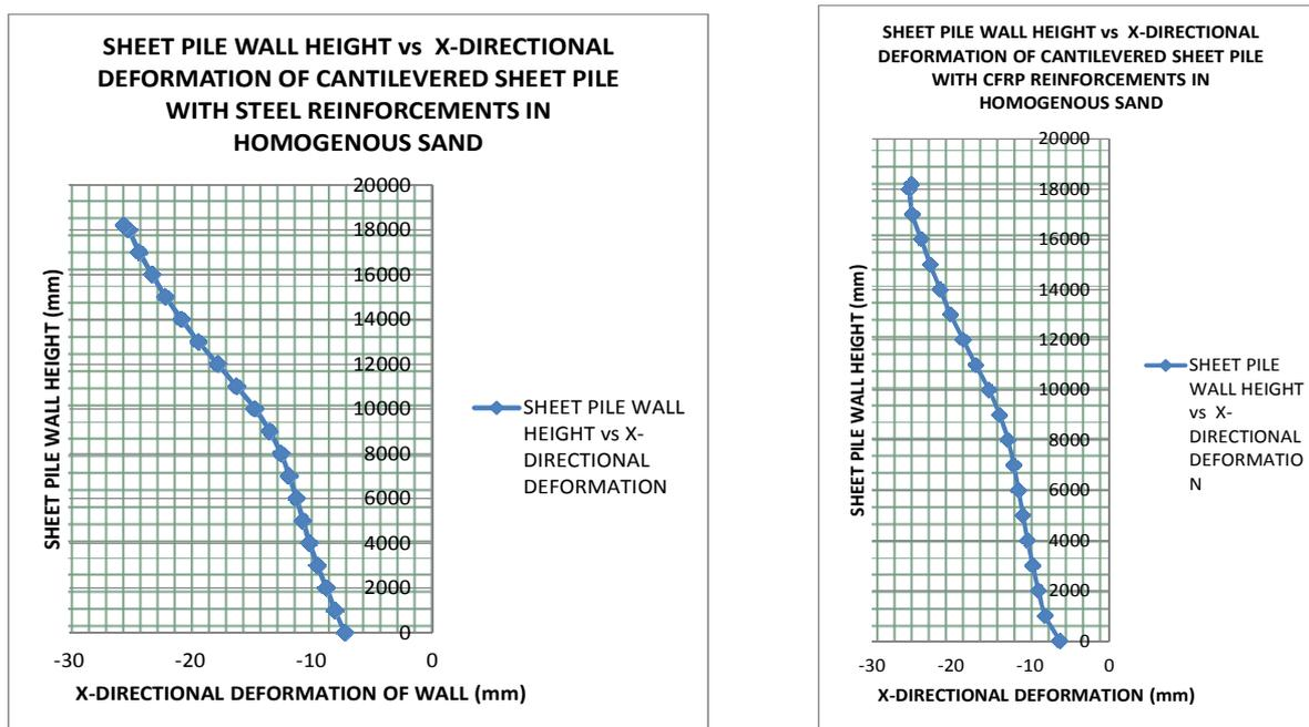
Figure 3.2: Horizontal deformation of wall with Steel & CFRP
