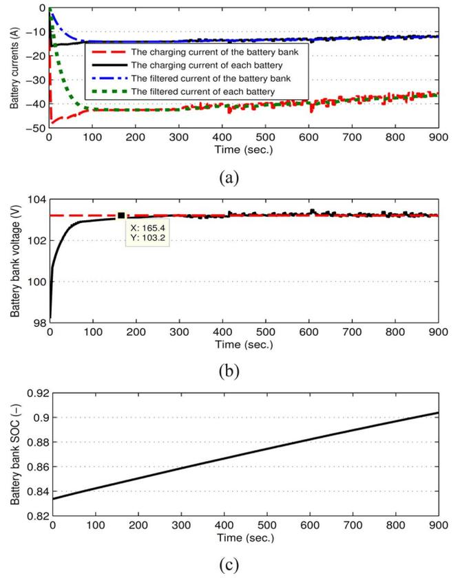
Fig. 7. (a) Charging current; (b) terminal voltage; and (c) SOC of the battery bank in Scenario II.
