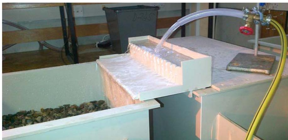
**Figure 2 - Spillway in operation**
