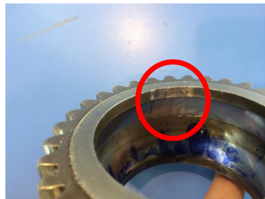
Figure 2 Slot across the bearing outer race
