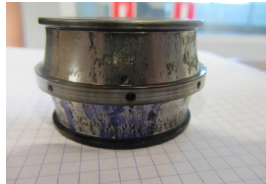
Figure 3 Inner race natural spalling
