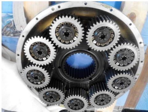
Figure 1 Second stage epicyclic gears
