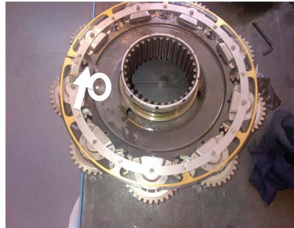
Figure 4 Moving coil mounted on the planetary carrier (coil arrowed, sensor circled)
