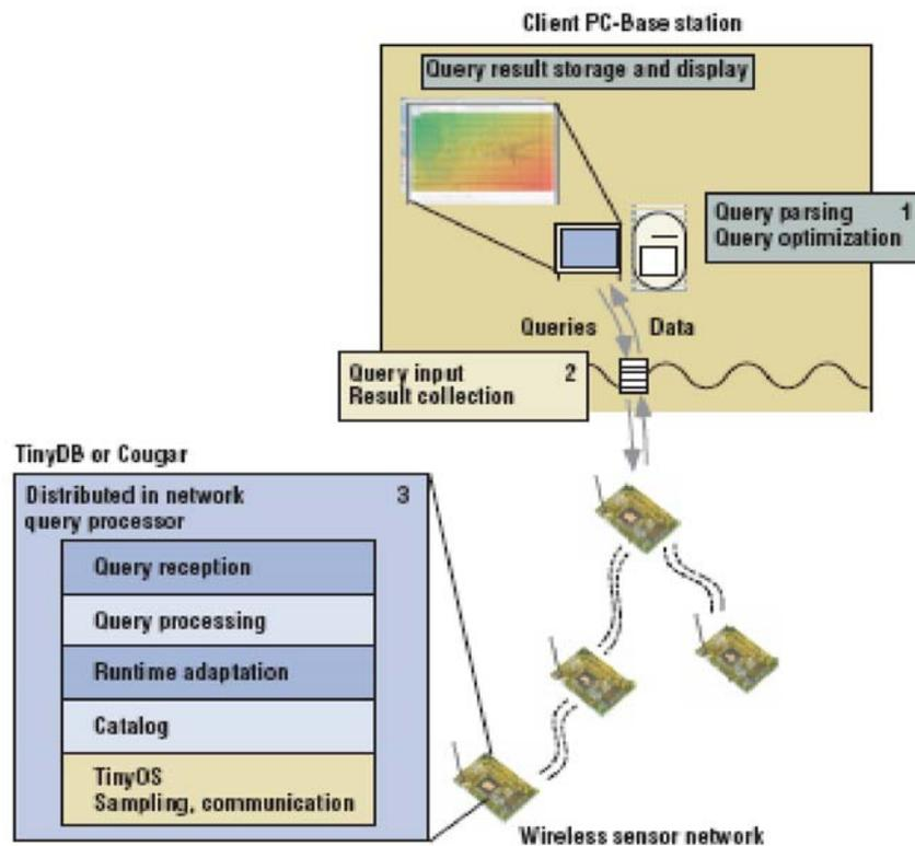
**Fig. 5.** A detailed view of the query processing architecture of TinyDB and Cougar taken from [35].
