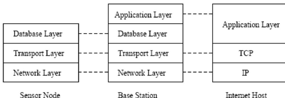
**Fig. 3.** A database-based query processing architecture taken from [34].
