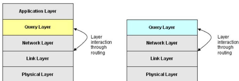
**Fig. 4.** A high level view of the query processing architecture used in Cougar and TinyDB.
