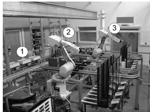
Fig. 5. Layout of the manufacturing cell; showing shuttles (1), robot 2 (2) and robot 1 (3)
