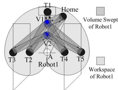
Fig. 6. Swept volume and trajectory of robot 1
