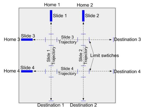
Fig. 3. Layout of the manufacturing cell for the two slide problem
