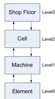
Fig. 1 Manufacturing system functional hierarchy (Phelan et al., 2003)
