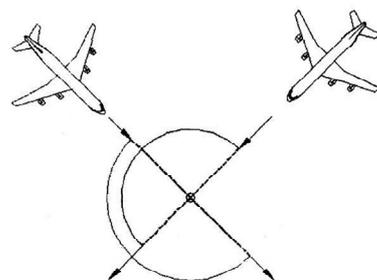
Fig. 2 The *roundabout* policy for air traffic collision avoidance (Massink et al., 2001)
